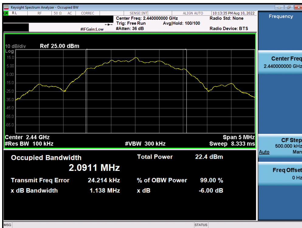
Plot 7-5. 6dB BW & 99% OBW Plot (Bluetooth (LE), 2Mbps – Ch. 19)
