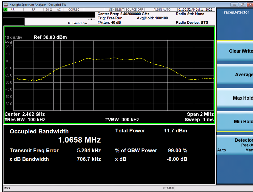
Plot 7-1. 6dB BW & 99% OBW Plot (Bluetooth (LE), 1Mbps – Ch. 0)
