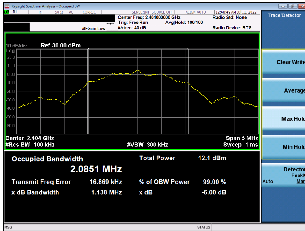
Plot 7-4. 6dB BW & 99% OBW Plot (Bluetooth (LE), 2Mbps – Ch. 1)
