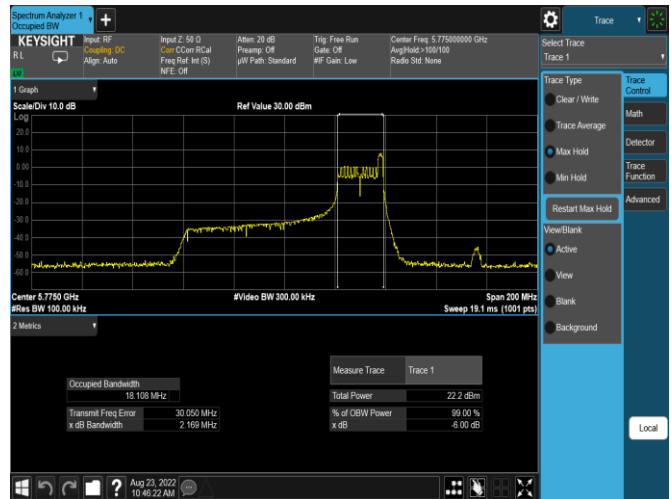
Plot 7-95. 6dB BW & 99% OBW Antenna WF7a (80MHz BW 11ax Index 36 – RU26 – Ch.155)
