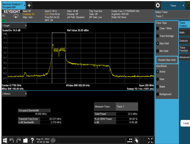
Plot 7-93. 6dB BW & 99% OBW Antenna WF7a (80MHz BW 11ax Index 0 – RU26 – Ch.155)
