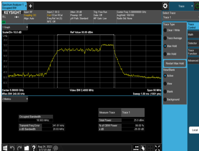
Plot 7-63. 26dB BW & 99% OBW Antenna WF7a (20MHz BW 11ax Index 44 – RU52 – Ch.116)
