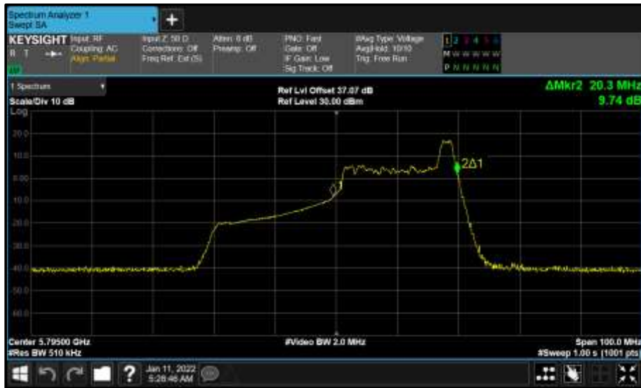
Figure 788 - Core 0 (A) 5795 MHz (CH159) 99% Bandwidth
