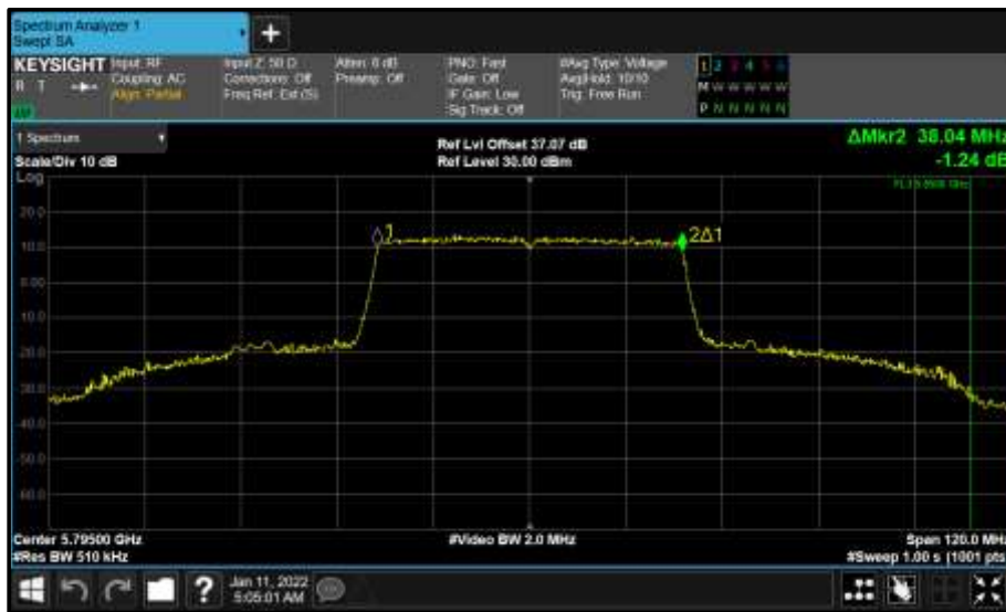
Figure 760 - Core 0 (A) 5795 MHz (CH159) 99% Bandwidth
