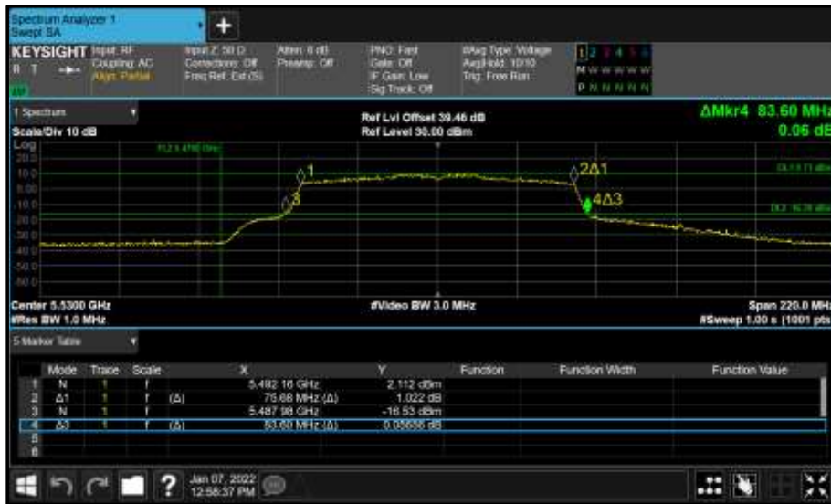
Figure 938 - Core 0 (A) 5530 MHz (CH106) 26 dB and 99% Bandwidth
