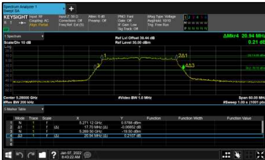
Figure 913 - Core 1 (B) 5280 MHz (CH56) 26 dB and 99% Bandwidth
