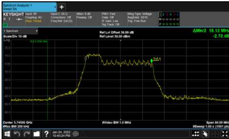
Figure 746 - Core 1 (B) 5745 MHz (CH149) 99% Bandwidth
