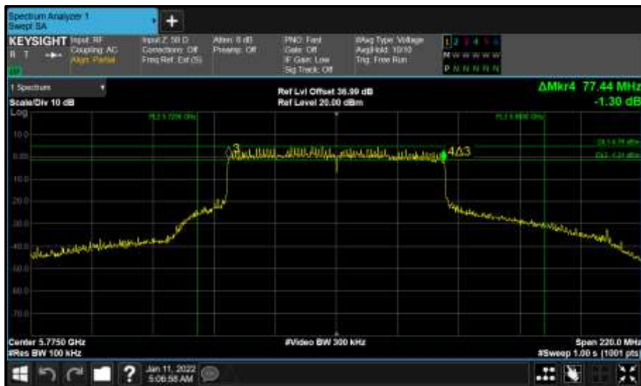
Figure 839 - Core 0 (A) 5775 MHz (CH155) 6 dB Bandwidth
