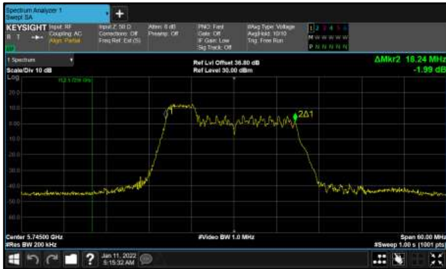
Figure 718 - Core 0 (A) 5745 MHz (CH149) 99% Bandwidth
