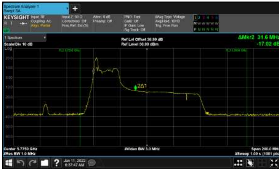
Figure 858 - Core 0 (A) 5775 MHz (CH155) 99% Bandwidth
