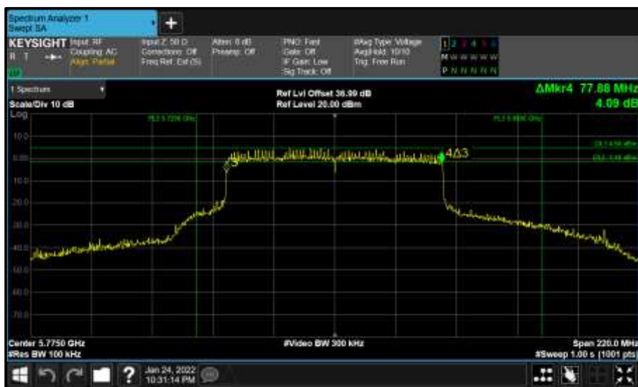
Figure 853 - Core 0 (A) 5775 MHz (CH155) 6 dB Bandwidth
