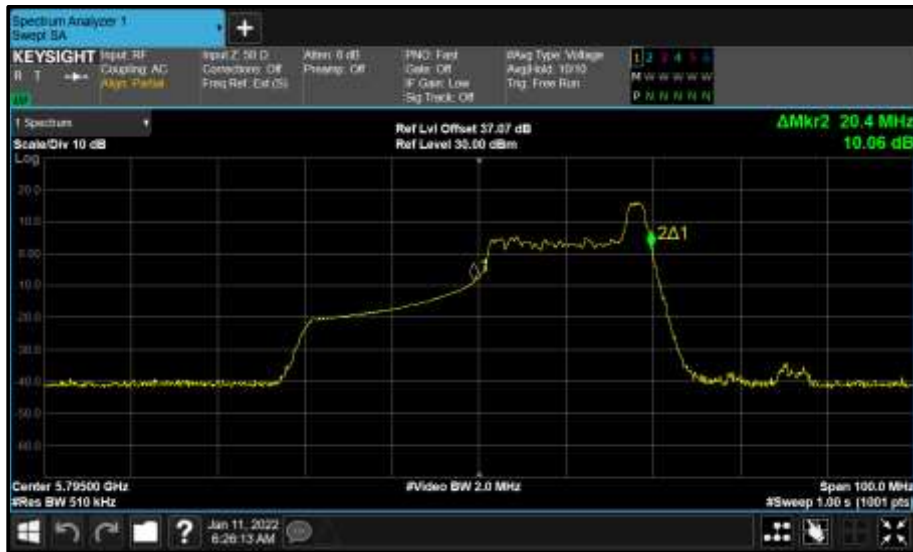
Figure 794 - Core 0 (A) 5795 MHz (CH159) 99% Bandwidth
