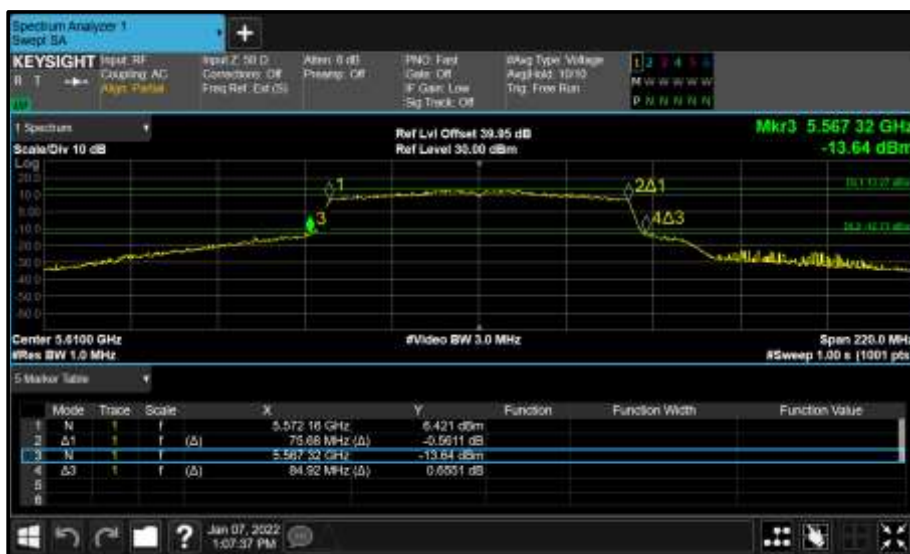
Figure 941 - Core 1 (B) 5610 MHz (CH122) 26 dB and 99% Bandwidth
