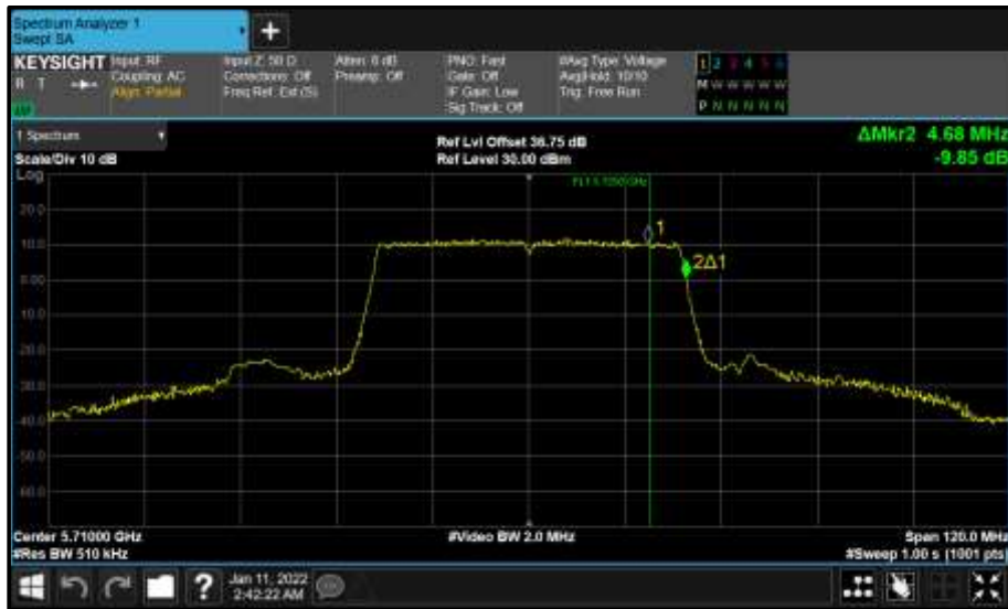
Figure 762 - Core 0 (A) 5710 MHz (CH142) 99% Bandwidth
