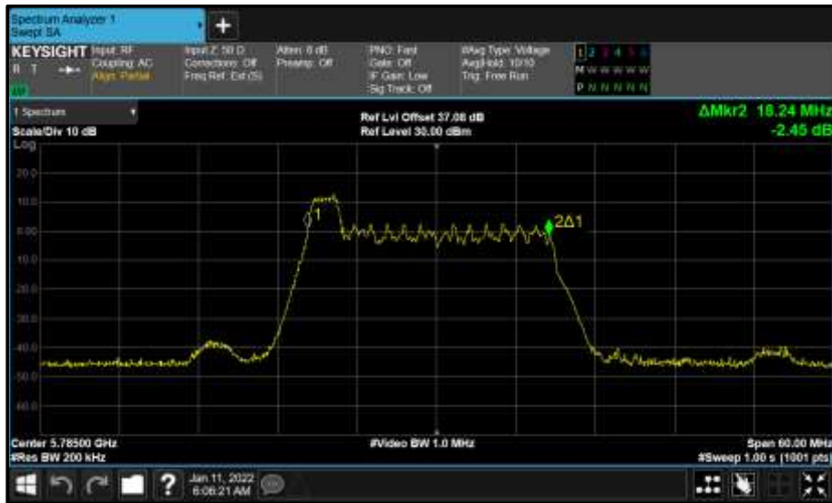
Figure 698 - Core 1 (B) 5785 MHz (CH157) 99% Bandwidth
