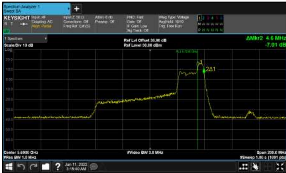
Figure 872 - Core 1 (B) 5690 MHz (CH138) 99% Bandwidth
