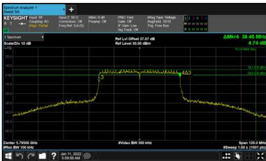
Figure 771 - Core 0 (A) 5795 MHz (CH159) 6 dB Bandwidth
