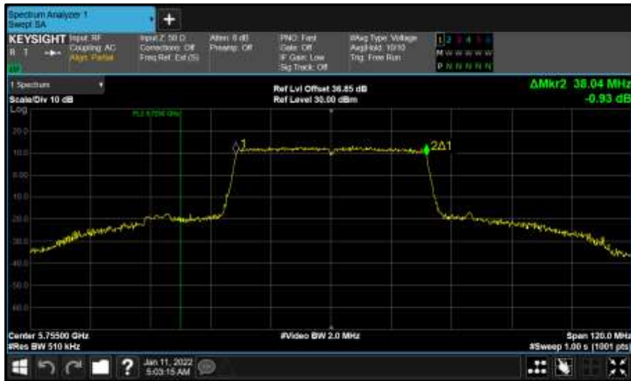
Figure 758 - Core 0 (A) 5755 MHz (CH151) 99% Bandwidth
