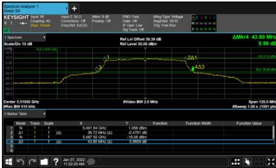
Figure 930 - Core 0 (A) 5510 MHz (CH102) 26 dB and 99% Bandwidth
