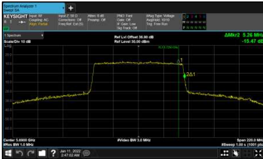
Figure 842 - Core 1 (B) 5690 MHz (CH138) 99% Bandwidth
