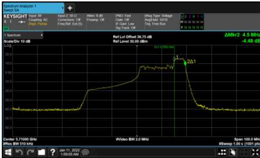
Figure 806 - Core 0 (A) 5710 MHz (CH142) 99% Bandwidth
