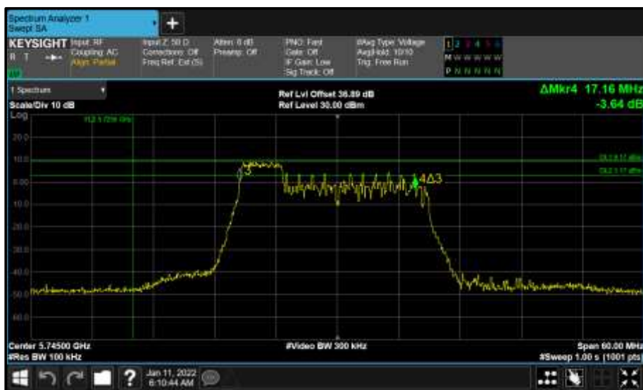
Figure 731 - Core 1 (B) 5745 MHz (CH149) 6 dB Bandwidth
