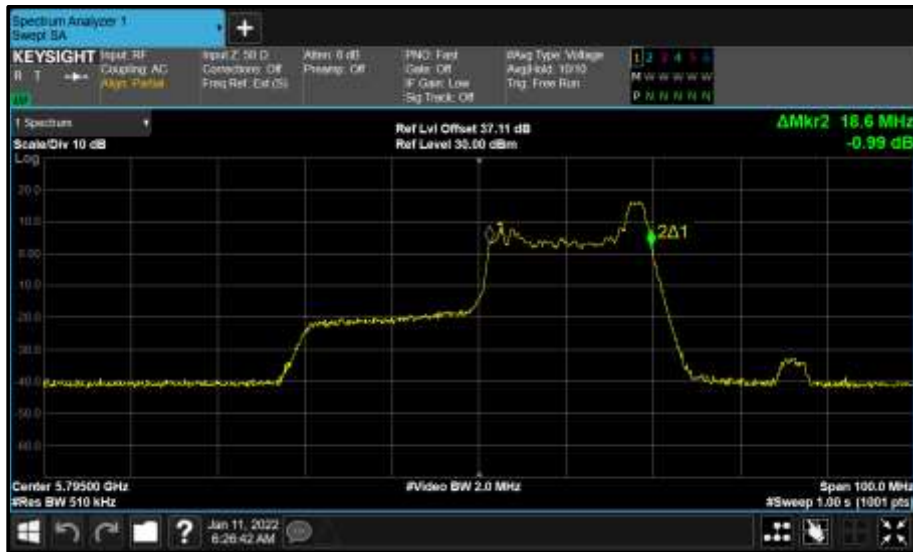
Figure 796 - Core 1 (B) 5795 MHz (CH159) 99% Bandwidth
