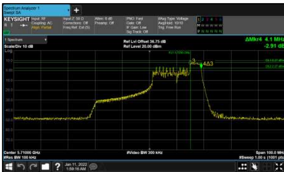
Figure 807 - Core 0 (A) 5710 MHz (CH142) 6 dB Bandwidth
