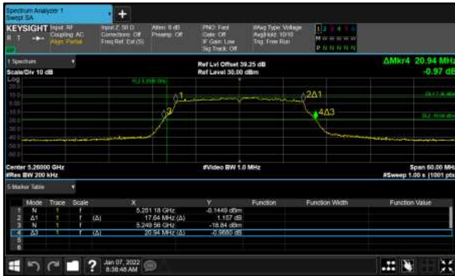
Figure 910 - Core 0 (A) 5260 MHz (CH52) 26 dB and 99% Bandwidth
