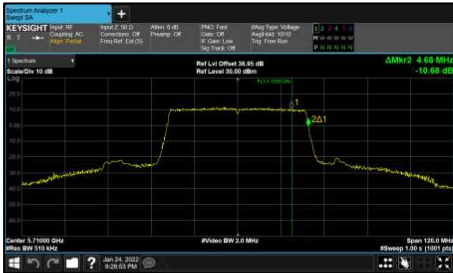
Figure 776 - Core 1 (B) 5710 MHz (CH142) 99% Bandwidth
