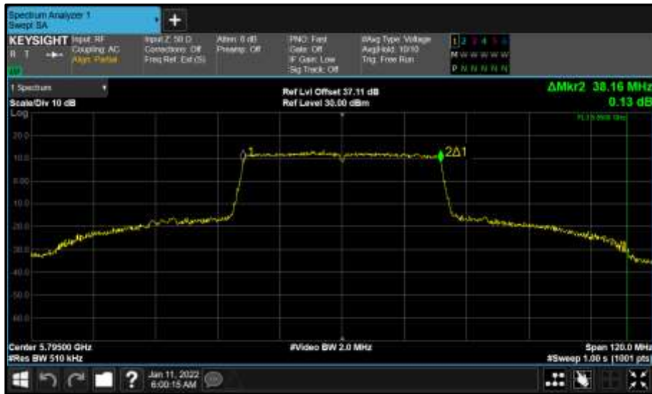
Figure 772 - Core 1 (B) 5795 MHz (CH159) 99% Bandwidth
