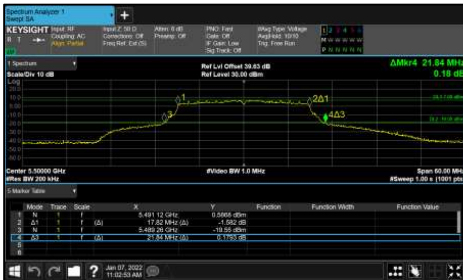
Figure 923 - Core 1 (B) 5500 MHz (CH100) 26 dB and 99% Bandwidth
