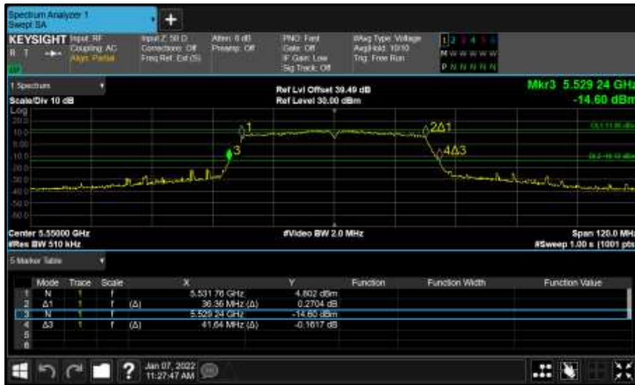
Figure 932 - Core 0 (A) 5550 MHz (CH110) 26 dB and 99% Bandwidth
