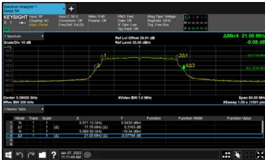
Figure 925 - Core 1 (B) 5580 MHz (CH116) 26 dB and 99% Bandwidth
