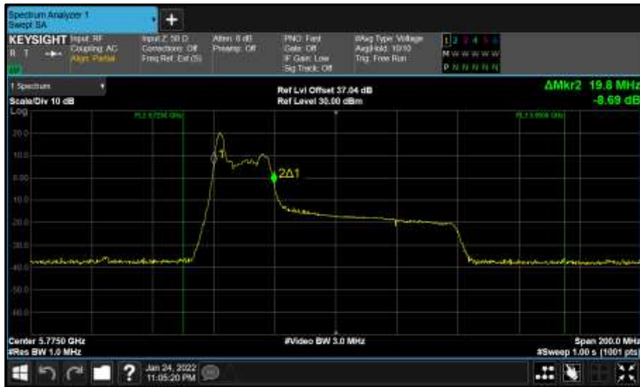
Figure 864 - Core 1 (B) 5775 MHz (CH155) 99% Bandwidth
