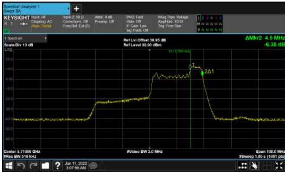
Figure 814 - Core 1 (B) 5710 MHz (CH142) 99% Bandwidth
