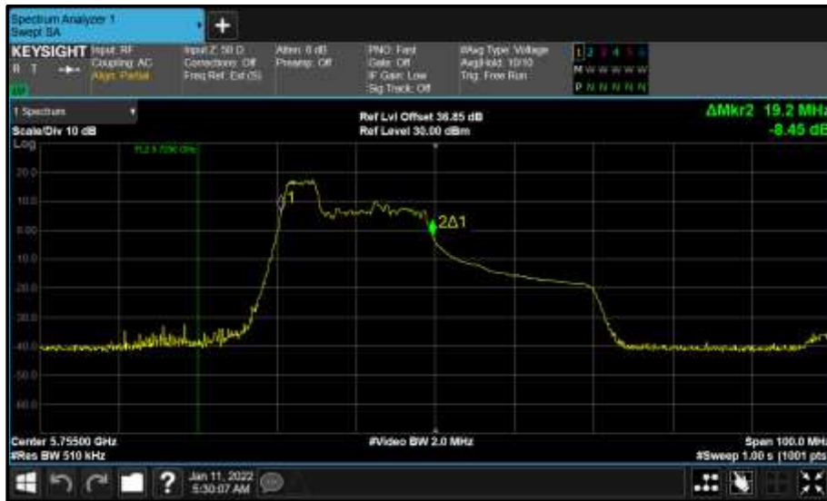
Figure 808 - Core 0 (A) 5755 MHz (CH151) 99% Bandwidth
