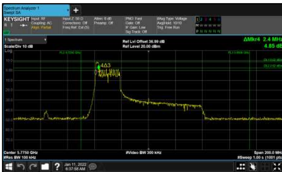
Figure 859 - Core 0 (A) 5775 MHz (CH155) 6 dB Bandwidth
