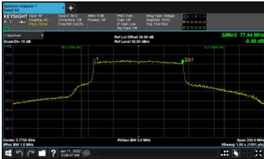
Figure 838 - Core 0 (A) 5775 MHz (CH155) 99% Bandwidth
