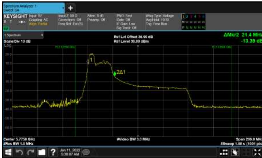
Figure 868 - Core 0 (A) 5775 MHz (CH155) 99% Bandwidth
