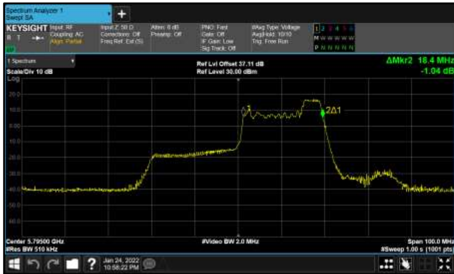
Figure 834 - Core 1 (B) 5795 MHz (CH159) 99% Bandwidth
