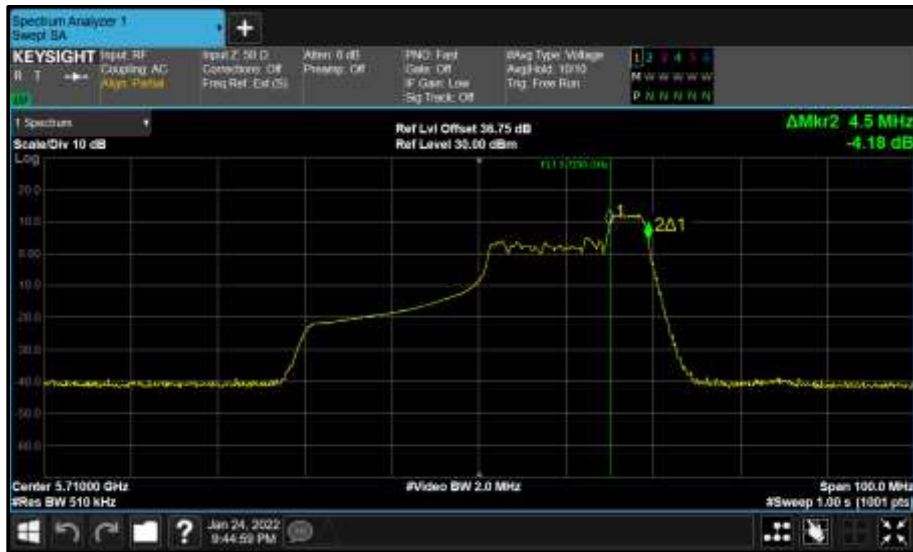
Figure 824 - Core 0 (A) 5710 MHz (CH142) 99% Bandwidth
