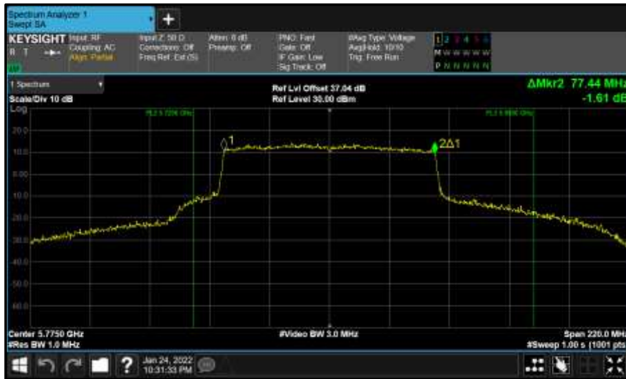
Figure 854 - Core 1 (B) 5775 MHz (CH155) 99% Bandwidth
