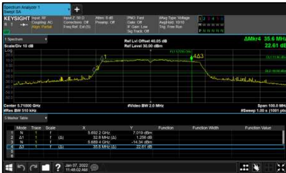
Figure 937 - Core 1 (B) 5710 MHz (CH142) 26 dB and 99% Bandwidth
