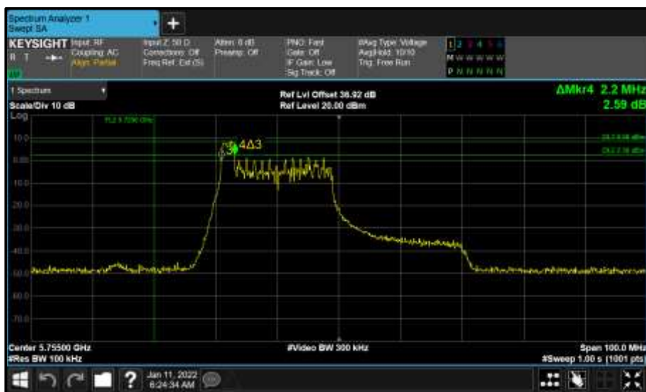
Figure 793 - Core 1 (B) 5755 MHz (CH151) 6 dB Bandwidth
