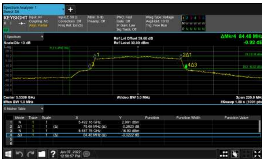
Figure 939 - Core 1 (B) 5530 MHz (CH106) 26 dB and 99% Bandwidth
