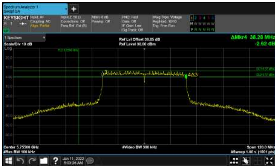
Figure 759 - Core 0 (A) 5755 MHz (CH151) 6 dB Bandwidth
