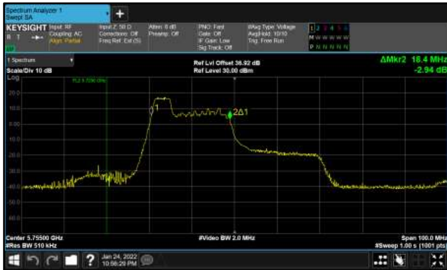
Figure 830 - Core 1 (B) 5755 MHz (CH151) 99% Bandwidth
