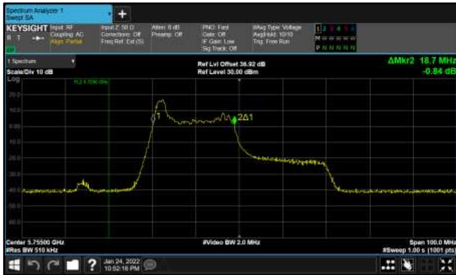
Figure 800 - Core 1 (B) 5755 MHz (CH151) 99% Bandwidth
