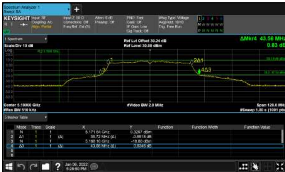
Figure 903 - Core 1 (B) 5190 MHz (CH38) 26 dB and 99% Bandwidth
