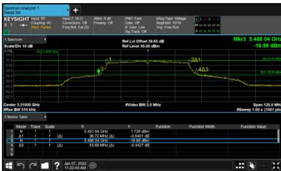
Figure 931 - Core 1 (B) 5510 MHz (CH102) 26 dB and 99% Bandwidth
