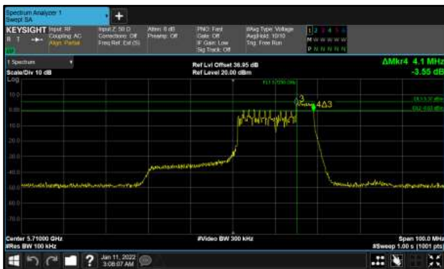
Figure 815 - Core 1 (B) 5710 MHz (CH142) 6 dB Bandwidth
