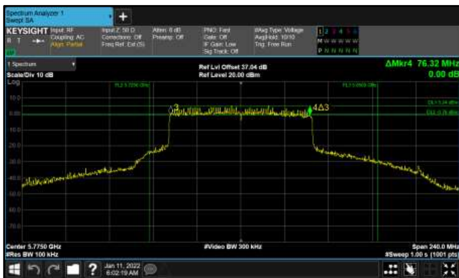
Figure 847 - Core 1 (B) 5775 MHz (CH155) 6 dB Bandwidth
