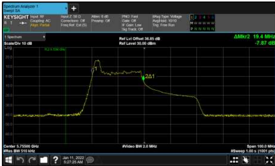
Figure 786 - Core 0 (A) 5755 MHz (CH151) 99% Bandwidth
