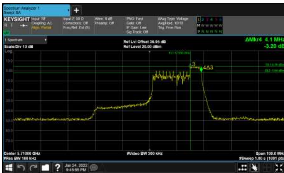
Figure 827 - Core 1 (B) 5710 MHz (CH142) 6 dB Bandwidth
