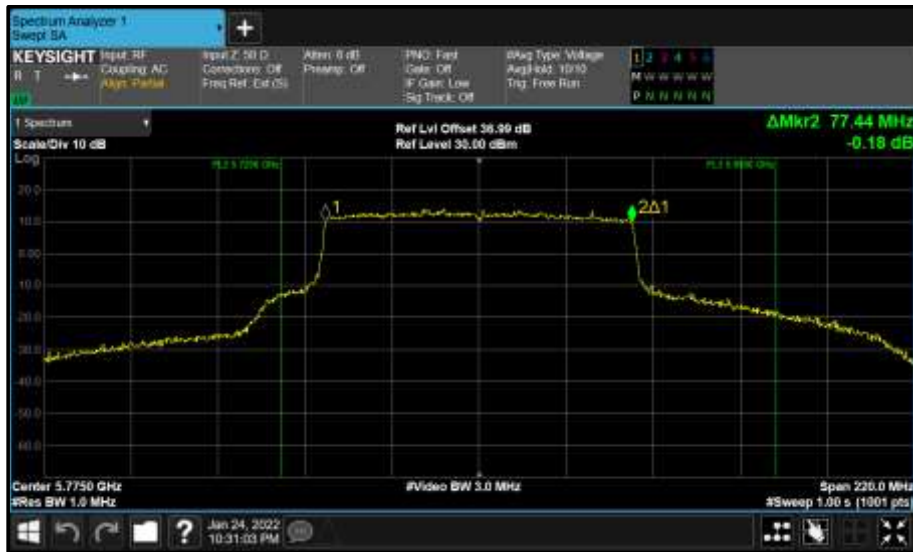
Figure 852 - Core 0 (A) 5775 MHz (CH155) 99% Bandwidth
