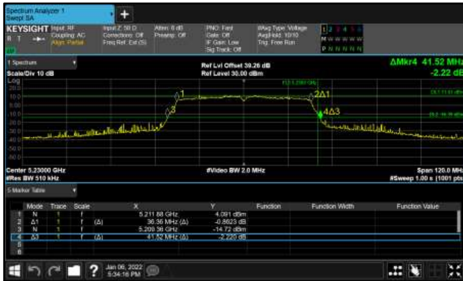
Figure 904 - Core 0 (A) 5230 MHz (CH46) 26 dB and 99% Bandwidth
