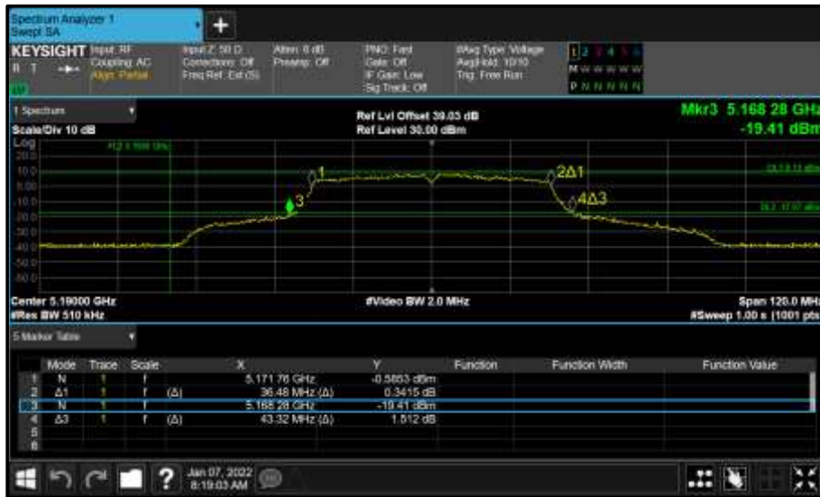
Figure 898 - Core 0 (A) 5190 MHz (CH38) 26 dB and 99% Bandwidth
