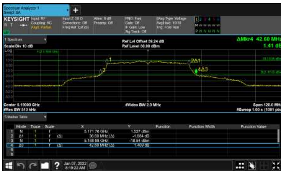
Figure 899 - Core 1 (B) 5190 MHz (CH38) 26 dB and 99% Bandwidth
