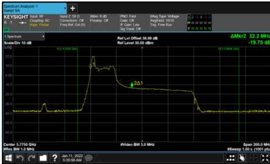
Figure 856 - Core 0 (A) 5775 MHz (CH155) 99% Bandwidth
