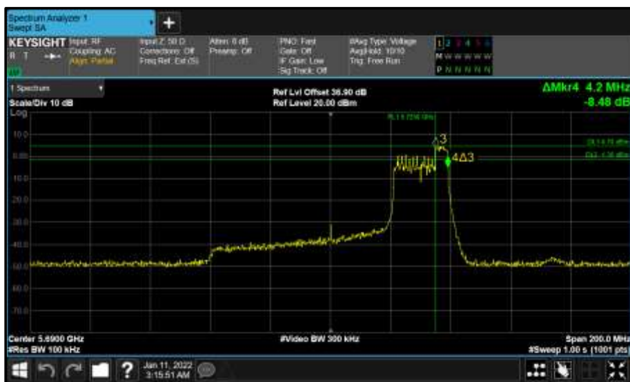
Figure 873 - Core 1 (B) 5690 MHz (CH138) 6 dB Bandwidth
