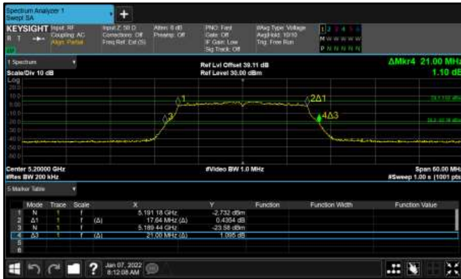
Figure 888 - Core 0 (A) 5200 MHz (CH40) 26 dB and 99% Bandwidth
