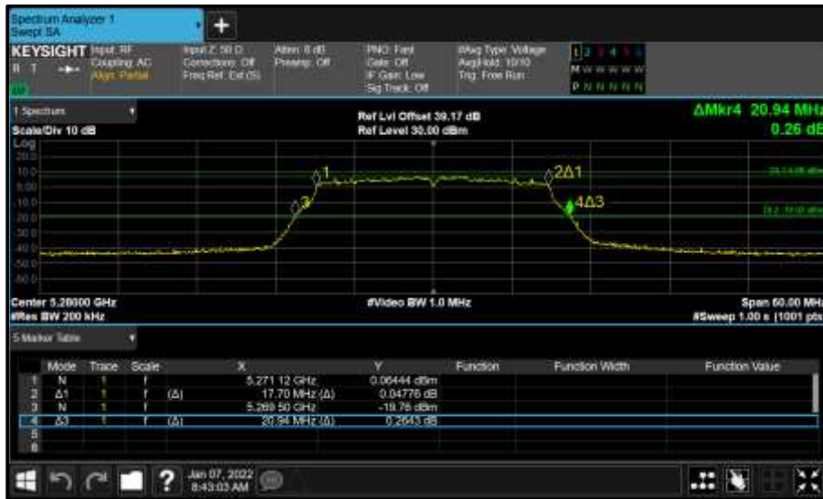
Figure 912 - Core 0 (A) 5280 MHz (CH56) 26 dB and 99% Bandwidth
