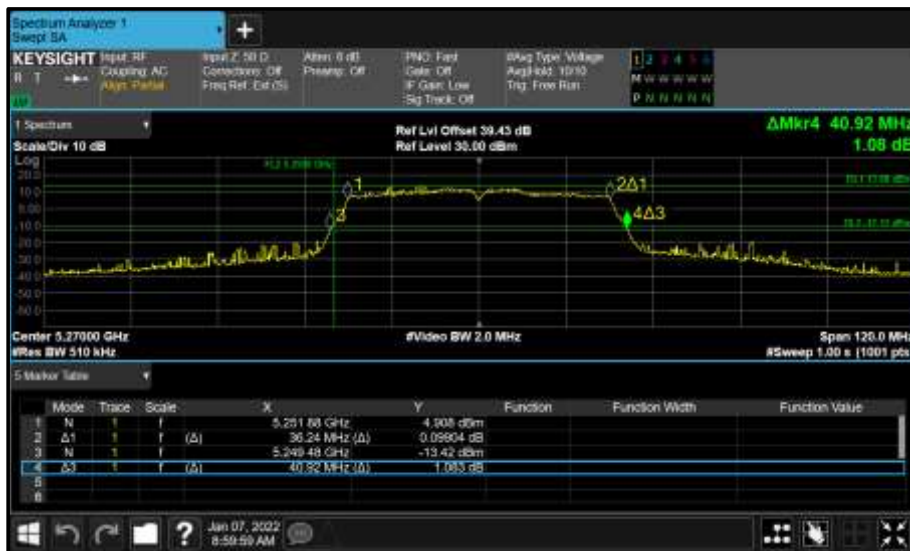
Figure 917 - Core 1 (B) 5270 MHz (CH54) 26 dB and 99% Bandwidth
