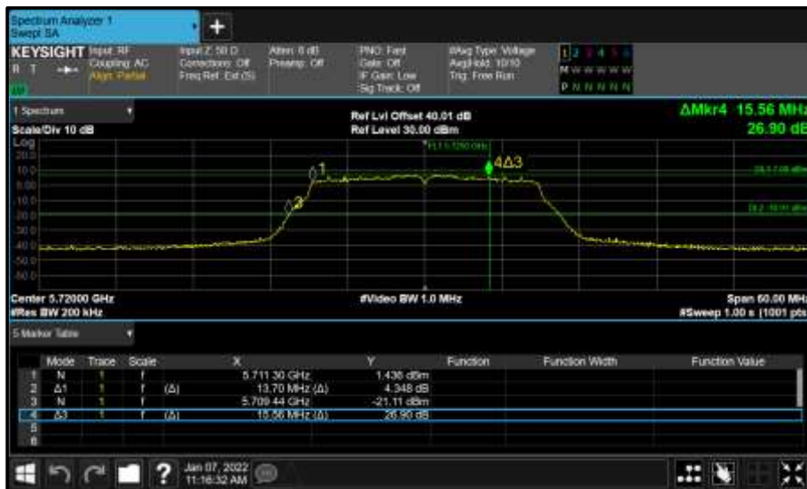
Figure 929 - Core 1 (B) 5720 MHz (CH144) 26 dB and 99% Bandwidth
