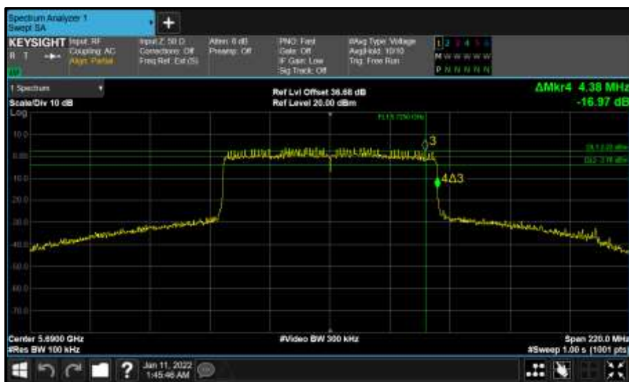
Figure 837 - Core 0 (A) 5690 MHz (CH138) 6 dB Bandwidth
