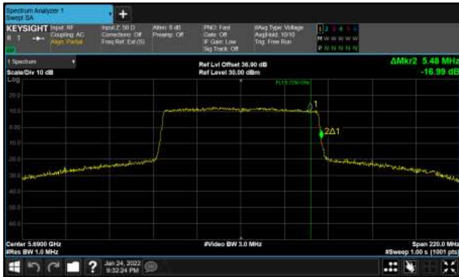
Figure 850 - Core 1 (B) 5690 MHz (CH138) 99% Bandwidth
