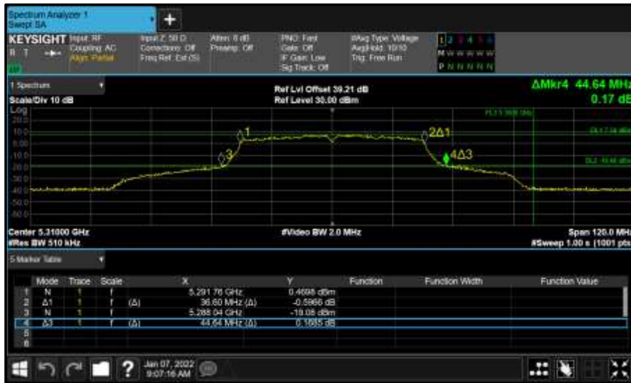
Figure 918 - Core 0 (A) 5310 MHz (CH62) 26 dB and 99% Bandwidth
