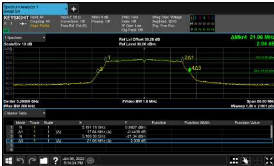
Figure 895 - Core 1 (B) 5200 MHz (CH40) 26 dB and 99% Bandwidth
