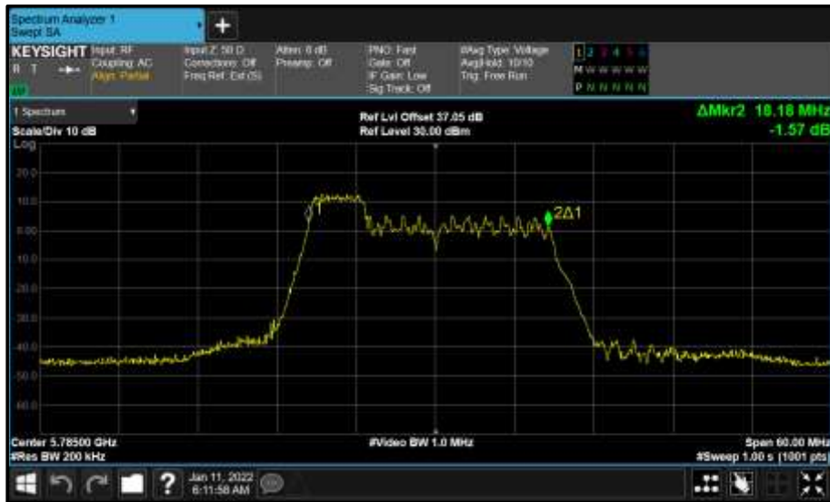
Figure 732 - Core 0 (A) 5785 MHz (CH157) 99% Bandwidth
