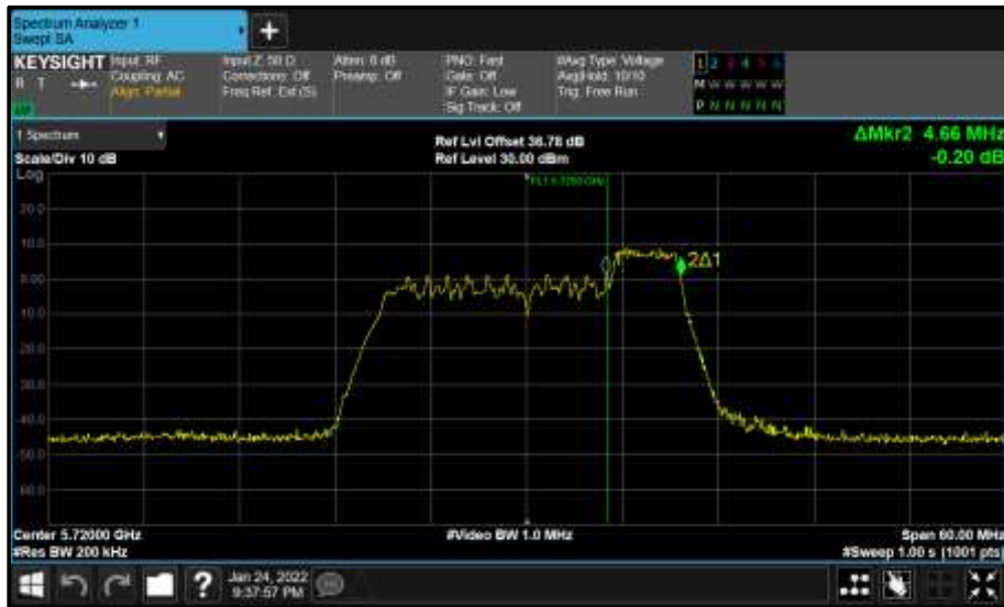
Figure 740 - Core 0 (A) 5720 MHz (CH144) 99% Bandwidth
