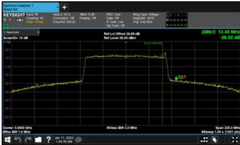
Figure 836 - Core 0 (A) 5690 MHz (CH138) 99% Bandwidth
