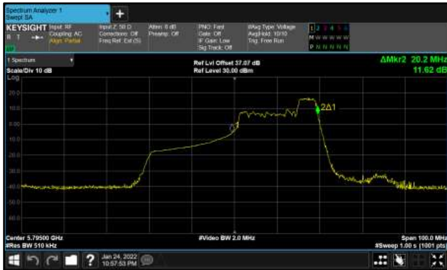
Figure 832 - Core 0 (A) 5795 MHz (CH159) 99% Bandwidth
