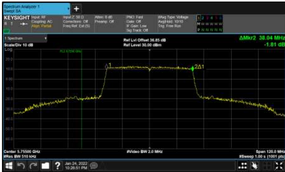
Figure 778 - Core 0 (A) 5755 MHz (CH151) 99% Bandwidth
