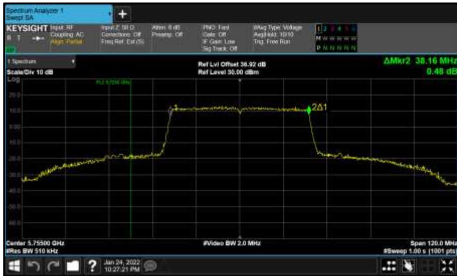
Figure 780 - Core 1 (B) 5755 MHz (CH151) 99% Bandwidth
