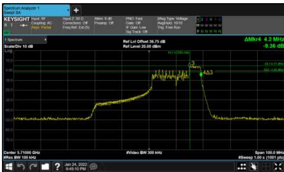
Figure 825 - Core 0 (A) 5710 MHz (CH142) 6 dB Bandwidth
