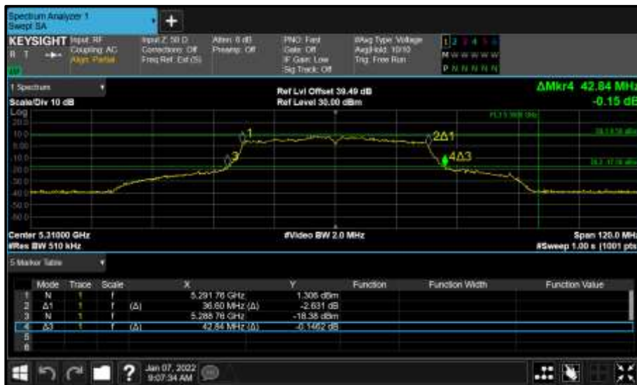
Figure 919 - Core 1 (B) 5310 MHz (CH62) 26 dB and 99% Bandwidth
