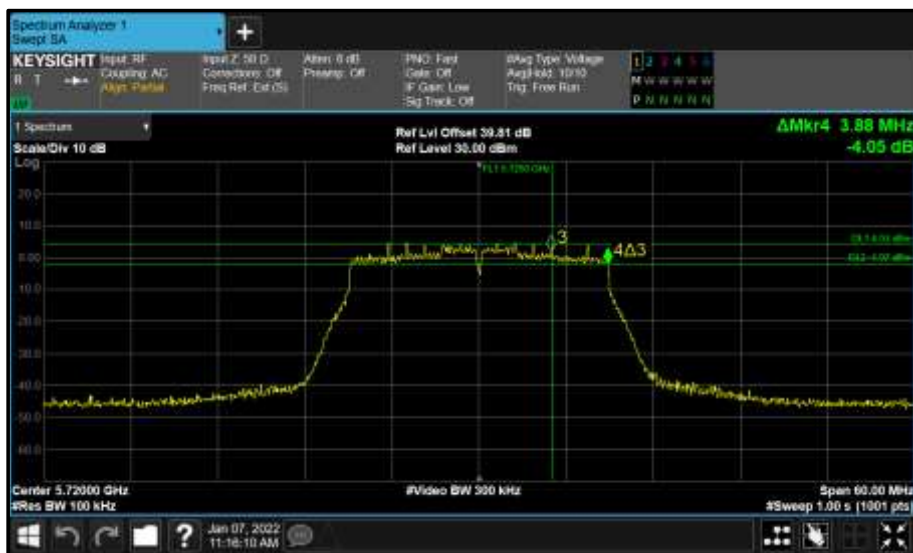
Figure 945 - Core 0 (A) 5720 MHz (CH144) 6 dB Bandwidth
