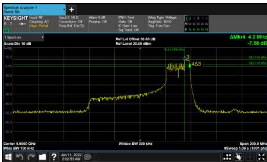
Figure 867 - Core 0 (A) 5690 MHz (CH138) 6 dB Bandwidth
