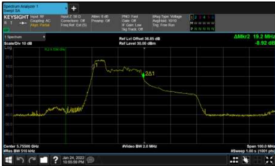
Figure 828 - Core 0 (A) 5755 MHz (CH151) 99% Bandwidth
