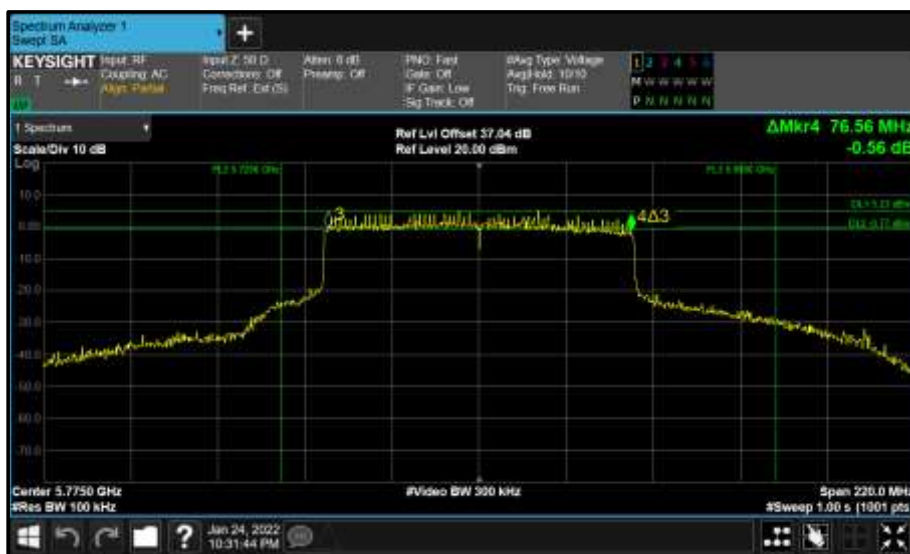
Figure 855 - Core 1 (B) 5775 MHz (CH155) 6 dB Bandwidth
