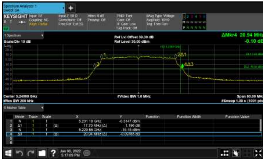
Figure 896 - Core 0 (A) 5240 MHz (CH48) 26 dB and 99% Bandwidth
