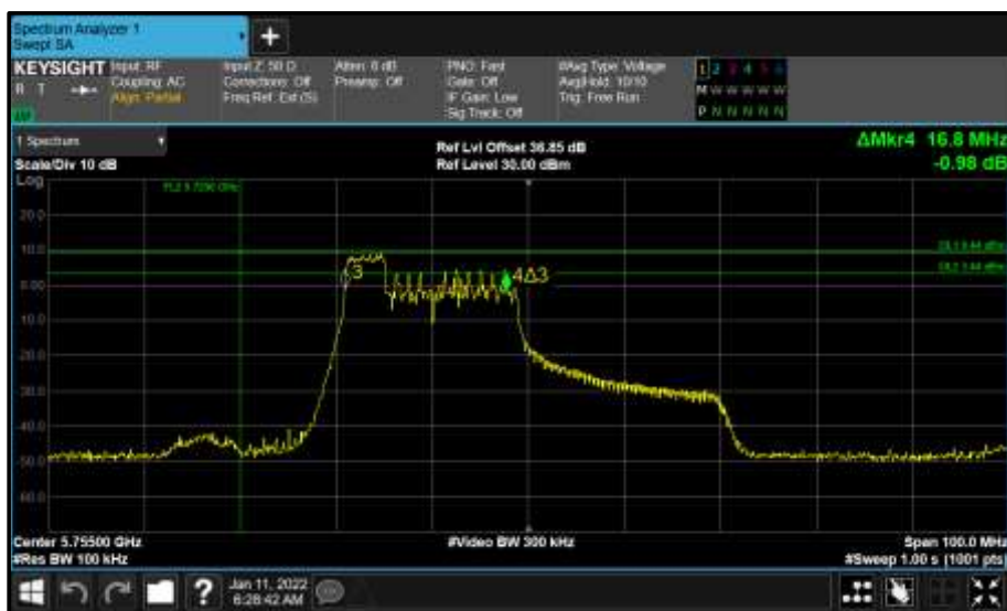
Figure 817 - Core 0 (A) 5755 MHz (CH151) 6 dB Bandwidth
