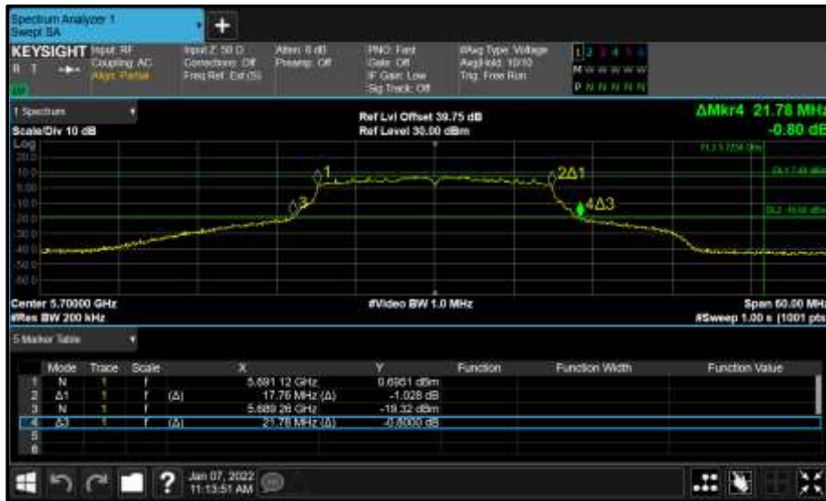
Figure 926 - Core 0 (A) 5700 MHz (CH140) 26 dB and 99% Bandwidth
