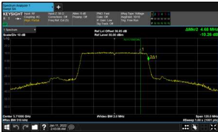
Figure 764 - Core 1 (B) 5710 MHz (CH142) 99% Bandwidth
