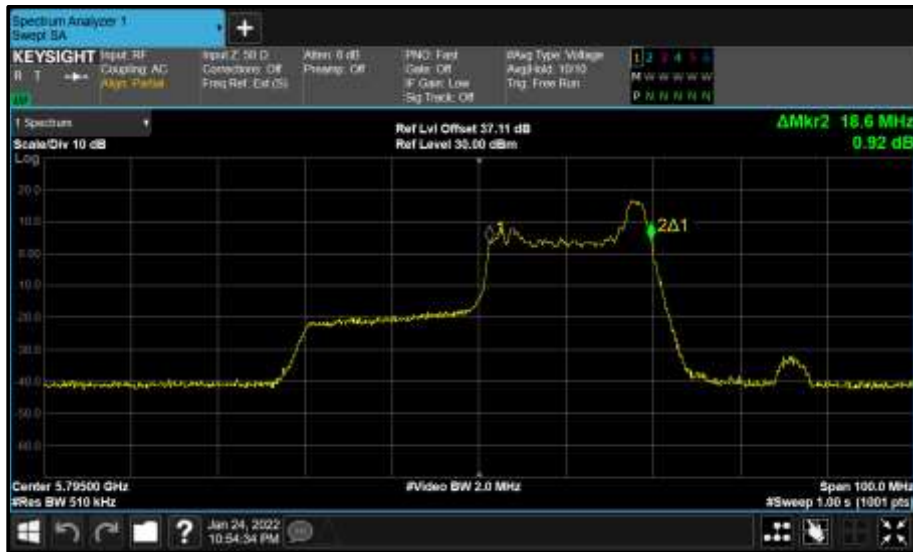
Figure 804 - Core 1 (B) 5795 MHz (CH159) 99% Bandwidth
