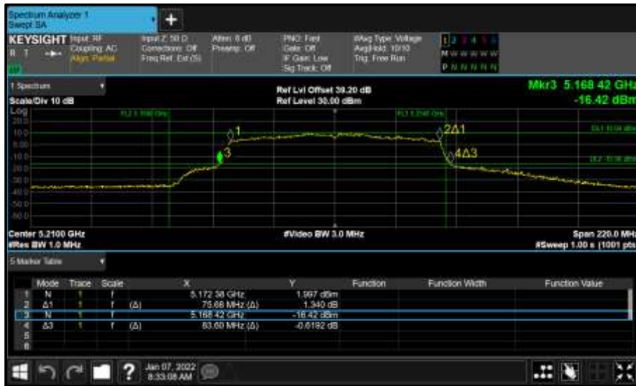
Figure 906 - Core 0 (A) 5210 MHz (CH42) 26 dB and 99% Bandwidth
