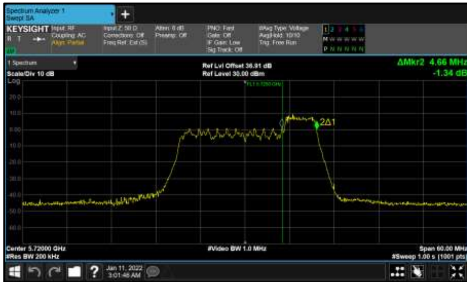
Figure 726 - Core 1 (B) 5720 MHz (CH144) 99% Bandwidth
