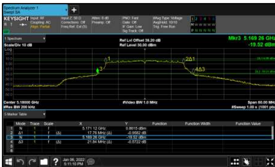
Figure 893 - Core 1 (B) 5180 MHz (CH36) 26 dB and 99% Bandwidth
