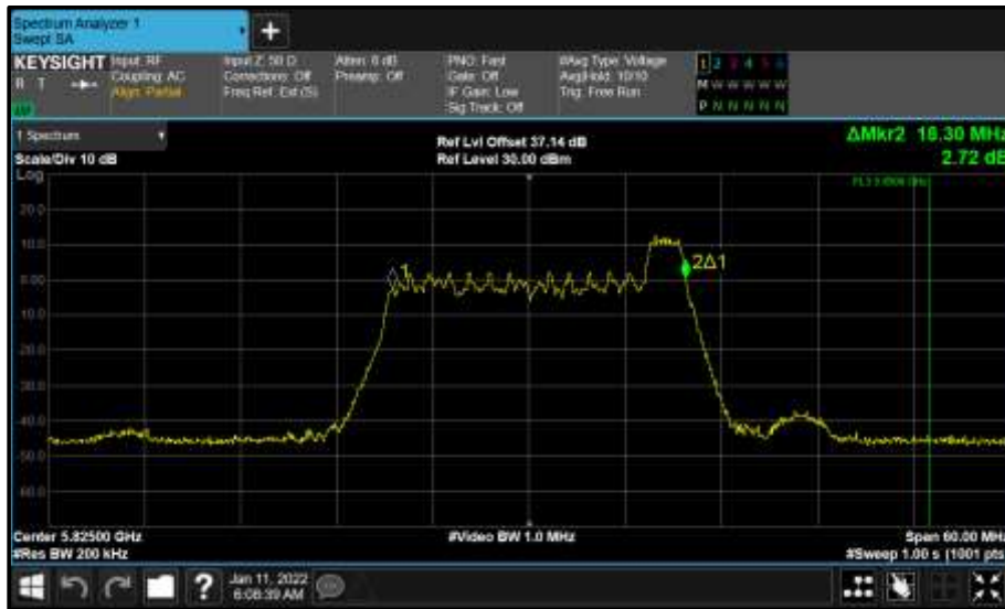
Figure 702 - Core 1 (B) 5825 MHz (CH165) 99% Bandwidth
