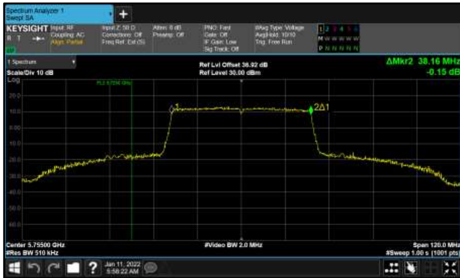
Figure 768 - Core 1 (B) 5755 MHz (CH151) 99% Bandwidth
