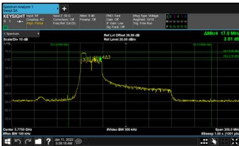
Figure 869 - Core 0 (A) 5775 MHz (CH155) 6 dB Bandwidth
