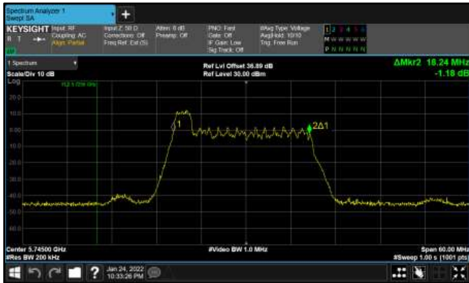
Figure 706 - Core 1 (B) 5745 MHz (CH149) 99% Bandwidth
