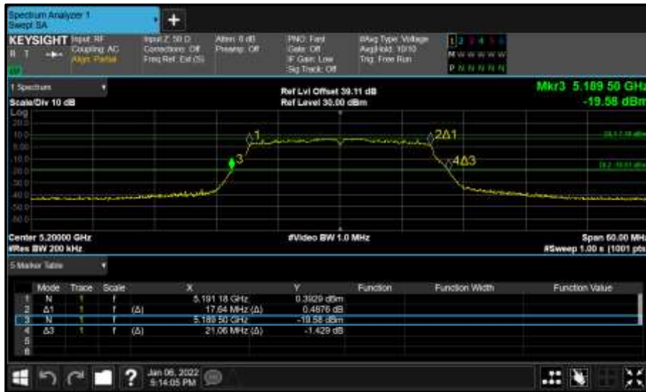
Figure 894 - Core 0 (A) 5200 MHz (CH40) 26 dB and 99% Bandwidth
