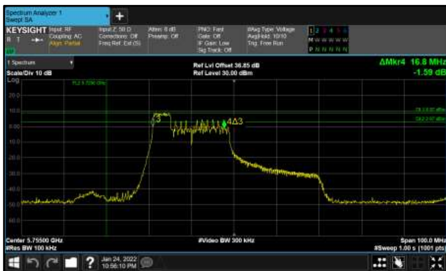
Figure 829 - Core 0 (A) 5755 MHz (CH151) 6 dB Bandwidth
