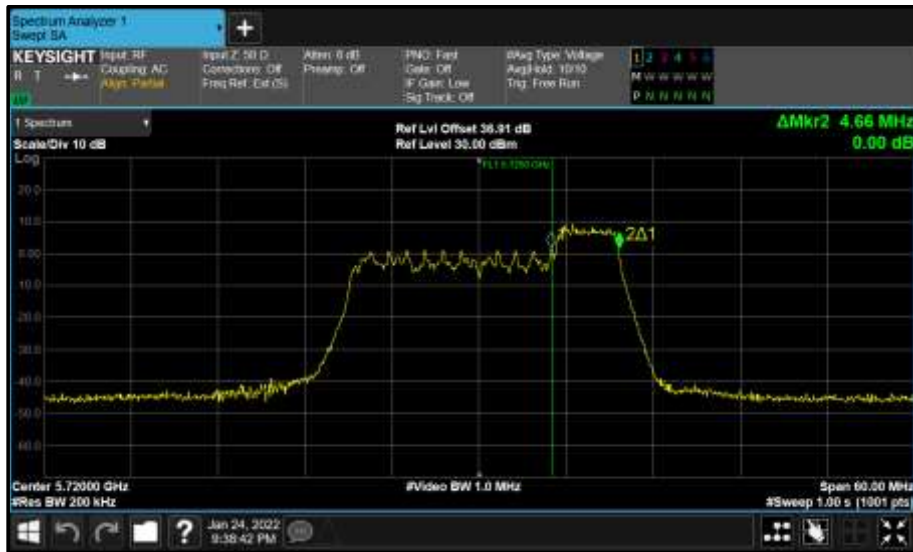
Figure 742 - Core 1 (B) 5720 MHz (CH144) 99% Bandwidth
