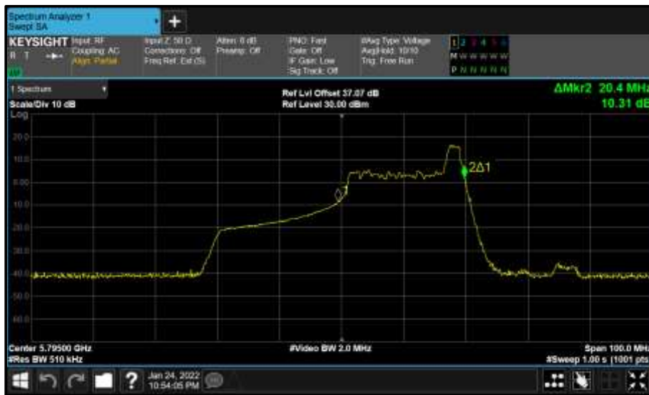
Figure 802 - Core 0 (A) 5795 MHz (CH159) 99% Bandwidth
