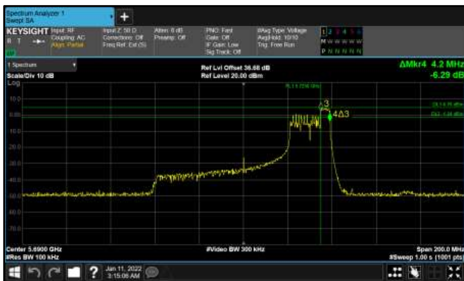
Figure 871 - Core 0 (A) 5690 MHz (CH138) 6 dB Bandwidth
