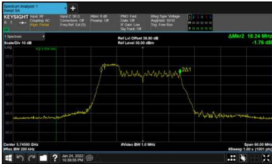
Figure 744 - Core 0 (A) 5745 MHz (CH149) 99% Bandwidth
