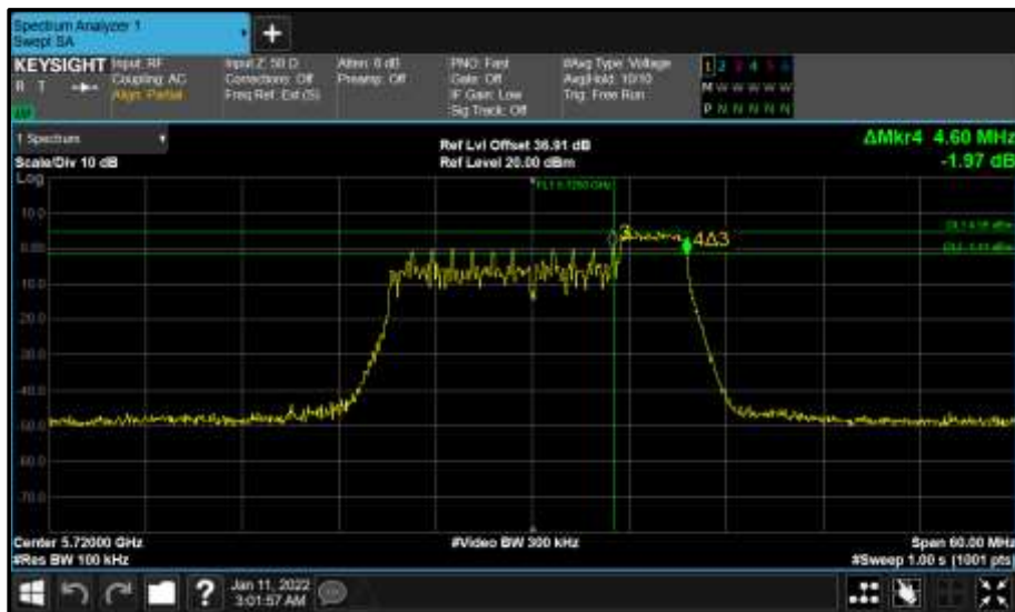
Figure 727 - Core 1 (B) 5720 MHz (CH144) 6 dB Bandwidth
