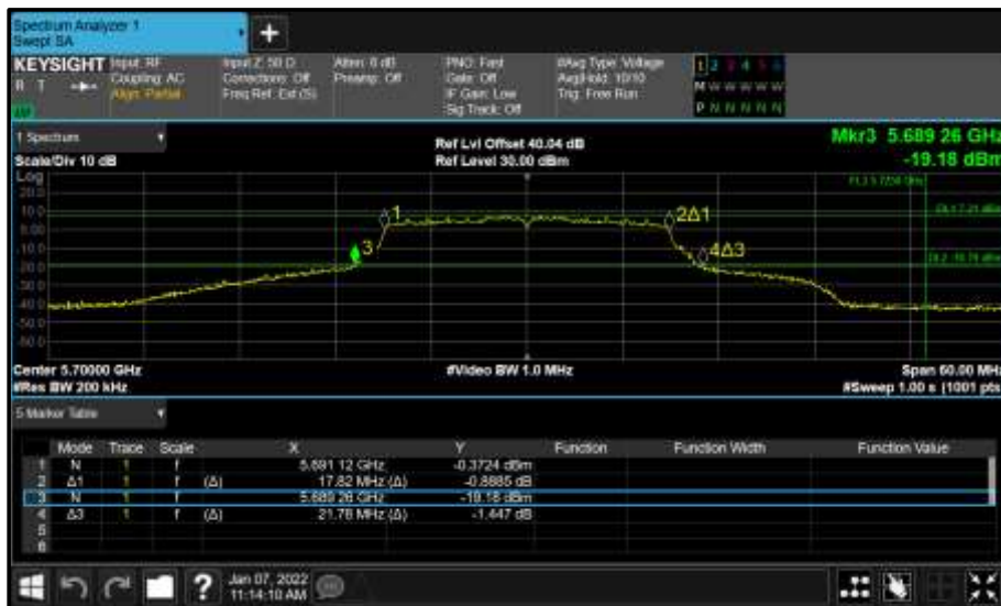
Figure 927 - Core 1 (B) 5700 MHz (CH140) 26 dB and 99% Bandwidth
