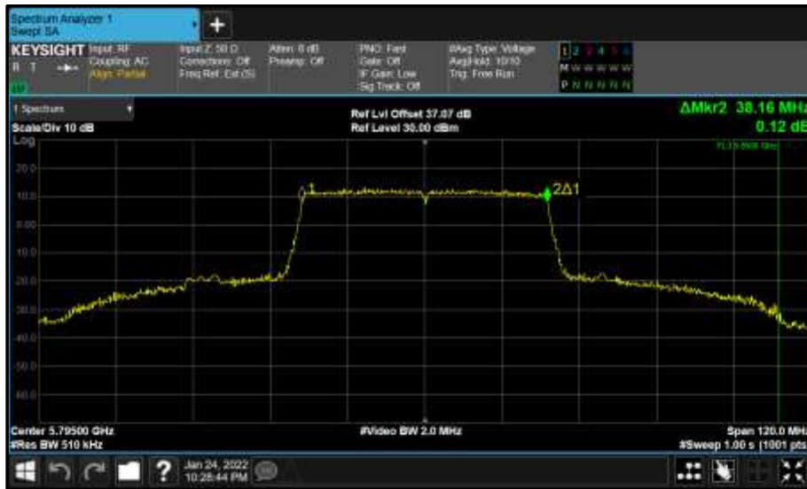
Figure 782 - Core 0 (A) 5795 MHz (CH159) 99% Bandwidth
