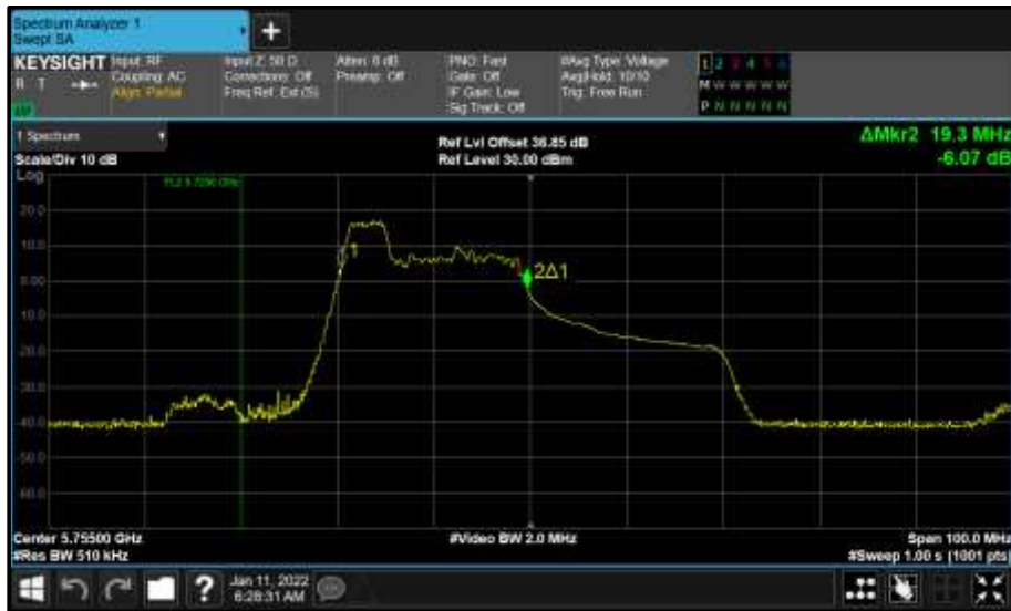
Figure 816 - Core 0 (A) 5755 MHz (CH151) 99% Bandwidth
