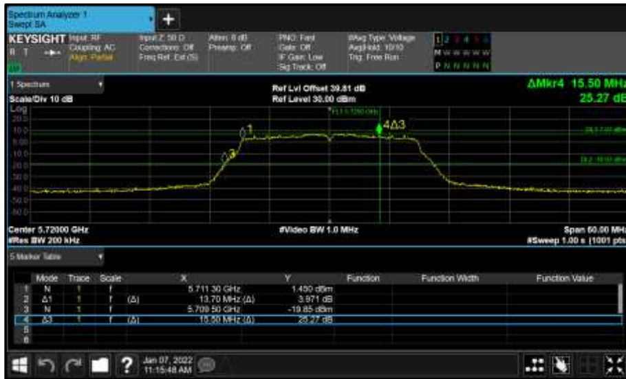
Figure 928 - Core 0 (A) 5720 MHz (CH144) 26 dB and 99% Bandwidth
