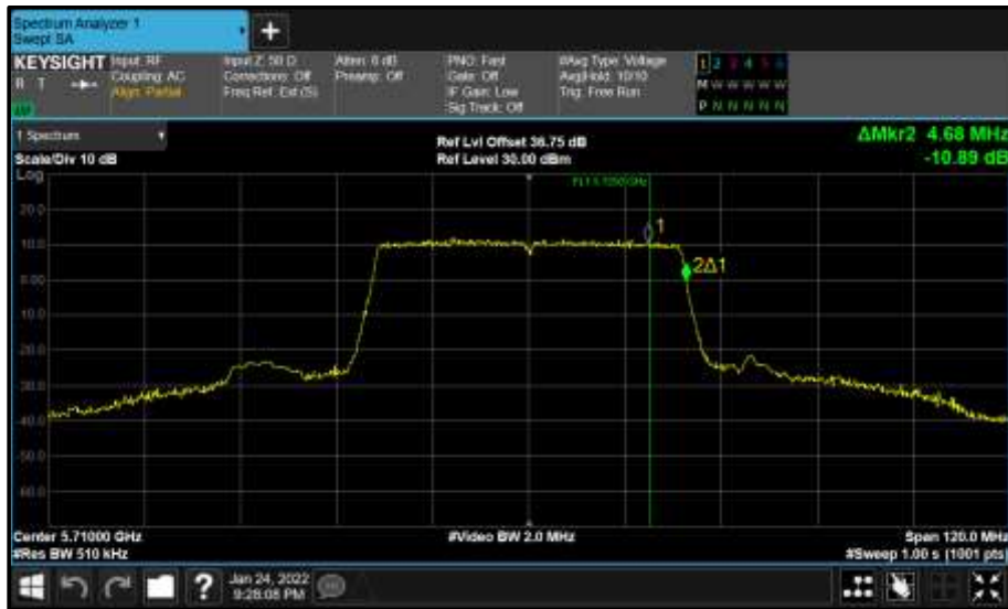
Figure 774 - Core 0 (A) 5710 MHz (CH142) 99% Bandwidth
