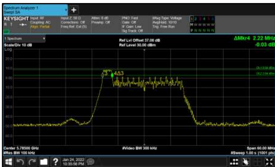
Figure 711 - Core 1 (B) 5785 MHz (CH157) 6 dB Bandwidth
