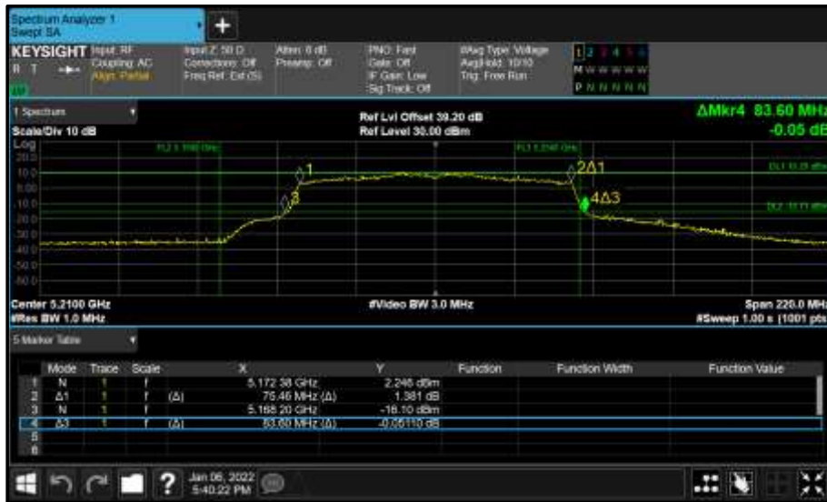
Figure 908 - Core 0 (A) 5210 MHz (CH42) 26 dB and 99% Bandwidth
