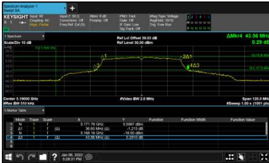
Figure 902 - Core 0 (A) 5190 MHz (CH38) 26 dB and 99% Bandwidth
