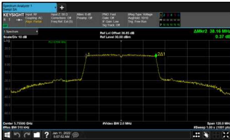
Figure 766 - Core 0 (A) 5755 MHz (CH151) 99% Bandwidth
