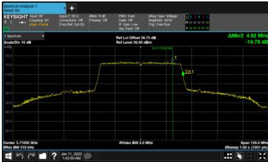
Figure 756 - Core 0 (A) 5710 MHz (CH142) 99% Bandwidth
