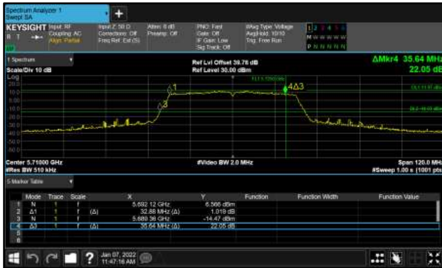
Figure 936 - Core 0 (A) 5710 MHz (CH142) 26 dB and 99% Bandwidth
