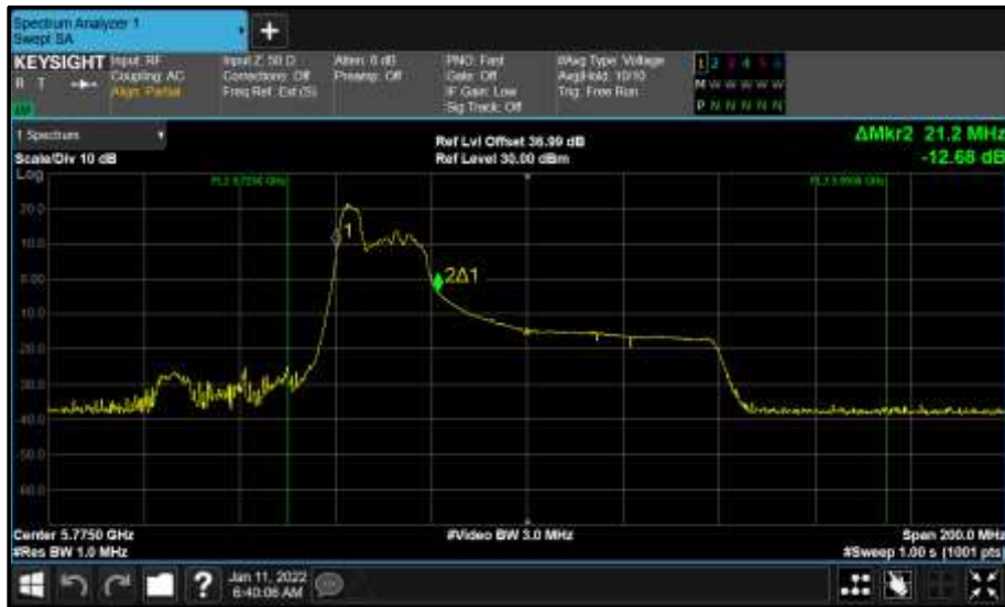
Figure 874 - Core 0 (A) 5775 MHz (CH155) 99% Bandwidth
