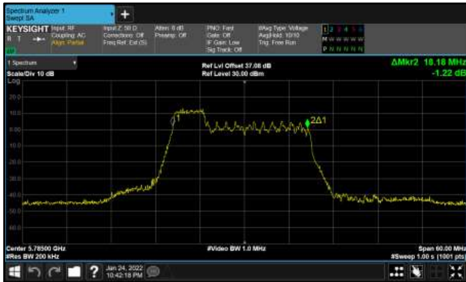
Figure 750 - Core 1 (B) 5785 MHz (CH157) 99% Bandwidth
