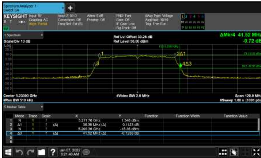
Figure 900 - Core 0 (A) 5230 MHz (CH46) 26 dB and 99% Bandwidth
