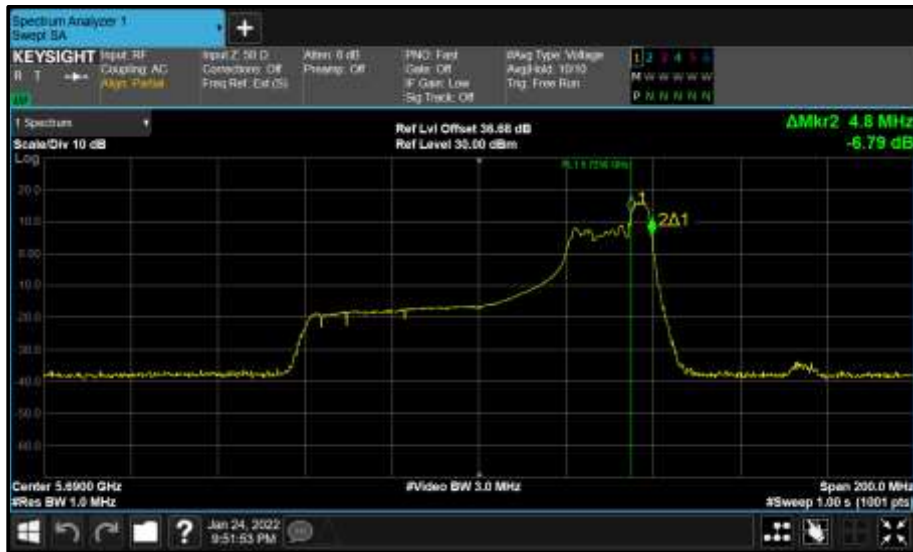
Figure 878 - Core 0 (A) 5690 MHz (CH138) 99% Bandwidth
