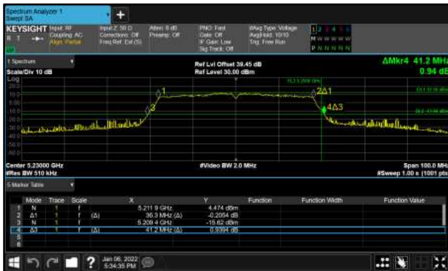
Figure 905 - Core 1 (B) 5230 MHz (CH46) 26 dB and 99% Bandwidth
