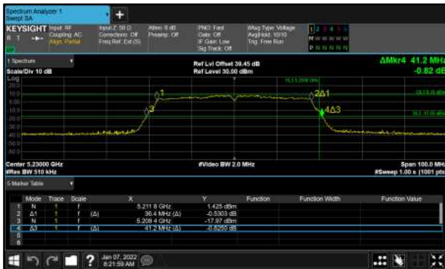
Figure 901 - Core 1 (B) 5230 MHz (CH46) 26 dB and 99% Bandwidth
