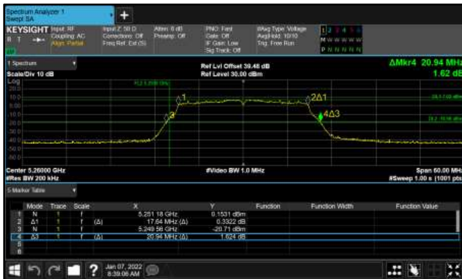
Figure 911 - Core 1 (B) 5260 MHz (CH52) 26 dB and 99% Bandwidth
