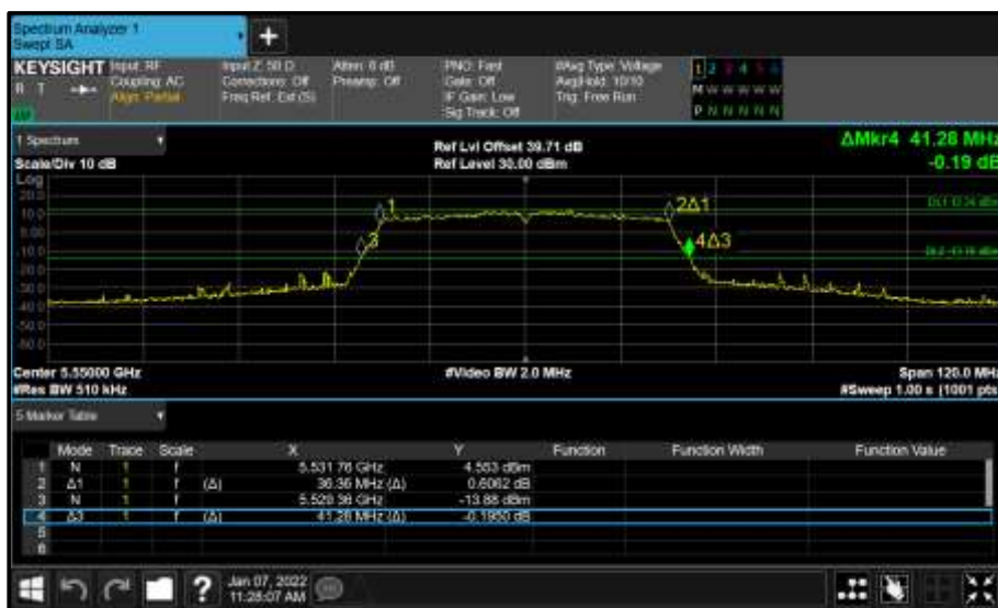
Figure 933 - Core 1 (B) 5550 MHz (CH110) 26 dB and 99% Bandwidth
