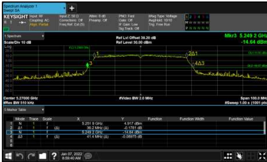
Figure 916 - Core 0 (A) 5270 MHz (CH54) 26 dB and 99% Bandwidth
