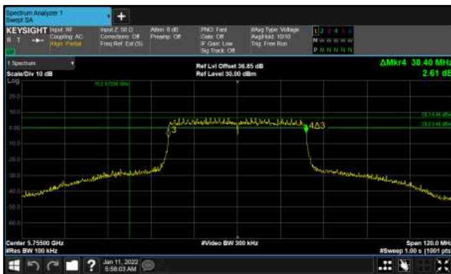
Figure 767 - Core 0 (A) 5755 MHz (CH151) 6 dB Bandwidth
