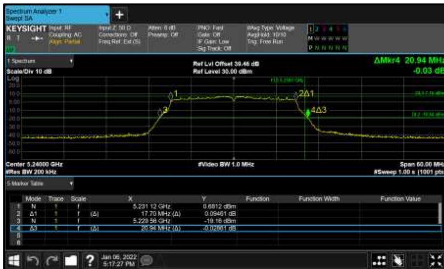
Figure 897 - Core 1 (B) 5240 MHz (CH48) 26 dB and 99% Bandwidth
