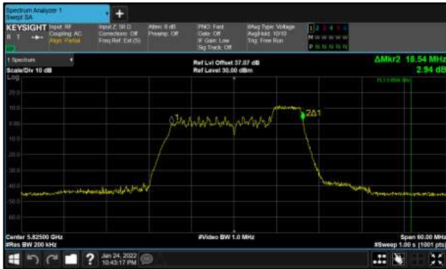
Figure 752 - Core 0 (A) 5825 MHz (CH165) 99% Bandwidth
