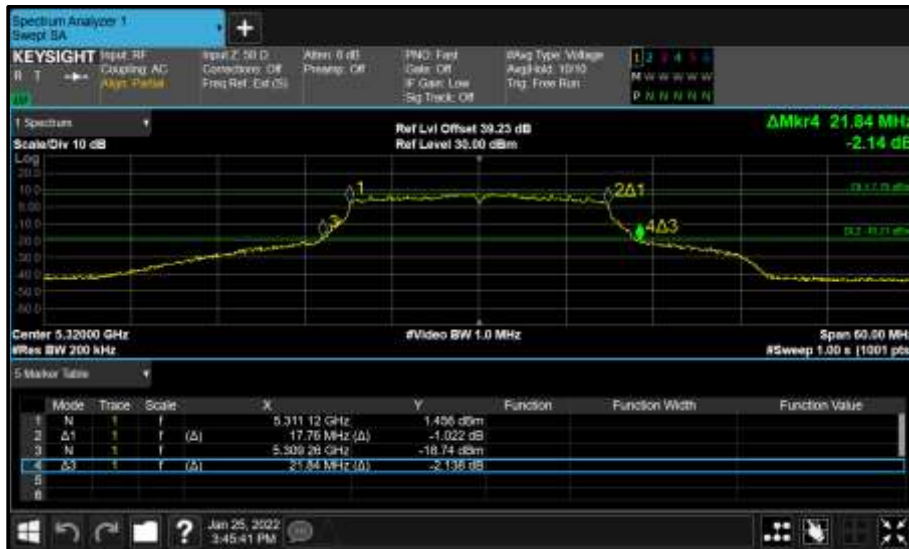
Figure 914- Core 0 (A) 5320 MHz (CH64) 26 dB and 99% Bandwidth
