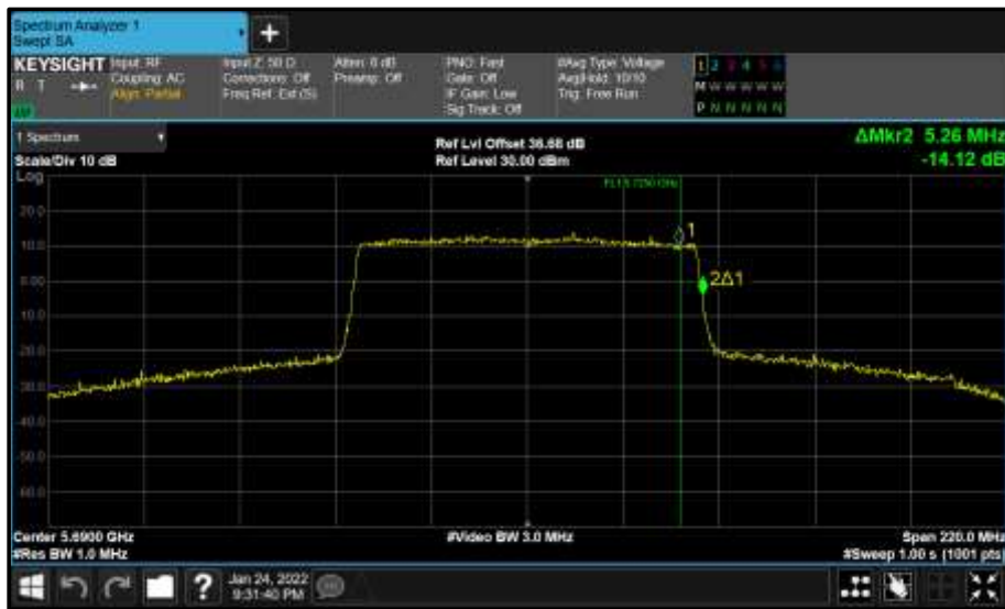
Figure 848 - Core 0 (A) 5690 MHz (CH138) 99% Bandwidth
