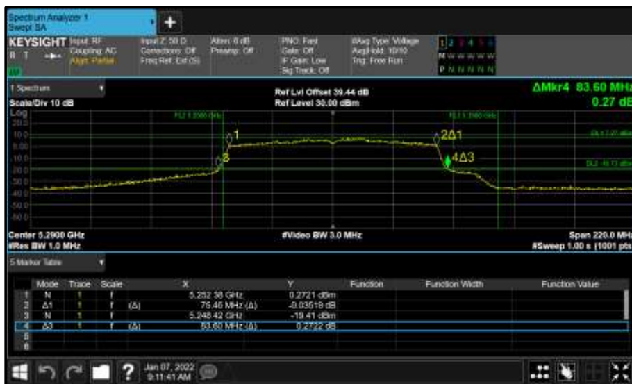
Figure 921 - Core 1 (B) 5290 MHz (CH58) 26 dB and 99% Bandwidth
