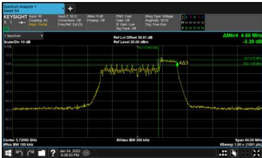
Figure 743 - Core 1 (B) 5720 MHz (CH144) 6 dB Bandwidth
