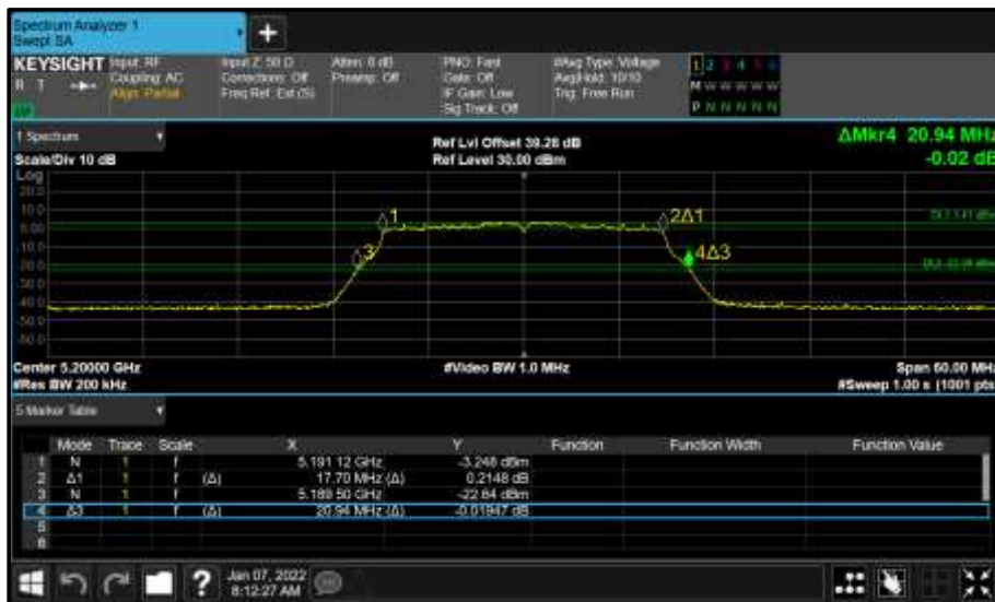
Figure 889 - Core 1 (B) 5200 MHz (CH40) 26 dB and 99% Bandwidth
