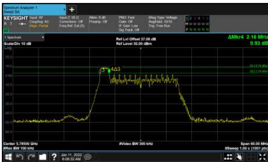
Figure 699 - Core 1 (B) 5785 MHz (CH157) 6 dB Bandwidth
