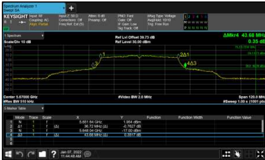
Figure 934 - Core 0 (A) 5670 MHz (CH134) 26 dB and 99% Bandwidth
