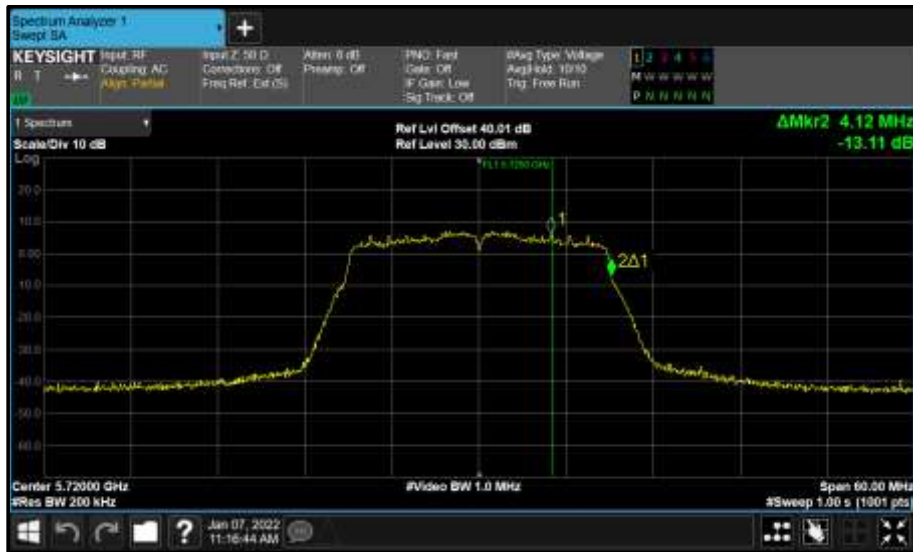
Figure 946 - Core 1 (B) 5720 MHz (CH144) 99% Bandwidth
