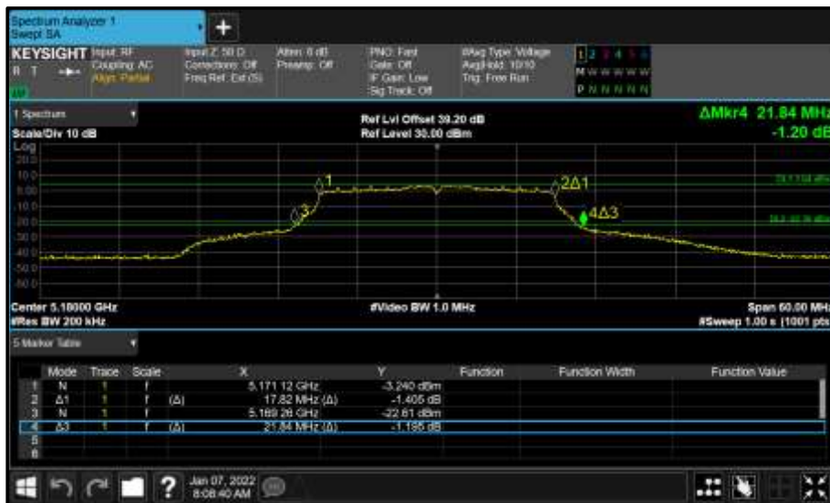
Figure 887 - Core 1 (B) 5180 MHz (CH36) 26 dB and 99% Bandwidth
