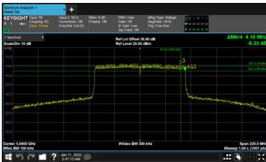
Figure 843 - Core 1 (B) 5690 MHz (CH138) 6 dB Bandwidth
