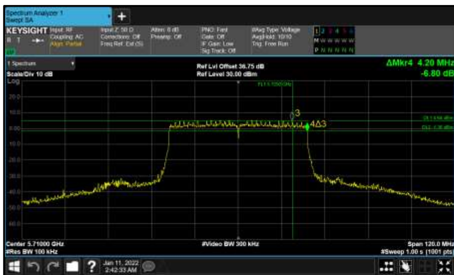
Figure 763 - Core 0 (A) 5710 MHz (CH142) 6 dB Bandwidth
