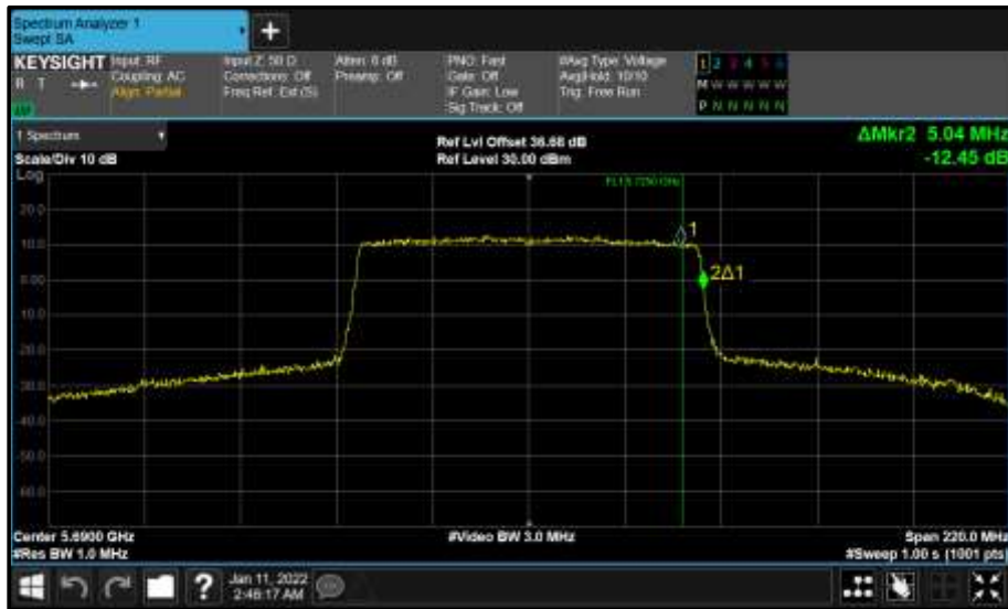
Figure 840 - Core 0 (A) 5690 MHz (CH138) 99% Bandwidth
