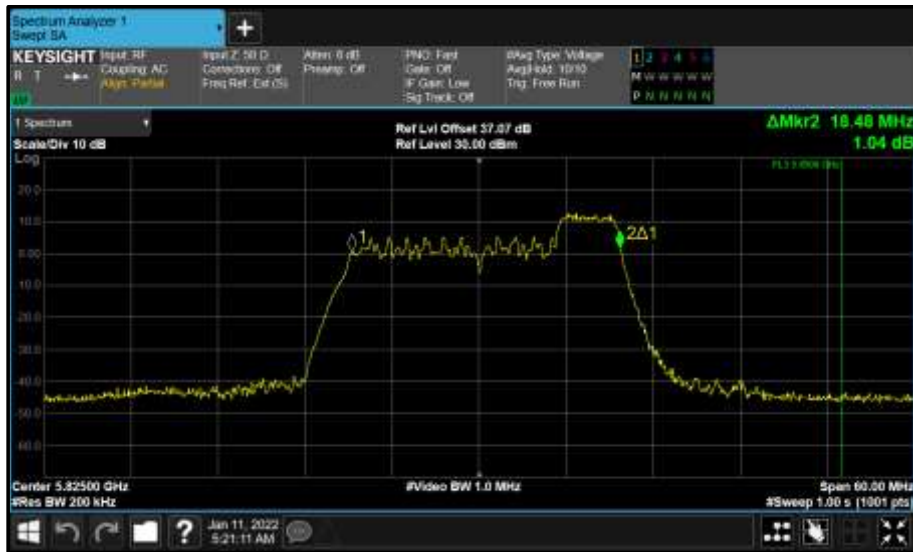
Figure 722 - Core 0 (A) 5825 MHz (CH165) 99% Bandwidth
