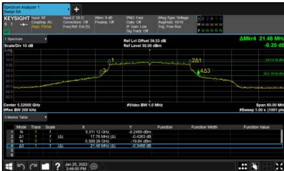
Figure 915- Core 1 (B) 5320 MHz (CH64) 26 dB and 99% Bandwidth
