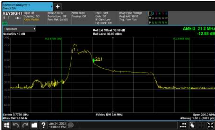
Figure 882 - Core 0 (A) 5775 MHz (CH155) 99% Bandwidth
