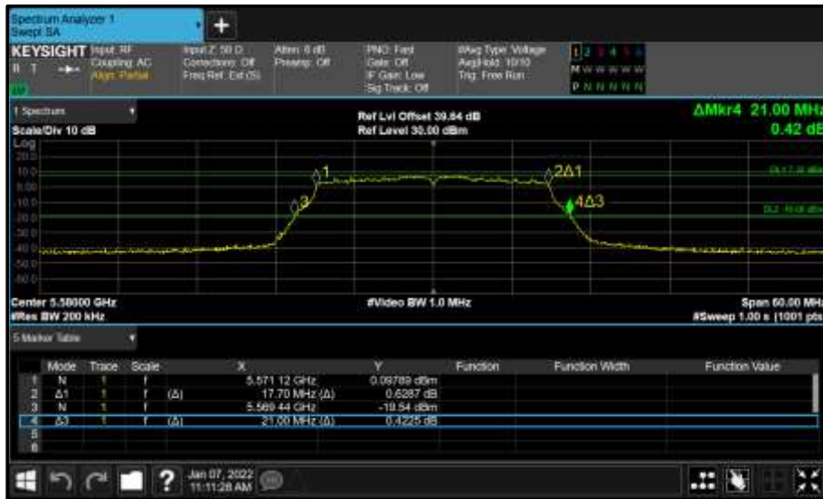
Figure 924 - Core 0 (A) 5580 MHz (CH116) 26 dB and 99% Bandwidth
