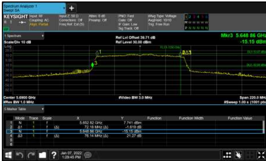
Figure 942 - Core 0 (A) 5690 MHz (CH138) 26 dB and 99% Bandwidth
