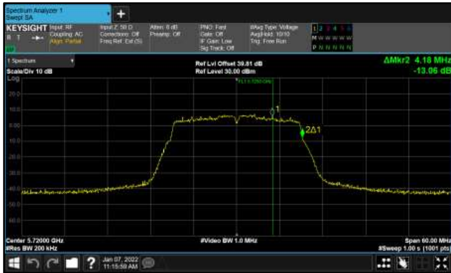
Figure 944 - Core 0 (A) 5720 MHz (CH144) 99% Bandwidth
