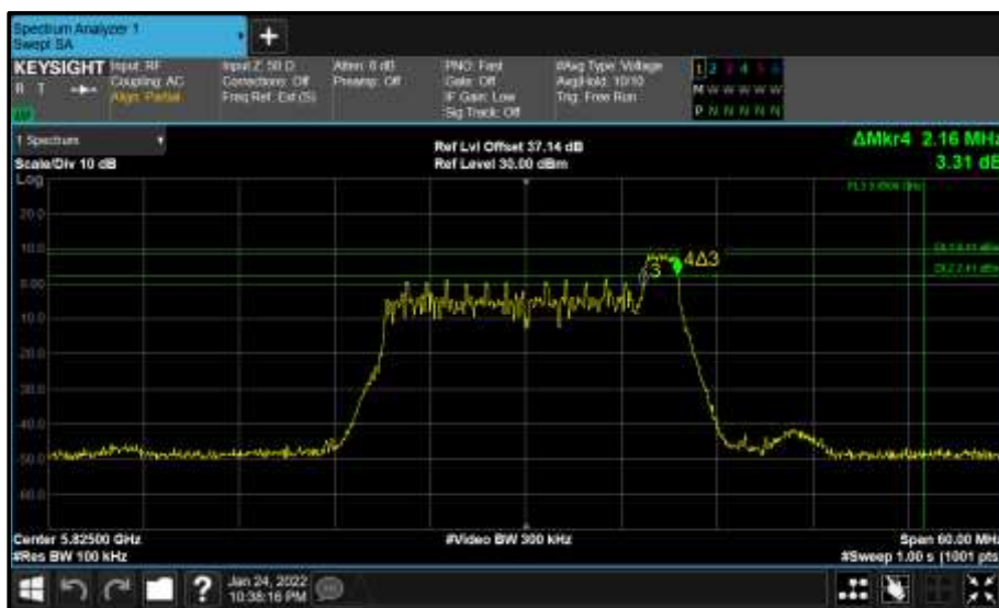
Figure 715 - Core 1 (B) 5825 MHz (CH165) 6 dB Bandwidth
