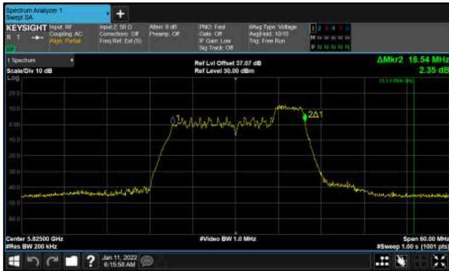
Figure 736 - Core 0 (A) 5825 MHz (CH165) 99% Bandwidth
