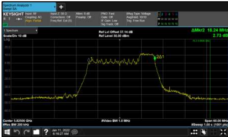
Figure 738 - Core 1 (B) 5825 MHz (CH165) 99% Bandwidth
