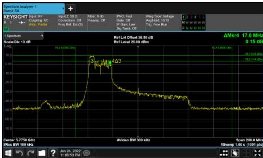
Figure 883 - Core 0 (A) 5775 MHz (CH155) 6 dB Bandwidth
