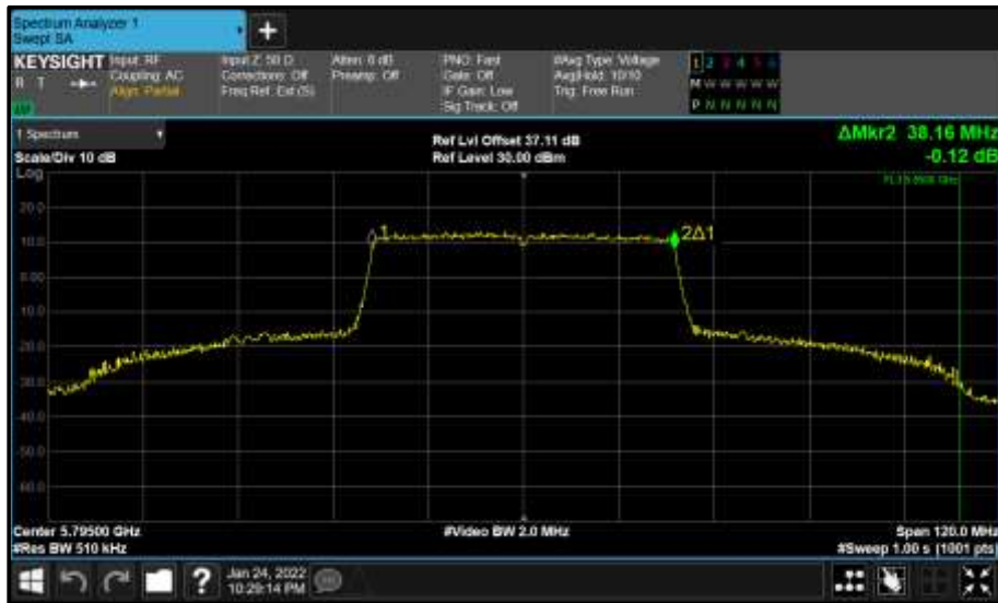
Figure 784 - Core 1 (B) 5795 MHz (CH159) 99% Bandwidth
