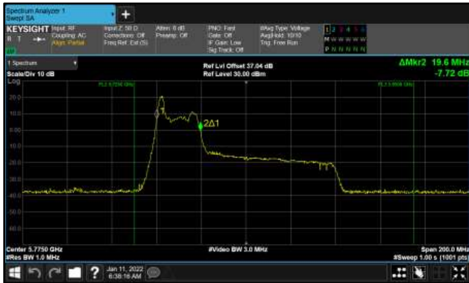
Figure 860 - Core 1 (B) 5775 MHz (CH155) 99% Bandwidth
