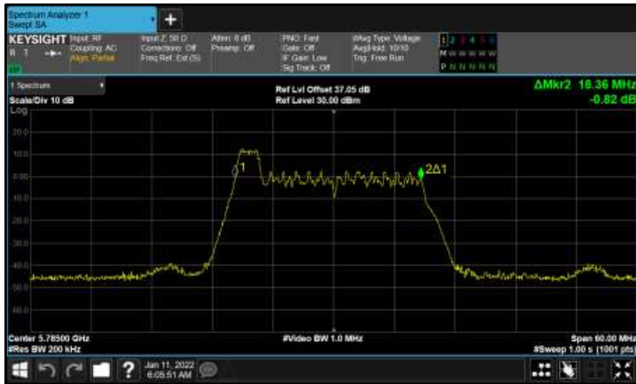
Figure 696 - Core 0 (A) 5785 MHz (CH157) 99% Bandwidth
