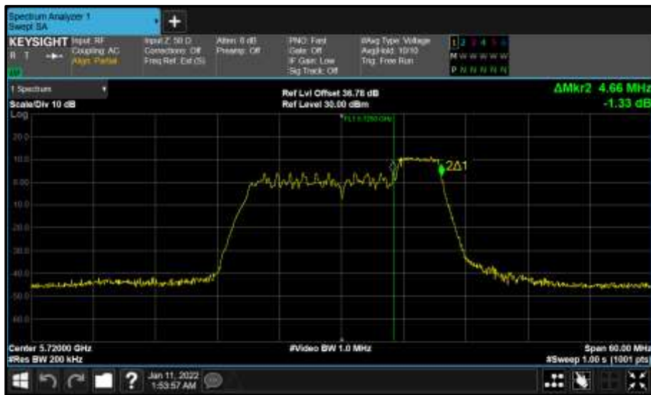
Figure 716 - Core 0 (A) 5720 MHz (CH144) 99% Bandwidth
