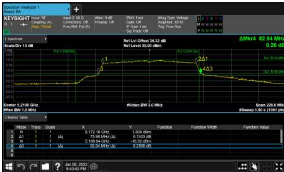
Figure 909 - Core 1 (B) 5210 MHz (CH42) 26 dB and 99% Bandwidth
