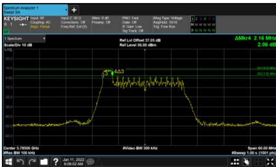
Figure 697 - Core 0 (A) 5785 MHz (CH157) 6 dB Bandwidth
