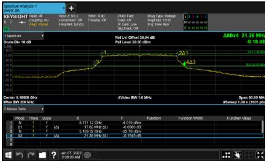
Figure 886 - Core 0 (A) 5180 MHz (CH36) 26 dB and 99% Bandwidth
