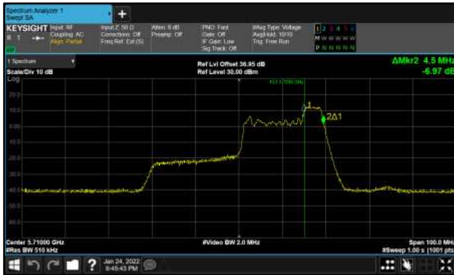
Figure 826 - Core 1 (B) 5710 MHz (CH142) 99% Bandwidth
