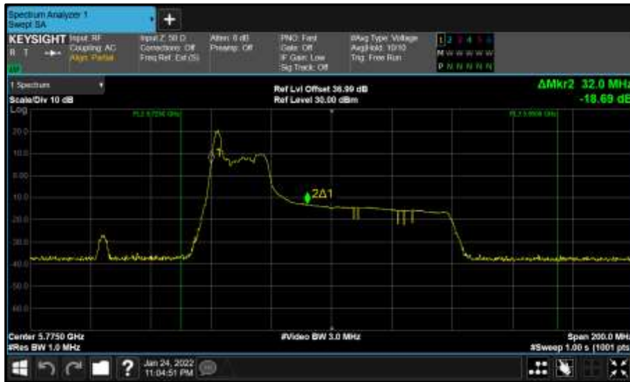
Figure 862 - Core 0 (A) 5775 MHz (CH155) 99% Bandwidth
