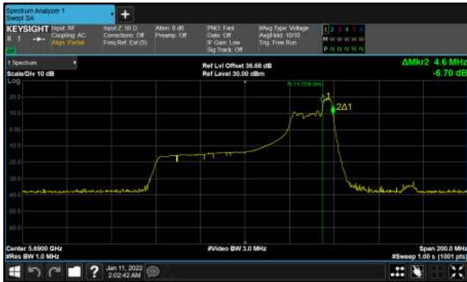
Figure 866 - Core 0 (A) 5690 MHz (CH138) 99% Bandwidth
