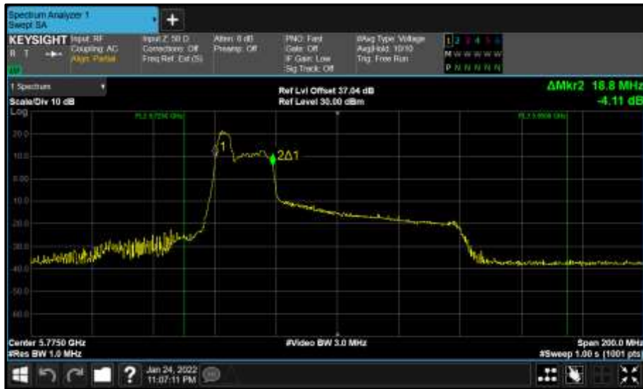
Figure 884 - Core 1 (B) 5775 MHz (CH155) 99% Bandwidth
