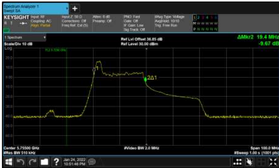
Figure 798 - Core 0 (A) 5755 MHz (CH151) 99% Bandwidth
