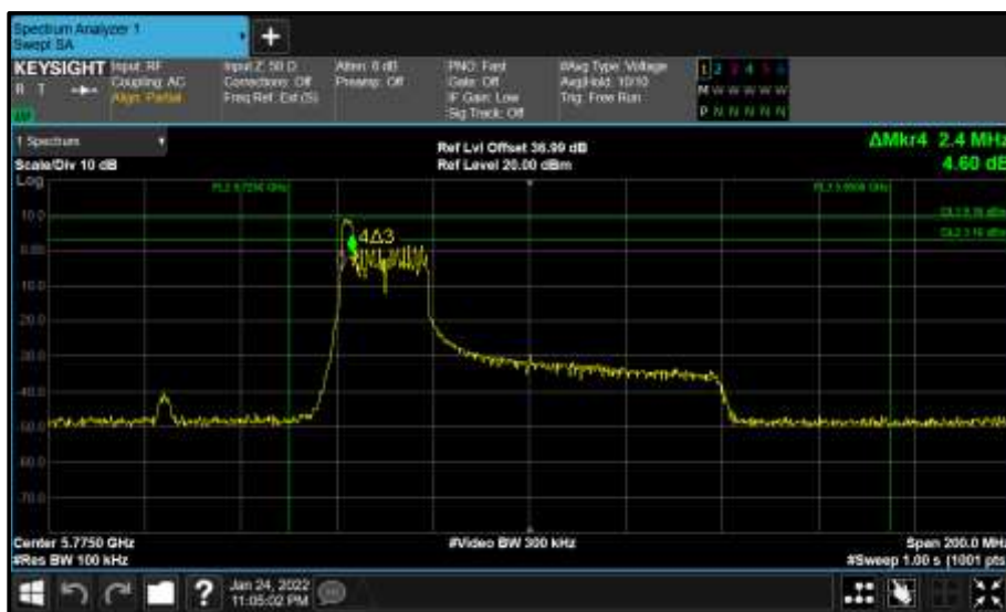
Figure 863 - Core 0 (A) 5775 MHz (CH155) 6 dB Bandwidth
