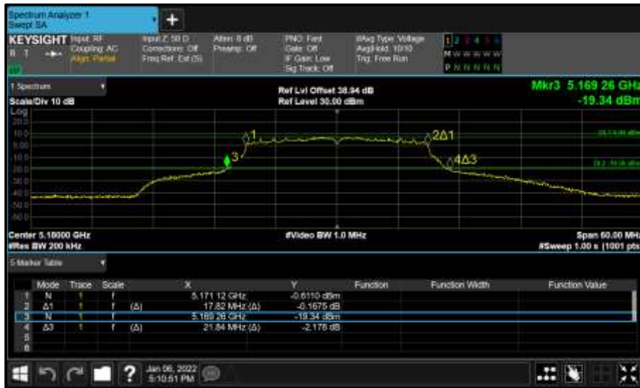
Figure 892 - Core 0 (A) 5180 MHz (CH36) 26 dB and 99% Bandwidth
