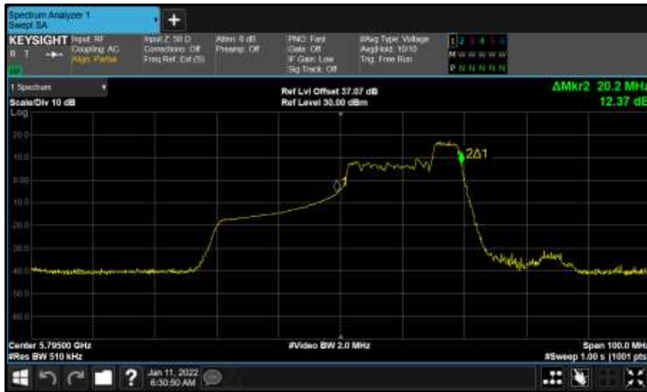
Figure 820 - Core 0 (A) 5795 MHz (CH159) 99% Bandwidth
