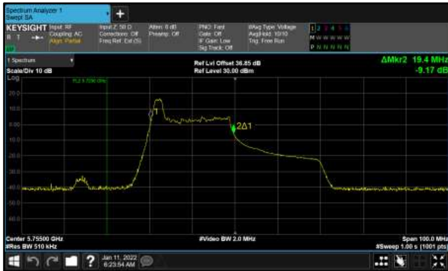
Figure 790 - Core 0 (A) 5755 MHz (CH151) 99% Bandwidth
