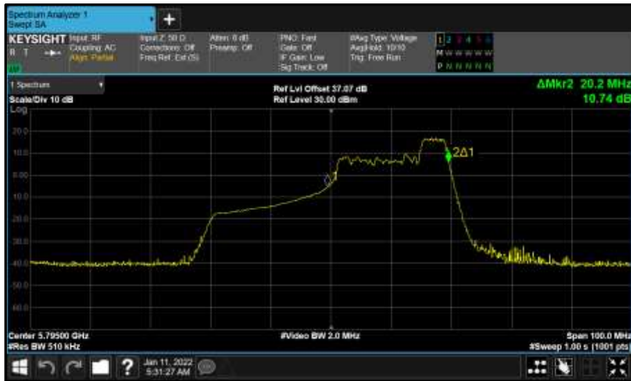
Figure 810 - Core 0 (A) 5795 MHz (CH159) 99% Bandwidth
