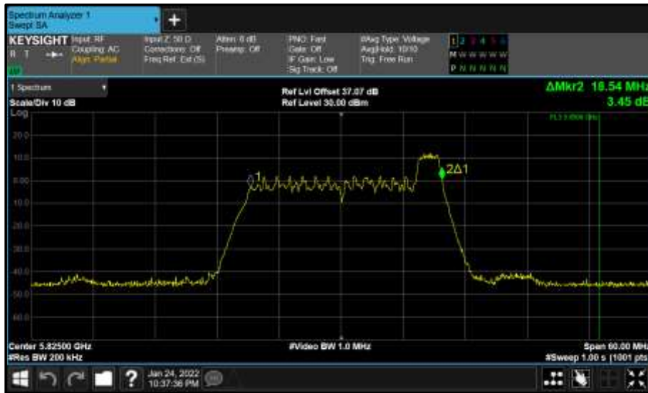
Figure 712 - Core 0 (A) 5825 MHz (CH165) 99% Bandwidth
