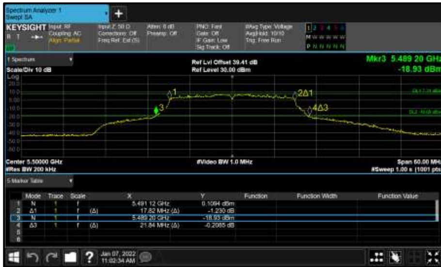
Figure 922 - Core 0 (A) 5500 MHz (CH100) 26 dB and 99% Bandwidth
