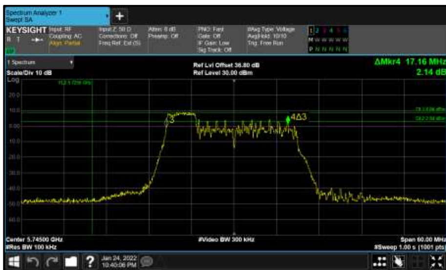
Figure 745 - Core 0 (A) 5745 MHz (CH149) 6 dB Bandwidth
