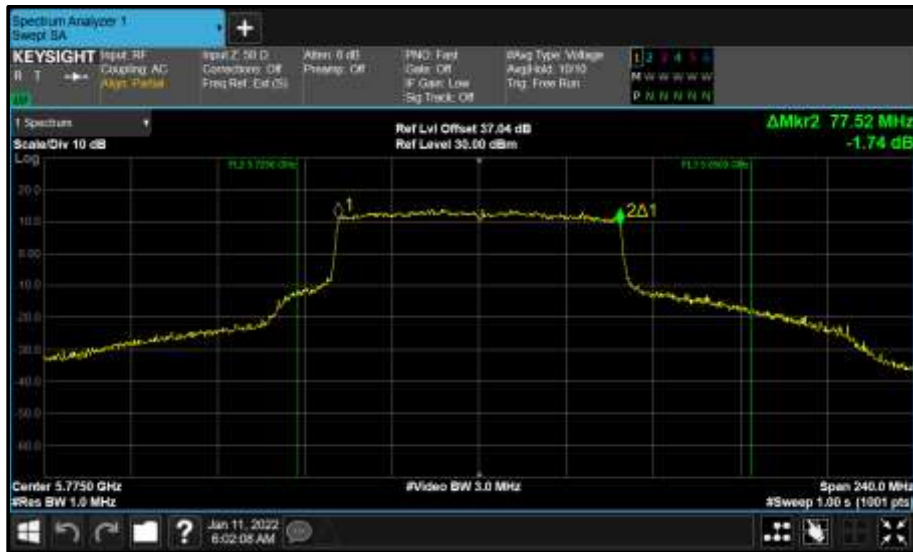
Figure 846 - Core 1 (B) 5775 MHz (CH155) 99% Bandwidth
