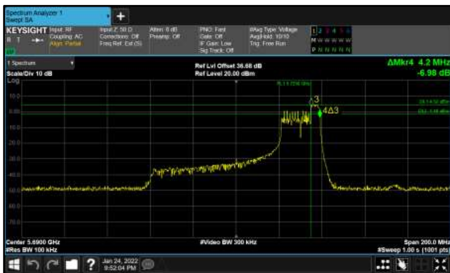
Figure 879 - Core 0 (A) 5690 MHz (CH138) 6 dB Bandwidth
