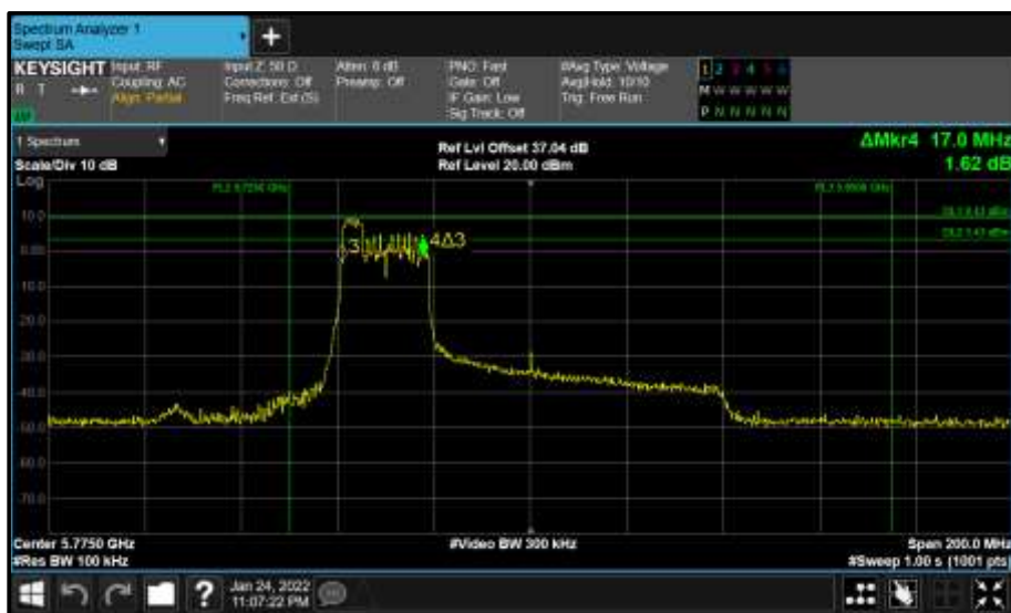
Figure 885 - Core 1 (B) 5775 MHz (CH155) 6 dB Bandwidth
