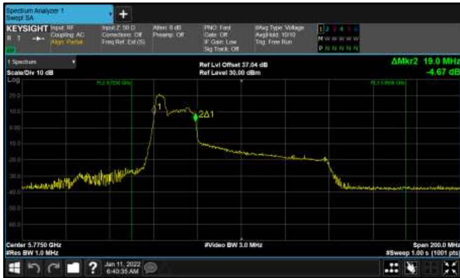
Figure 876 - Core 1 (B) 5775 MHz (CH155) 99% Bandwidth
