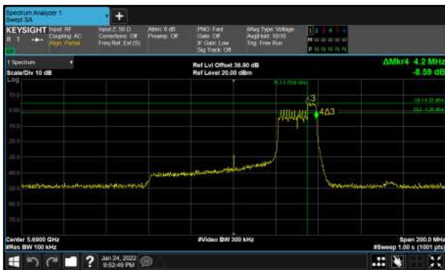
Figure 881 - Core 1 (B) 5690 MHz (CH138) 6 dB Bandwidth
