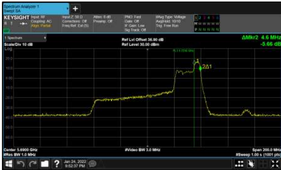
Figure 880 - Core 1 (B) 5690 MHz (CH138) 99% Bandwidth
