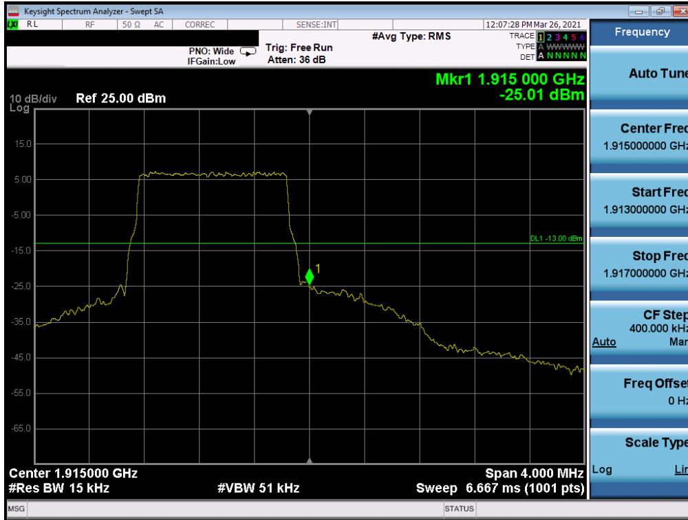
Plot 7-40. Upper Band Edge Plot (LTE Band 25 – 1.4MHz QPSK – Full RB Configuration)
