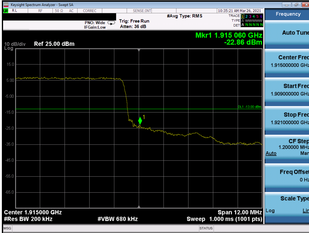
Plot 7-56. Upper Band Edge Plot (LTE Band 25 - 15MHz QPSK – Full RB Configuration)
