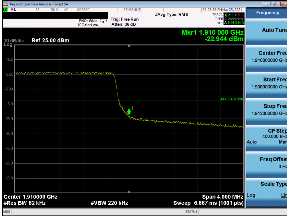
Plot 7-72. Upper Band Edge Plot (LTE Band 2 - 5MHz QPSK – Full RB Configuration)
