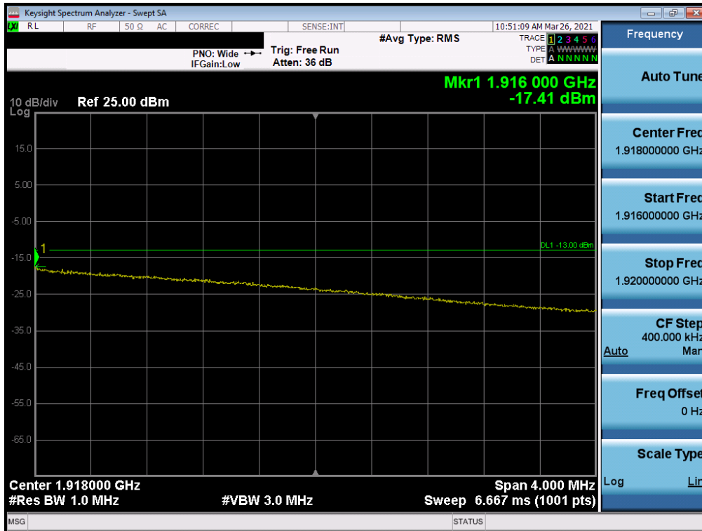
Plot 7-53. Extended Upper Band Edge Plot (LTE Band 25 - 10MHz QPSK – Full RB Configuration)
