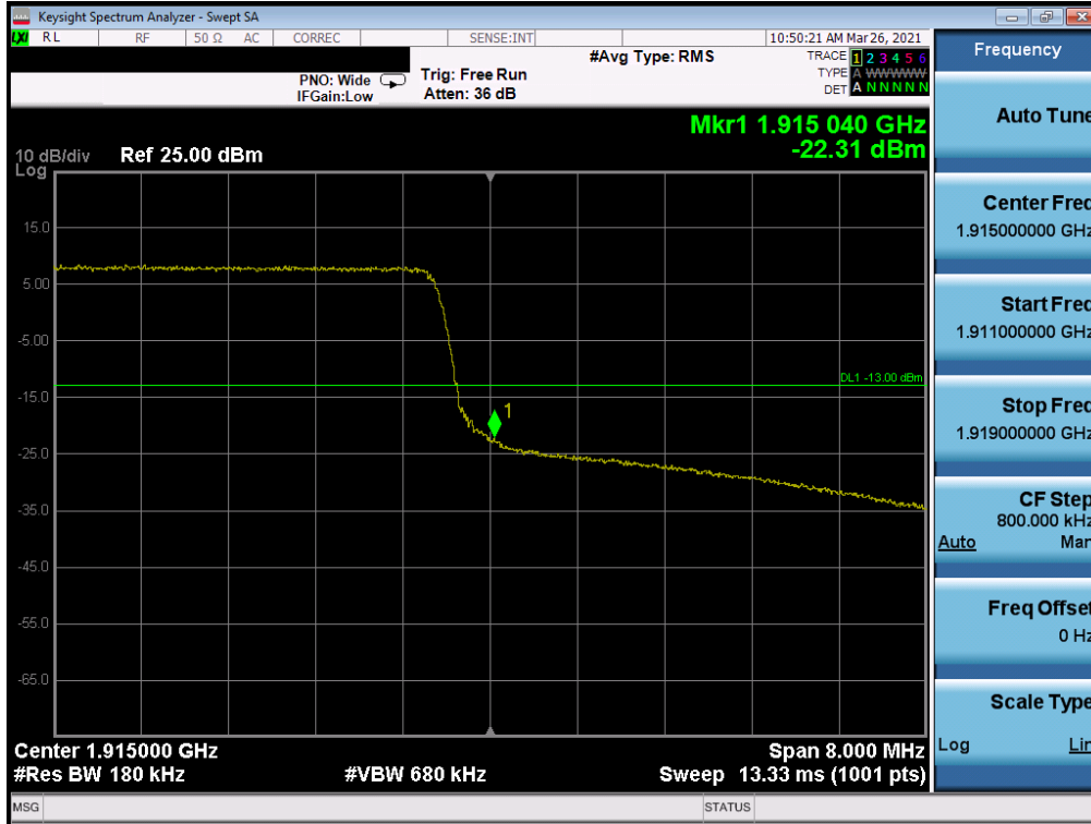
Plot 7-52. Upper Band Edge Plot (LTE Band 25 - 10MHz QPSK – Full RB Configuration)
