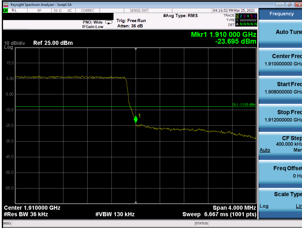
Plot 7-68. Upper Band Edge Plot (LTE Band 2 - 3MHz QPSK – Full RB Configuration)
