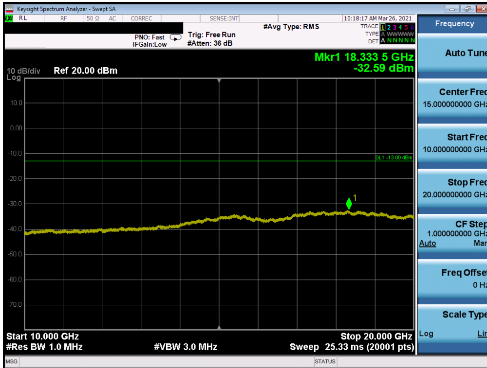
Plot 7-28. CSE (LTE Band 25/2 - 20MHz QPSK - RB Size 1, RB Offset 0 - High Channel)
