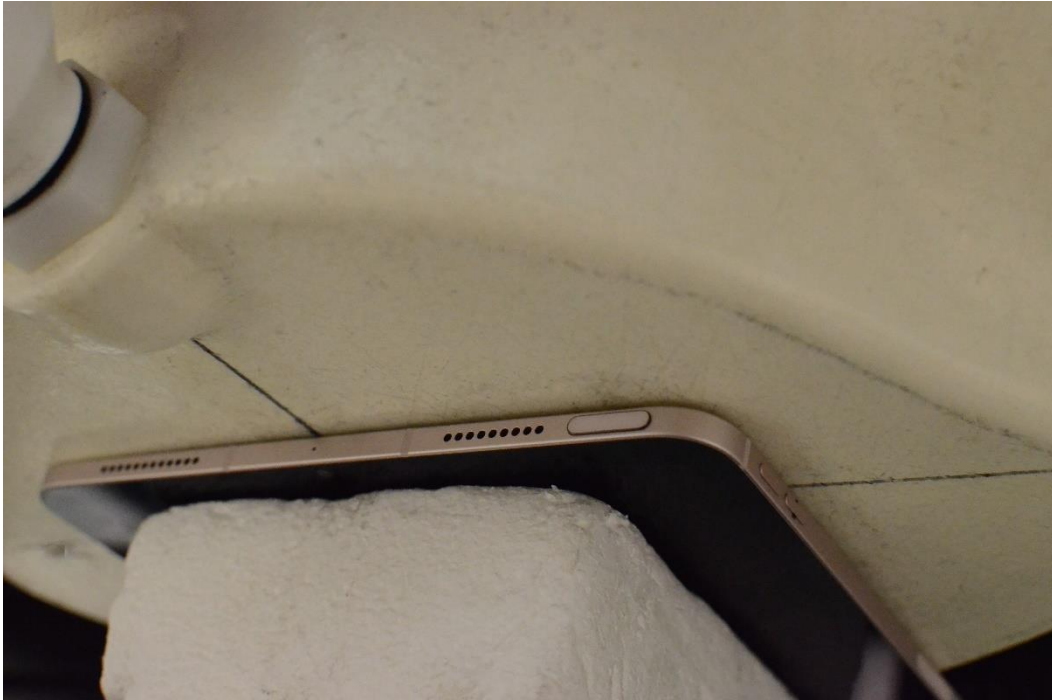
SAR Test Setup Photo 1: Body, Back Side at 0.0 cm – Antenna 3a/3b/4
