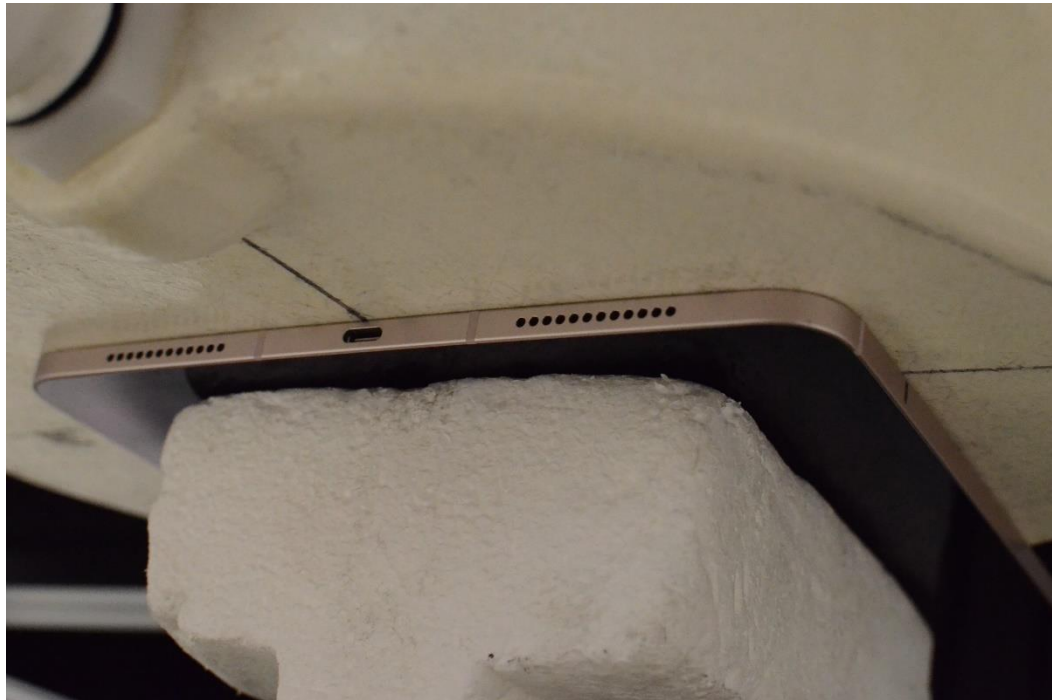
SAR Test Setup Photo 2: Body, Back Side at 0.0 cm – Antenna 1a/1b/2a/2b
