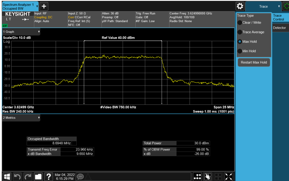
Plot 7-1. Occupied Bandwidth Plot (NR Band n48 - 10MHz \pi/2 BPSK - Full RB Configuration)
