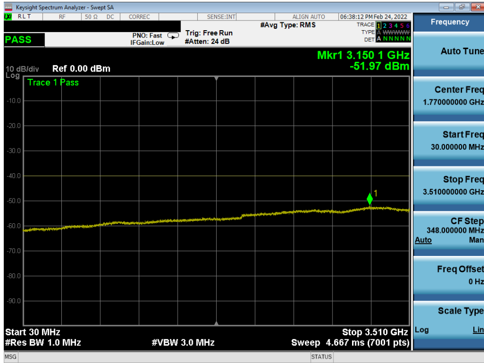
Plot 7-16. Conducted Spurious Plot (NR Band n48 - 40MHz DFT-s-OFDM QPSK - Low Channel)
