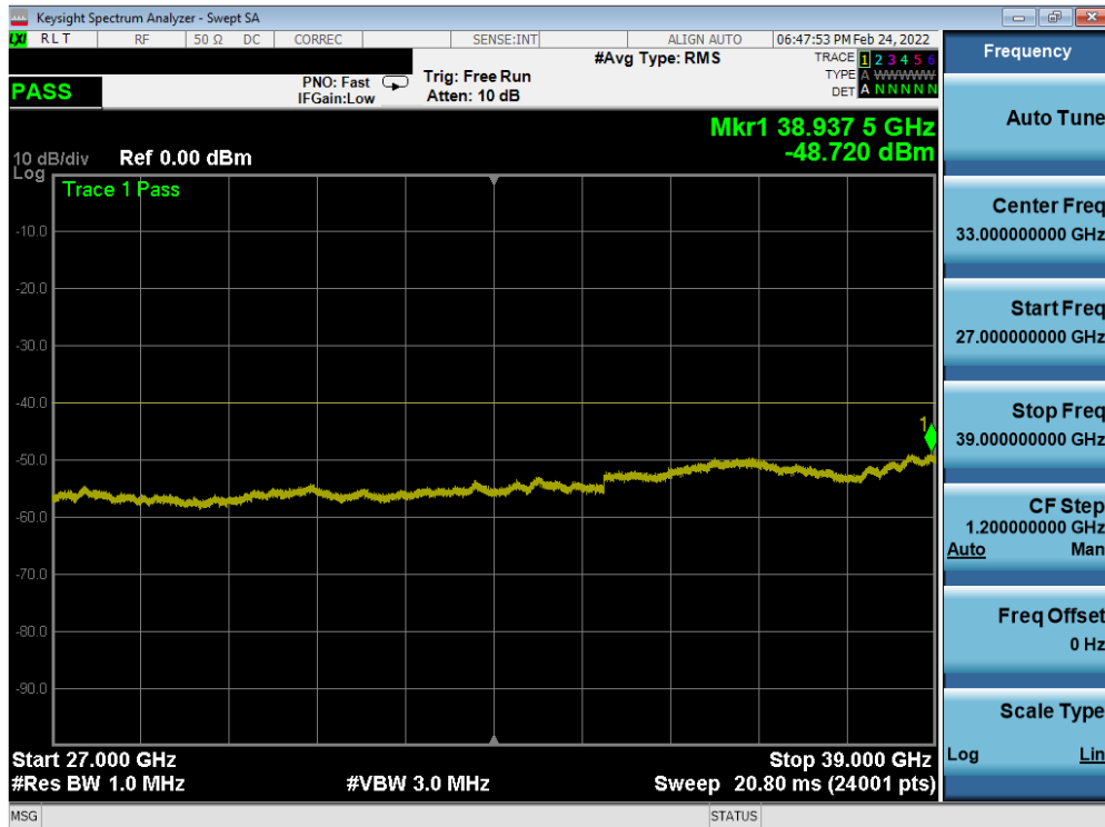
Plot 7-27. Conducted Spurious Plot (NR Band n48 - 40MHz DFT-s-OFDM QPSK - High Channel)
