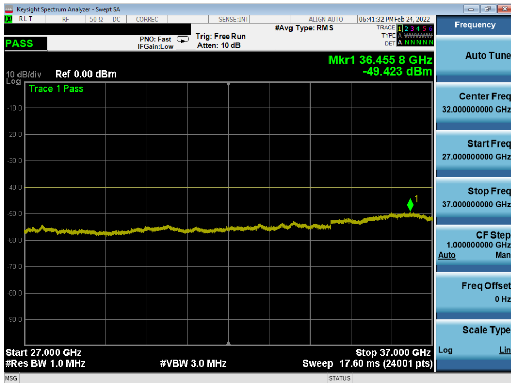
Plot 7-19. Conducted Spurious Plot (NR Band n48 - 40MHz DFT-s-OFDM QPSK - Low Channel)
