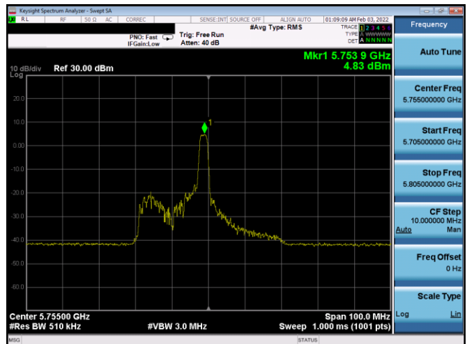
Plot 7-408. PSD CDD Primary Antenna 1b (40MHz BW 11ax Index 8 - RU26 - Ch.151)
