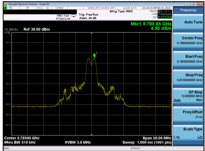
Plot 7-400. PSD CDD Primary Antenna 1b (20MHz BW 11ax Index 4 – RU26 – Ch.157)
