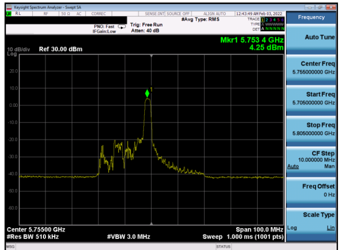
Plot 7-407. PSD CDD Primary Antenna 2b (40MHz BW 11ax Index 8 - RU26 - Ch.151)
