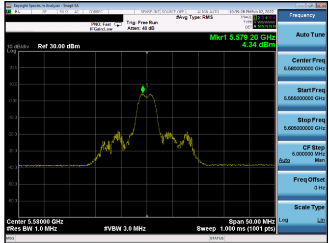
Plot 7-376. PSD CDD Primary Antenna 1b (20MHz BW 11ax Index 4 – RU26 – Ch.116)
