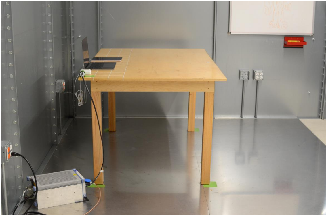
Figure 4: AC Line Conducted Emissions (Side View)
