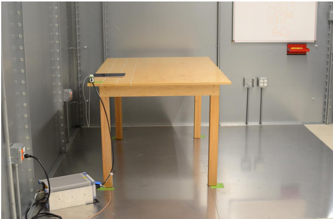
Figure 2: AC Line Conducted Emissions (Side View)
