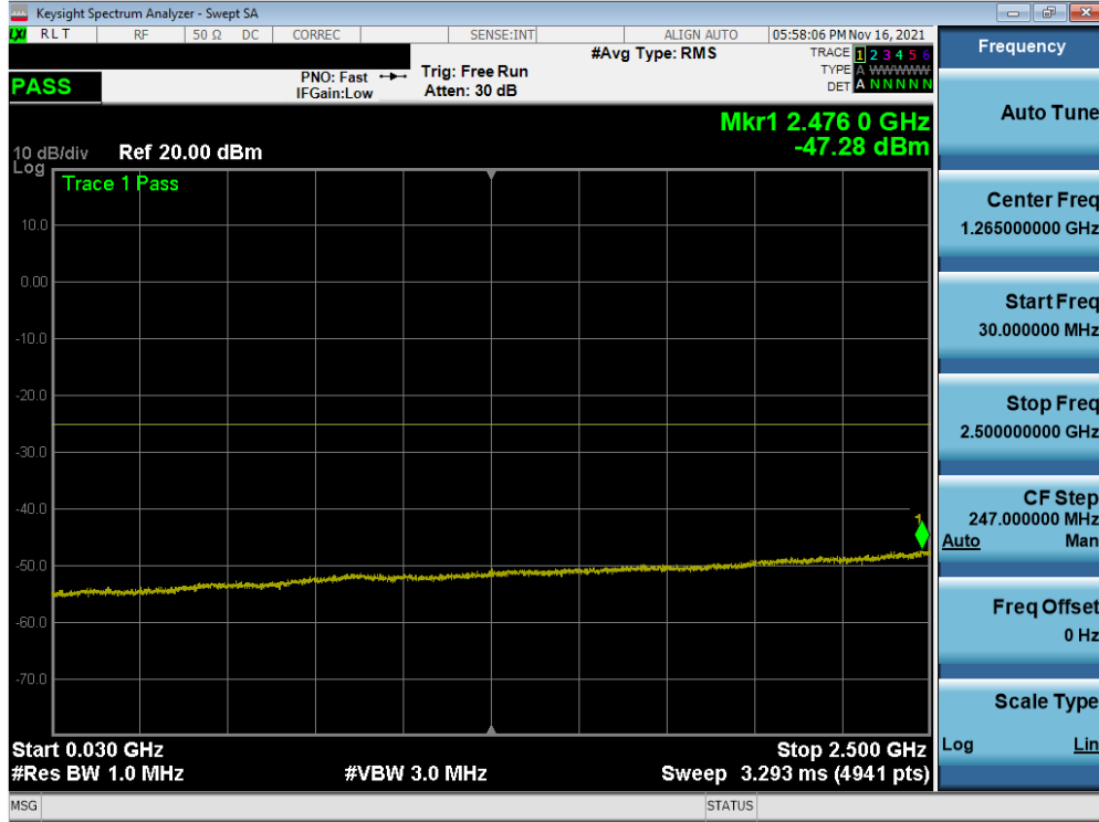
Plot 7-194. Conducted Spurious Plot (ULCA LTE B7 – (20+20)MHz QPSK - RB Size 1, RB Offset 0 - High Channel)
