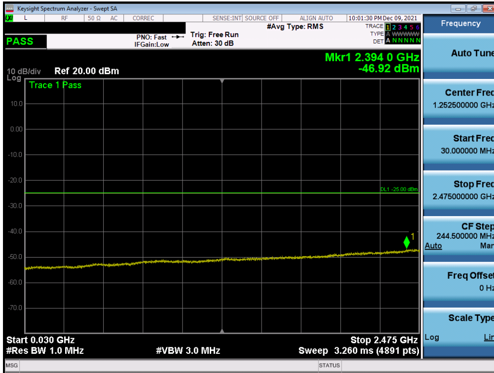
Plot 7-170. Conducted Spurious Plot (NR Band n7 - 40MHz DFT-s-OFDM-QPSK - RB Size 1, RB Offset 0 - Low Channel)
