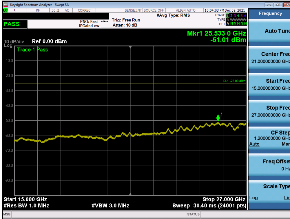
Plot 7-178. Conducted Spurious Plot (NR Band n7 - 40MHz DFT-s-OFDM-QPSK - RB Size 1, RB Offset 0 - High Channel)
