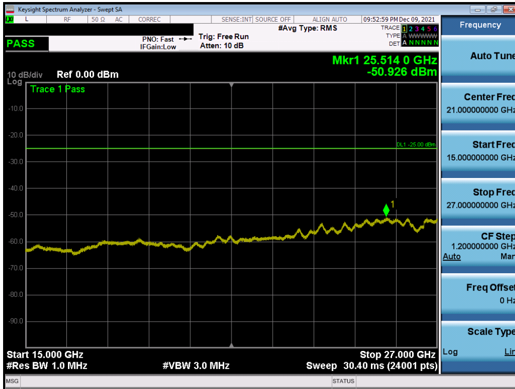
Plot 7-175. Conducted Spurious Plot (NR Band n7 - 40MHz DFT-s-OFDM-QPSK - RB Size 1, RB Offset 0 - Mid Channel)
