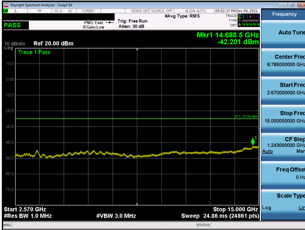
Plot 7-174. Conducted Spurious Plot (NR Band n7 - 40MHz DFT-s-OFDM-QPSK - RB Size 1, RB Offset 0 - Mid Channel)
