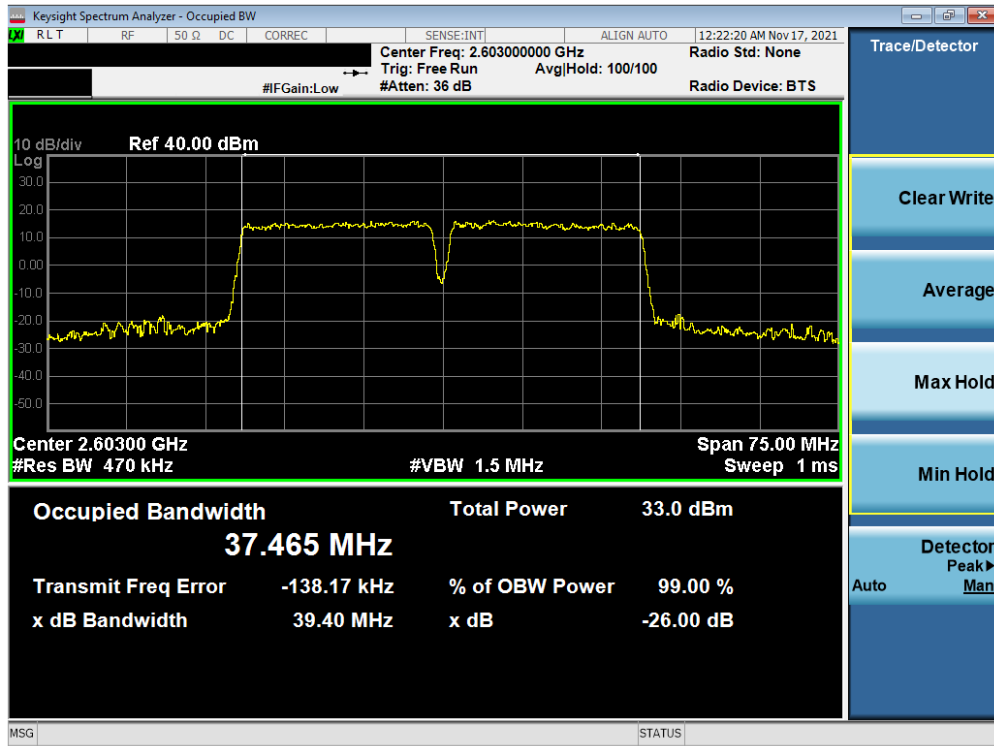
Plot 7-132. Occupied Bandwidth Plot (LTE Band 41 - (20+20)MHz 64-QAM - Full RB)
