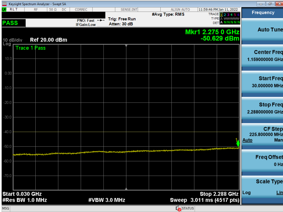
Plot 7-161. Conducted Spurious Plot (NR Band n30 - 5MHz DFT-s-OFDM-QPSK - RB Size 1, RB Offset 0 – Low Channel)
