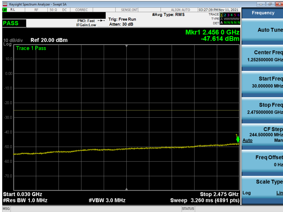
Plot 7-143. Conducted Spurious Plot (LTE Band 7 - 20MHz QPSK - RB Size 1, RB Offset 0 - Low Channel)
