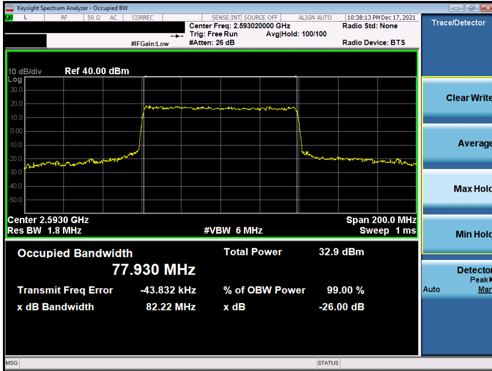
Plot 7-114. Occupied Bandwidth Plot (NR Band n41 - 80MHz CP-OFDM 64-QAM - Full RB)
