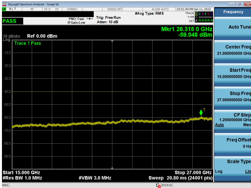
Plot 7-166. Conducted Spurious Plot (NR Band n30 - 10MHz DFT-s-OFDM-QPSK - RB Size 1, RB Offset 0 – Mid Channel)
