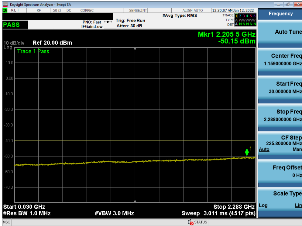
Plot 7-167. Conducted Spurious Plot (NR Band n30 - 5MHz DFT-s-OFDM-QPSK - RB Size 1, RB Offset 0 – High Channel)
