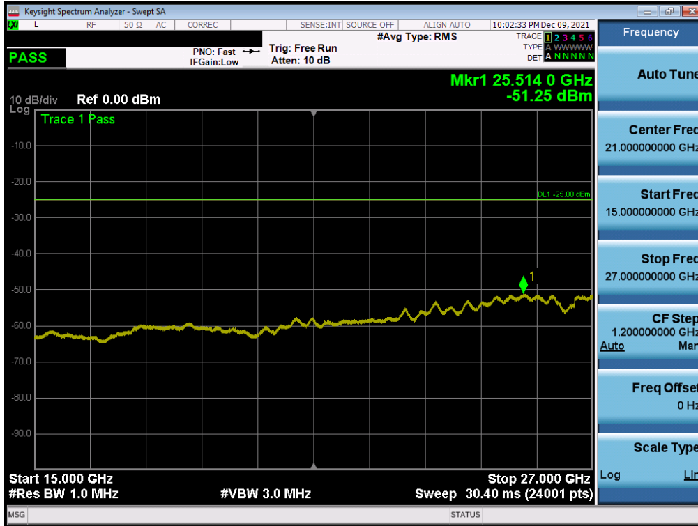
Plot 7-172. Conducted Spurious Plot (NR Band n7 - 40MHz DFT-s-OFDM-QPSK - RB Size 1, RB Offset 0 - Low Channel)
