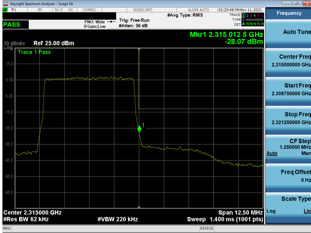
Plot 7-208. Upper Band Edge Plot (LTE Band 30 - 5MHz QPSK – Full RB)
