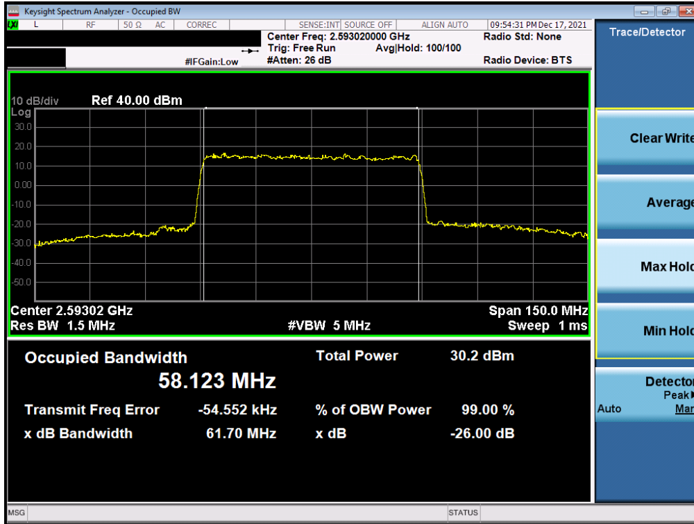
Plot 7-110. Occupied Bandwidth Plot (NR Band n41 - 60MHz DFT-s-OFDM 256-QAM - Full RB)
