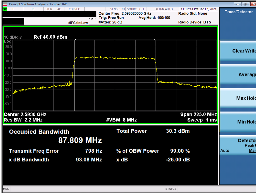
Plot 7-120. Occupied Bandwidth Plot (NR Band n41 - 90MHz CP-OFDM 256-QAM - Full RB)
