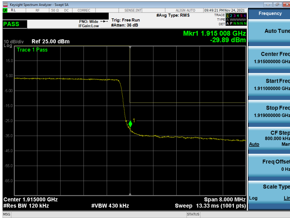
Plot 7-142. Upper Band Edge Plot (NR Band n25 – 10MHz DFT-s-OFDM \pi/2 BPSK – Full RB Configuration)
