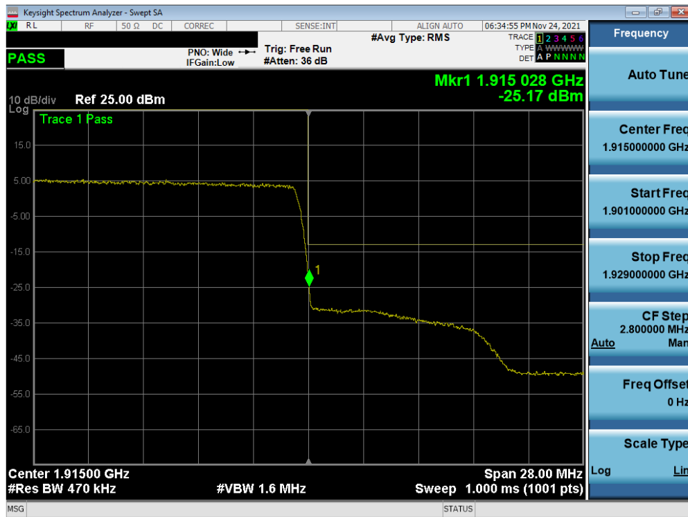
Plot 7-162. Upper Band Edge Plot (NR Band n25 – 40MHz DFT-s-OFDM QPSK – Full RB Configuration)
