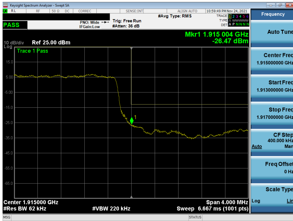
Plot 7-138. Upper Band Edge Plot (NR Band n25 – 5MHz DFT-s-OFDM \pi/2 BPSK – Full RB Configuration)
