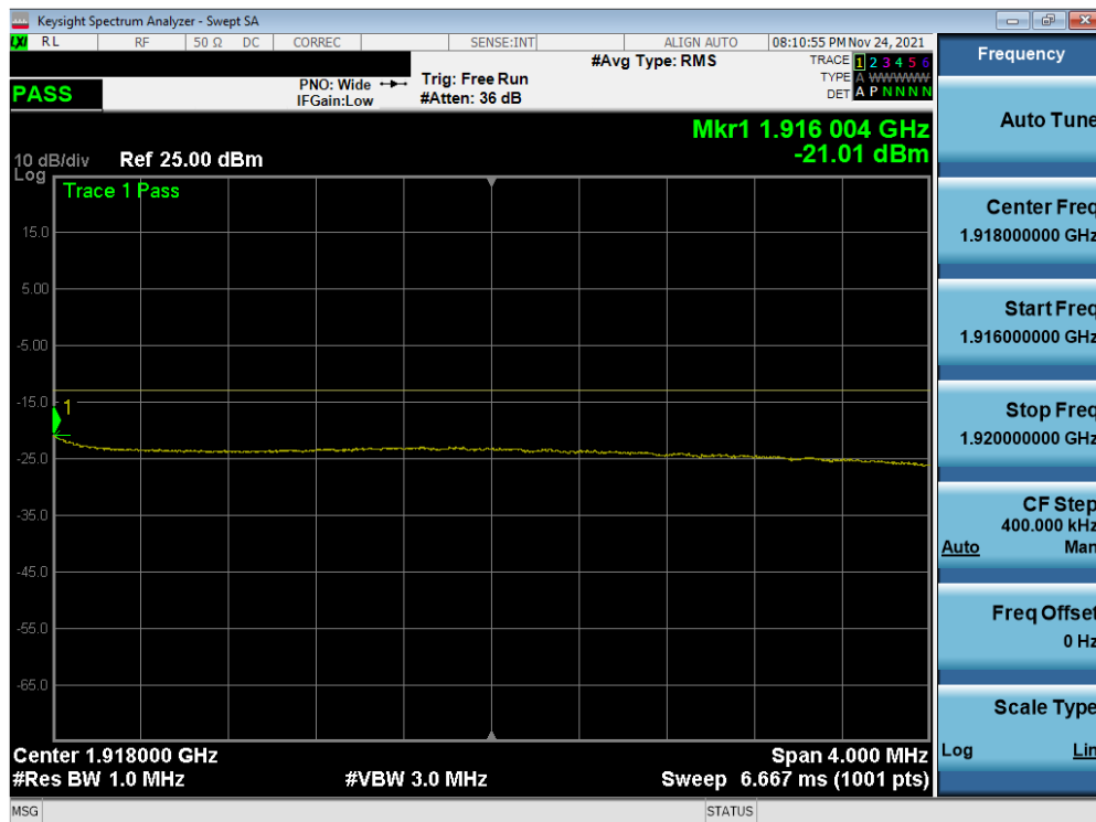
Plot 7-147. Extended Upper Band Edge Plot (NR Band n25 – 15MHz DFT-s-OFDM QPSK – Full RB Configuration)
