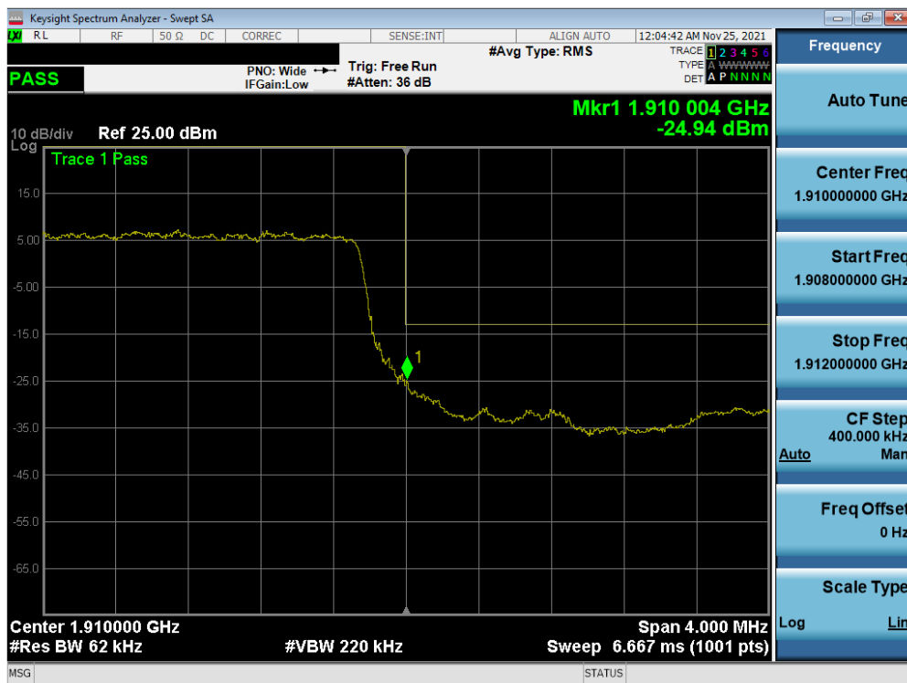
Plot 7-166. Upper Band Edge Plot (NR Band n2 – 5MHz DFT-s-OFDM \pi/2 BPSK – Full RB Configuration)
