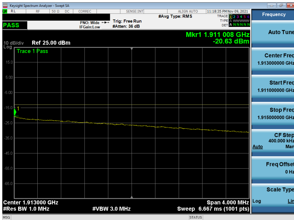
Plot 7-127. Extended Upper Band Edge Plot (LTE Band 2 – 10MHz QPSK – Full RB Configuration)
