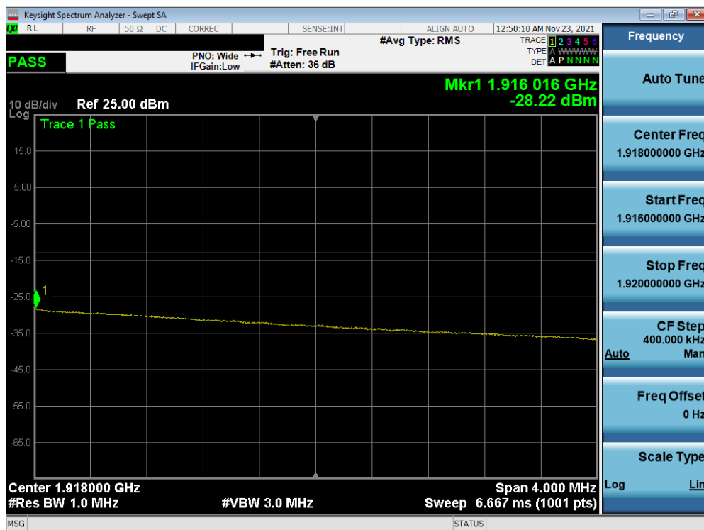
Plot 7-159. Extended Upper Band Edge Plot (NR Band n25 – 30MHz DFT-s-OFDM \pi/2 BPSK – Full RB Configuration)
