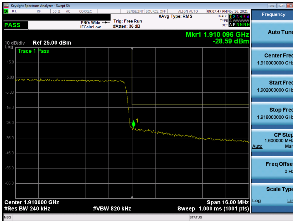
Plot 7-178. Upper Band Edge Plot (NR Band n2 – 20MHz CP-OFDM QPSK – Full RB Configuration)
