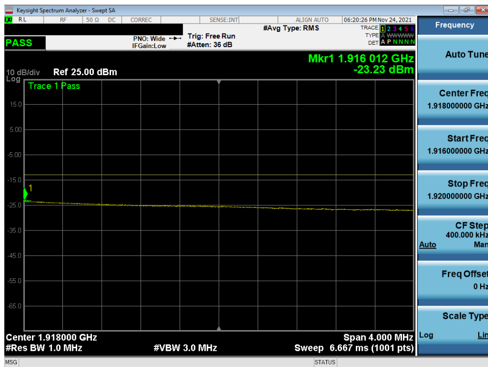
Plot 7-155. Extended Upper Band Edge Plot (NR Band n25 – 25MHz DFT-s-OFDM QPSK – Full RB Configuration)
