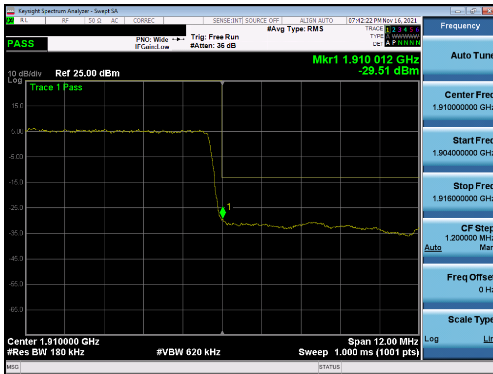
Plot 7-174. Upper Band Edge Plot (NR Band n2 – 15MHz DFT-s-OFDM QPSK – Full RB Configuration)
