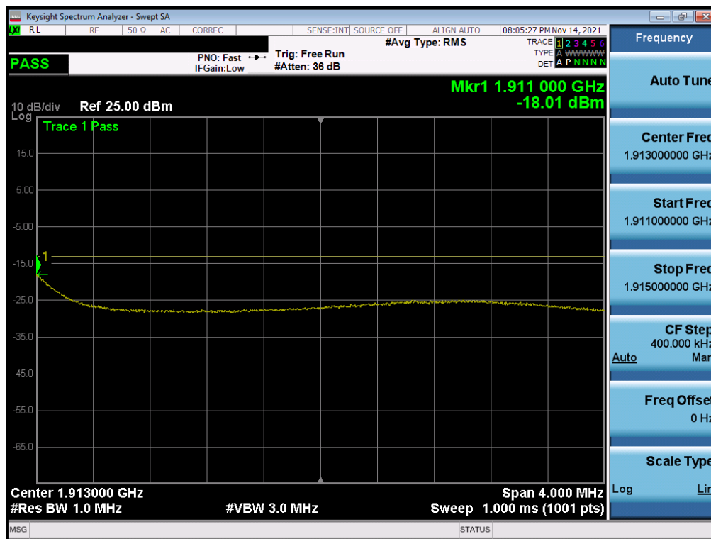
Plot 7-171. Extended Upper Band Edge Plot (NR Band n2 – 10MHz DFT-s-OFDM \pi/2 BPSK – Full RB Configuration)
