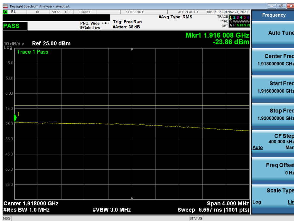
Plot 7-163. Extended Upper Band Edge Plot (NR Band n25 – 40MHz DFT-s-OFDM \pi/2 BPSK – Full RB Configuration)
