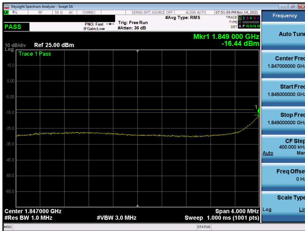
Plot 7-169. Extended Lower Band Edge Plot (NR Band n2 – 10MHz DFT-s-OFDM \pi/2 BPSK – Full RB Configuration)
