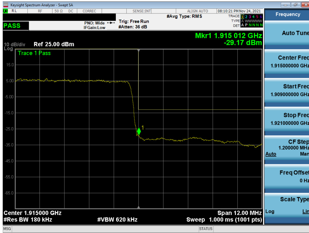
Plot 7-146. Upper Band Edge Plot (NR Band n25 – 15MHz DFT-s-OFDM QPSK – Full RB Configuration)
