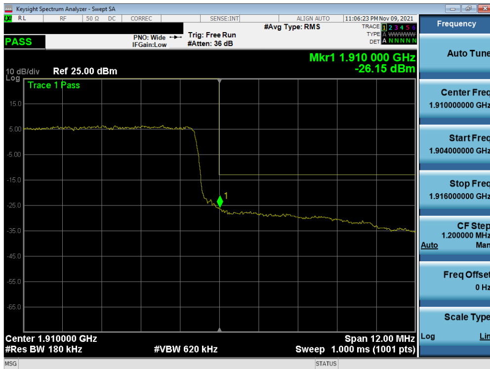
Plot 7-130. Upper Band Edge Plot (LTE Band 2 – 15MHz QPSK – Full RB Configuration)
