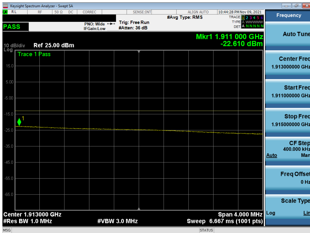
Plot 7-135. Extended Upper Band Edge Plot (LTE Band 2 – 20MHz QPSK – Full RB Configuration)
