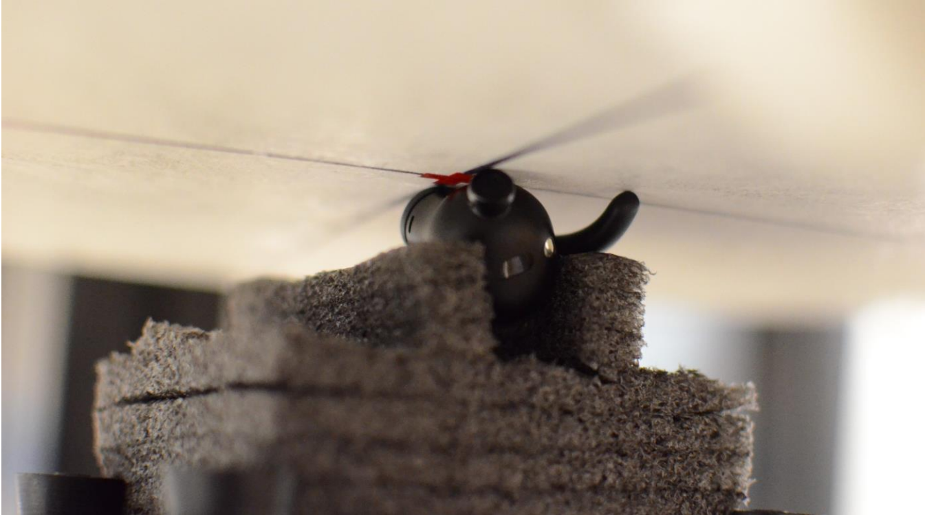
SAR Test Setup Photo 1: Head, Left Earbud, 0 mm
