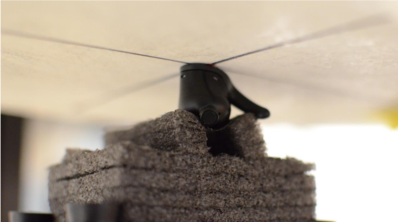
SAR Test Setup Photo 2: Body-Worn, Back Side, 0 mm
