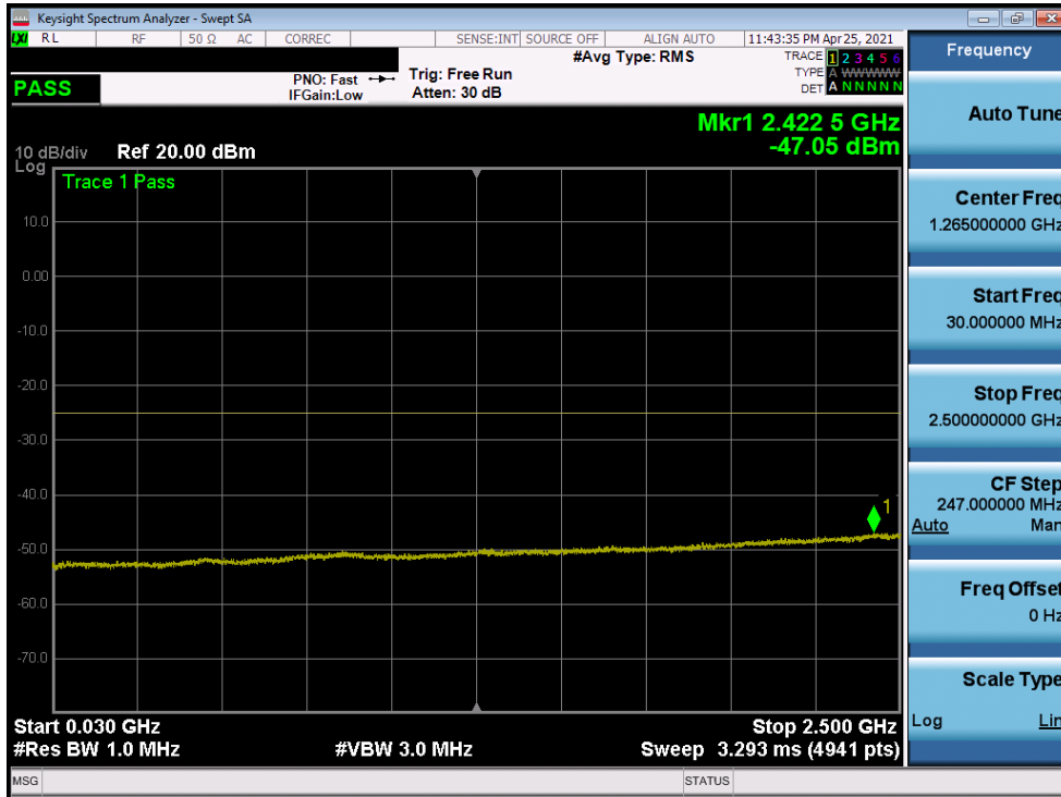
Plot 7-149. Conducted Spurious Plot (LTE Band 7 - 20MHz QPSK - RB Size 1, RB Offset 0 - High Channel)
