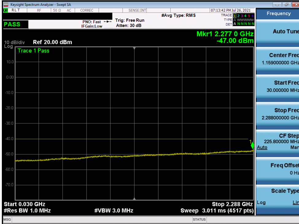
Plot 7-140. Conducted Spurious Plot (LTE Band 30 - 5MHz QPSK - RB Size 1, RB Offset 0 – High Channel)
