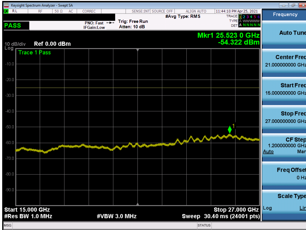
Plot 7-151. Conducted Spurious Plot (LTE Band 7 - 20MHz QPSK - RB Size 1, RB Offset 0 - High Channel)
