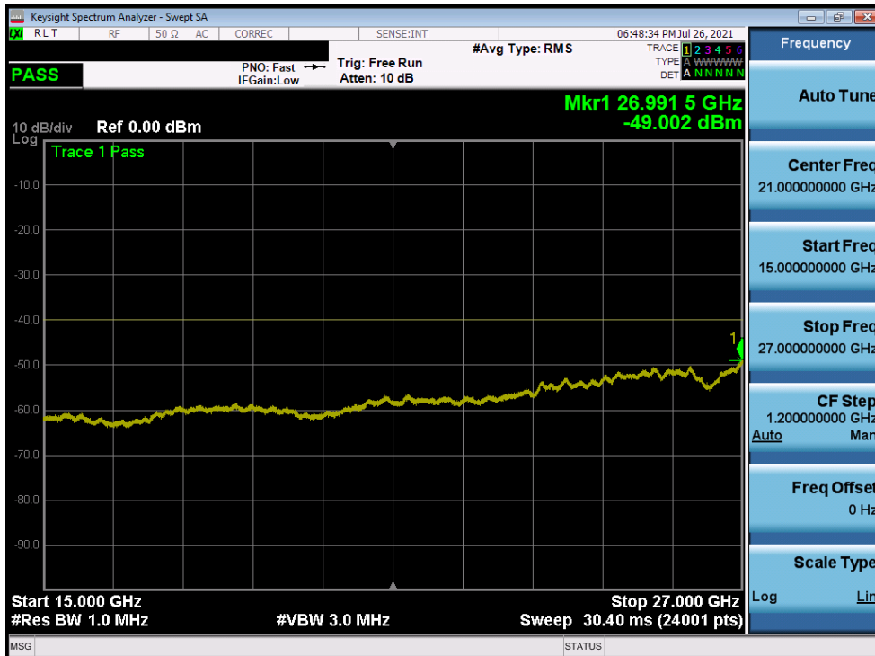
Plot 7-139. Conducted Spurious Plot (LTE Band 30 - 10MHz QPSK - RB Size 1, RB Offset 0 – Mid Channel)
