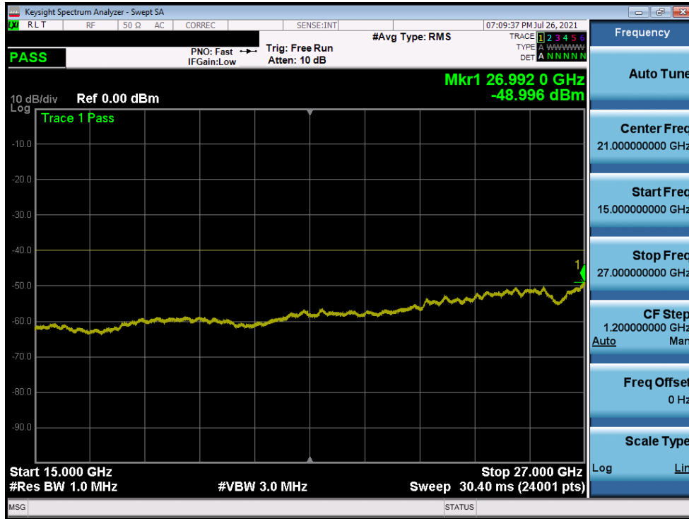
Plot 7-136. Conducted Spurious Plot (LTE Band 30 - 5MHz QPSK - RB Size 1, RB Offset 0 – Low Channel)
