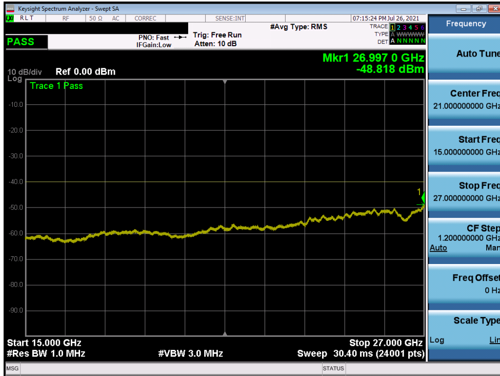
Plot 7-142. Conducted Spurious Plot (LTE Band 30 - 5MHz QPSK - RB Size 1, RB Offset 0 – High Channel)
