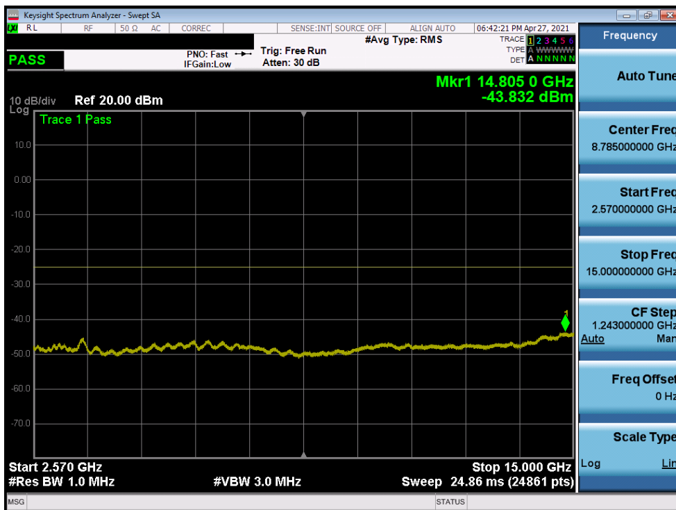
Plot 7-189. Conducted Spurious Plot (ULCA LTE B7 - (20+20)MHz QPSK - RB Size 1, RB Offset 0 - Low Channel)
