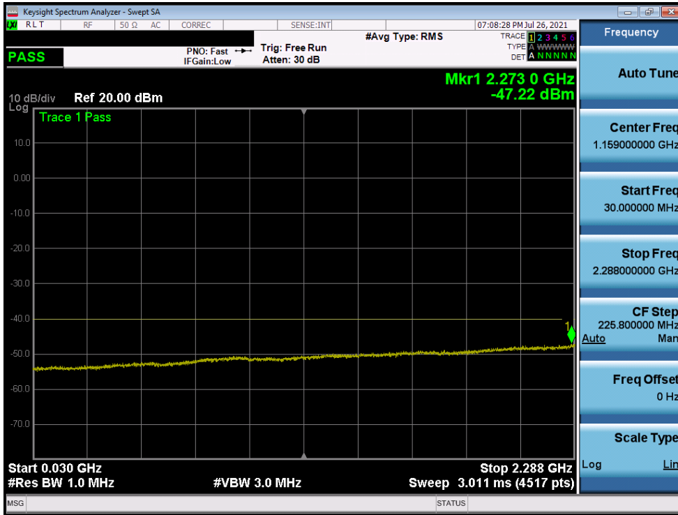
Plot 7-134. Conducted Spurious Plot (LTE Band 30 - 5MHz QPSK - RB Size 1, RB Offset 0 – Low Channel)
