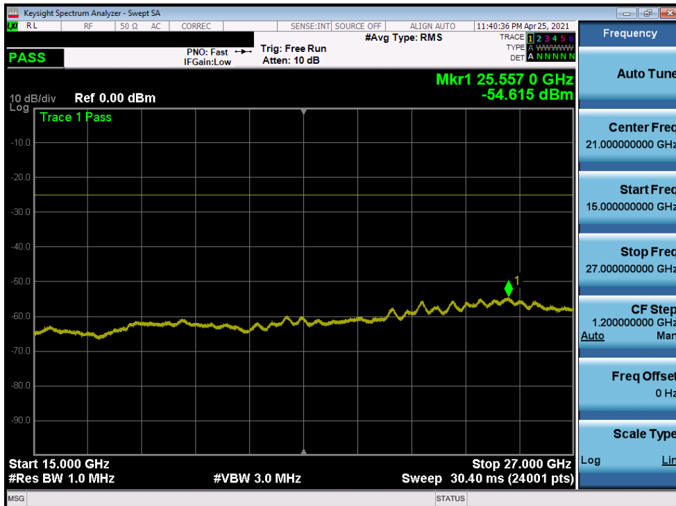
Plot 7-148. Conducted Spurious Plot (LTE Band 7 - 20MHz QPSK - RB Size 1, RB Offset 0 - Mid Channel)
