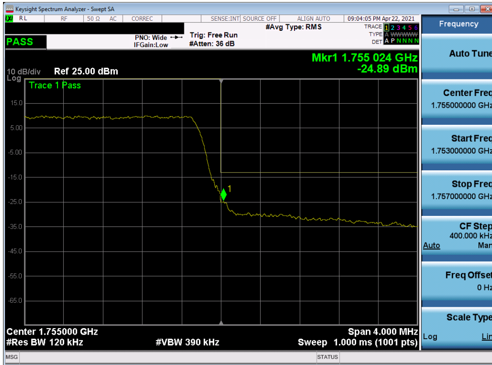
Plot 7-220. Upper Band Edge Plot (LTE Band 4 - 5MHz QPSK – Full RB)
