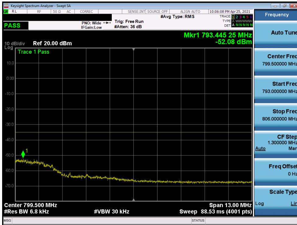
Plot 7-281. Upper Emission Mask Plot (LTE Band 13 - 5MHz QPSK – Full RB)
