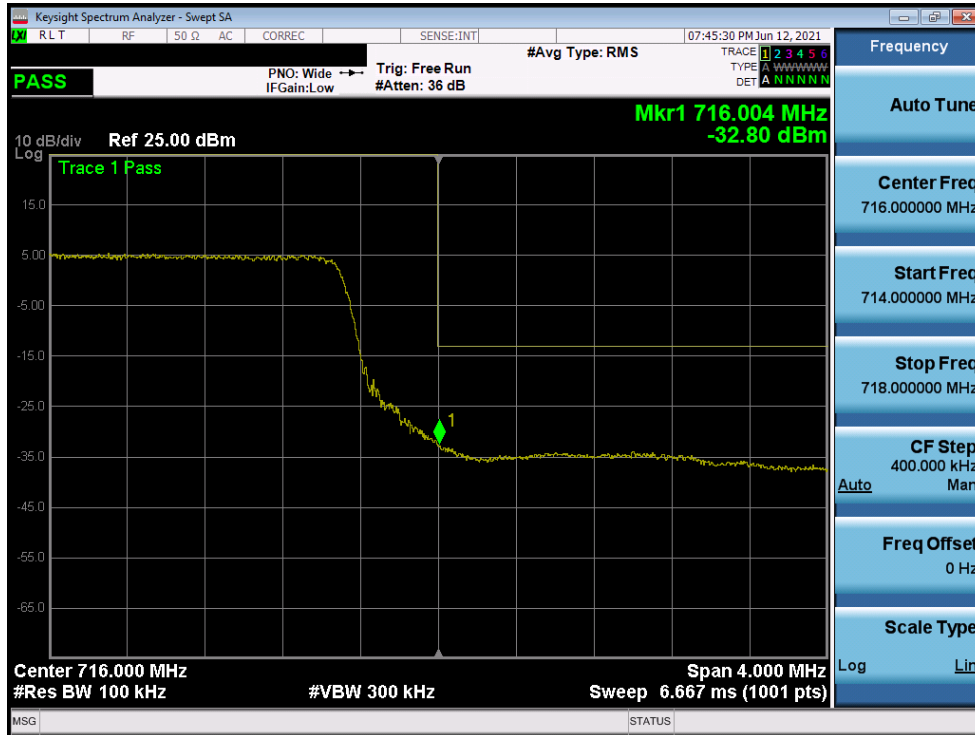
Plot 7-277. Upper Band Edge Plot (LTE Band 17 - 10MHz QPSK – Full RB)
