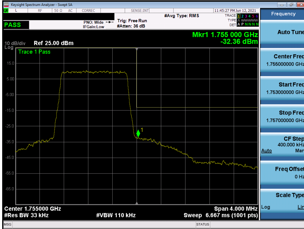
Plot 7-212. Upper Band Edge Plot (LTE Band 4 – 1.4MHz QPSK – Full RB)
