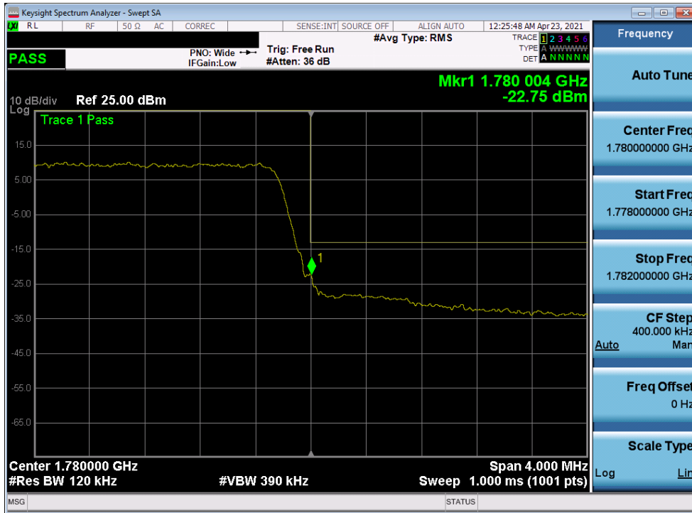
Plot 7-244. Upper Band Edge Plot (LTE Band 66 - 5MHz QPSK – Full RB)
