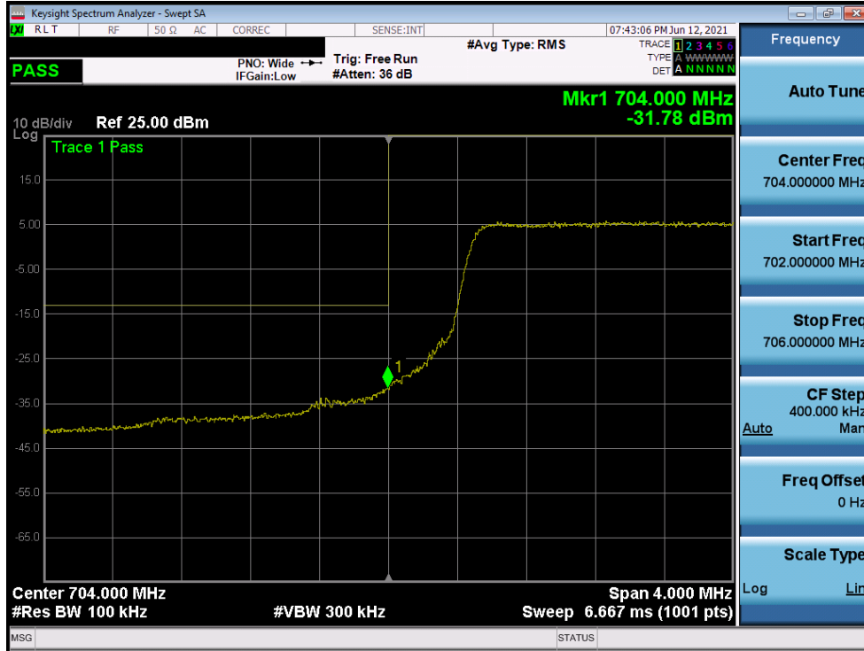
Plot 7-276. Lower Band Edge Plot (LTE Band 17 - 10MHz QPSK – Full RB)
