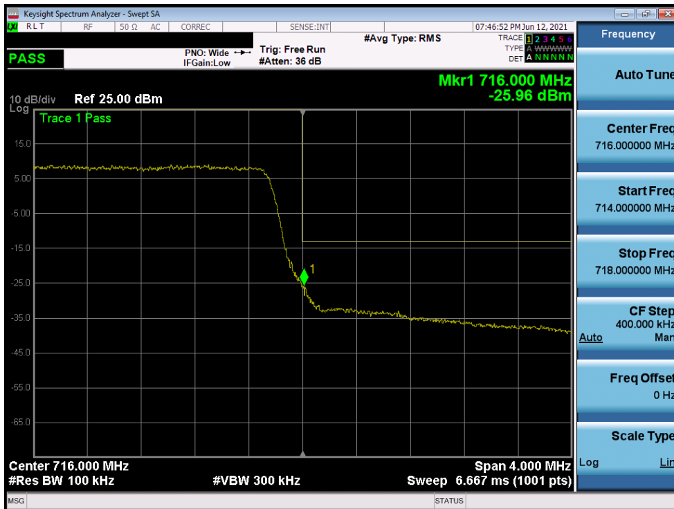
Plot 7-275. Upper Band Edge Plot (LTE Band 17 - 5MHz QPSK – Full RB)
