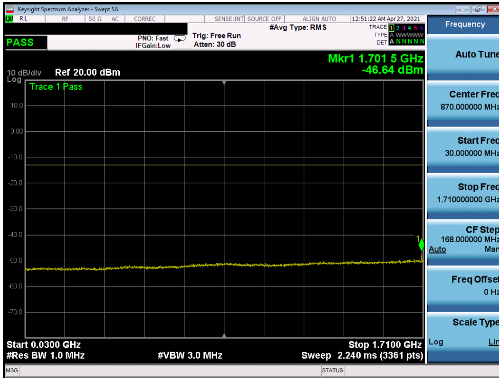
Plot 7-207. Conducted Spurious Plot (ULCA LTE Band 66 – (20+20)MHz QPSK – High Channel)
