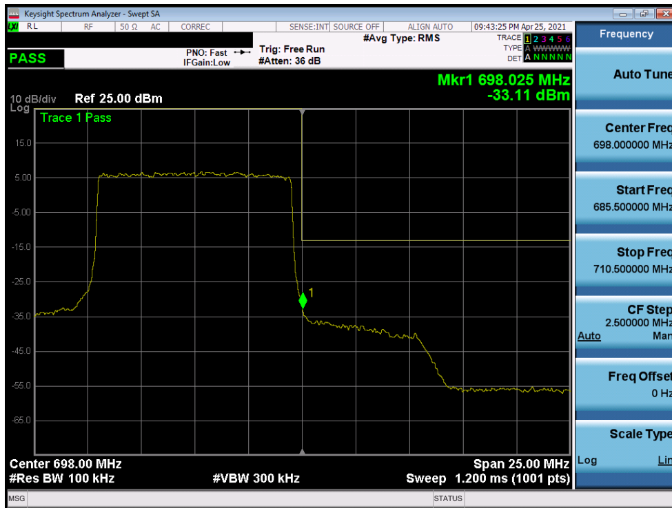
Plot 7-261. Upper Band Edge Plot (LTE Band 71 - 10MHz QPSK – Full RB)
