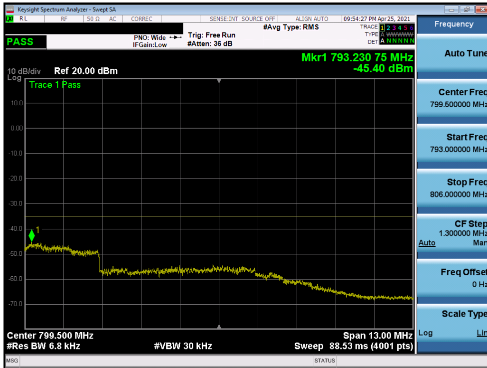
Plot 7-285. Upper Emission Mask Plot (LTE Band 13 - 10MHz QPSK – Full RB)
