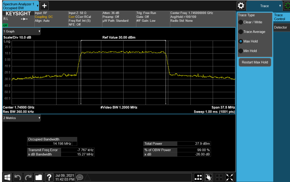
Plot 7-79. Occupied Bandwidth Plot (NR Band n66 - 15.0MHz CP-OFDM 256QAM - Full RB)
