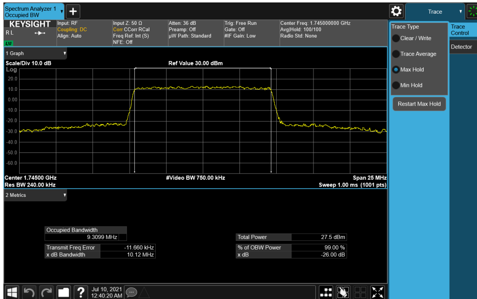
Plot 7-74. Occupied Bandwidth Plot (NR Band n66 - 10.0MHz CP-OFDM 256QAM - Full RB)
