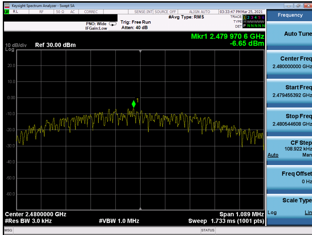
Plot 7-9. Power Spectral Density (Bluetooth (LE), 1Mbps,- Ch. 39)
