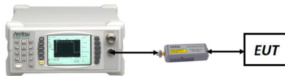
Figure 7-2. Test Instrument & Measurement Setup for Peak and Average Power Measurement
