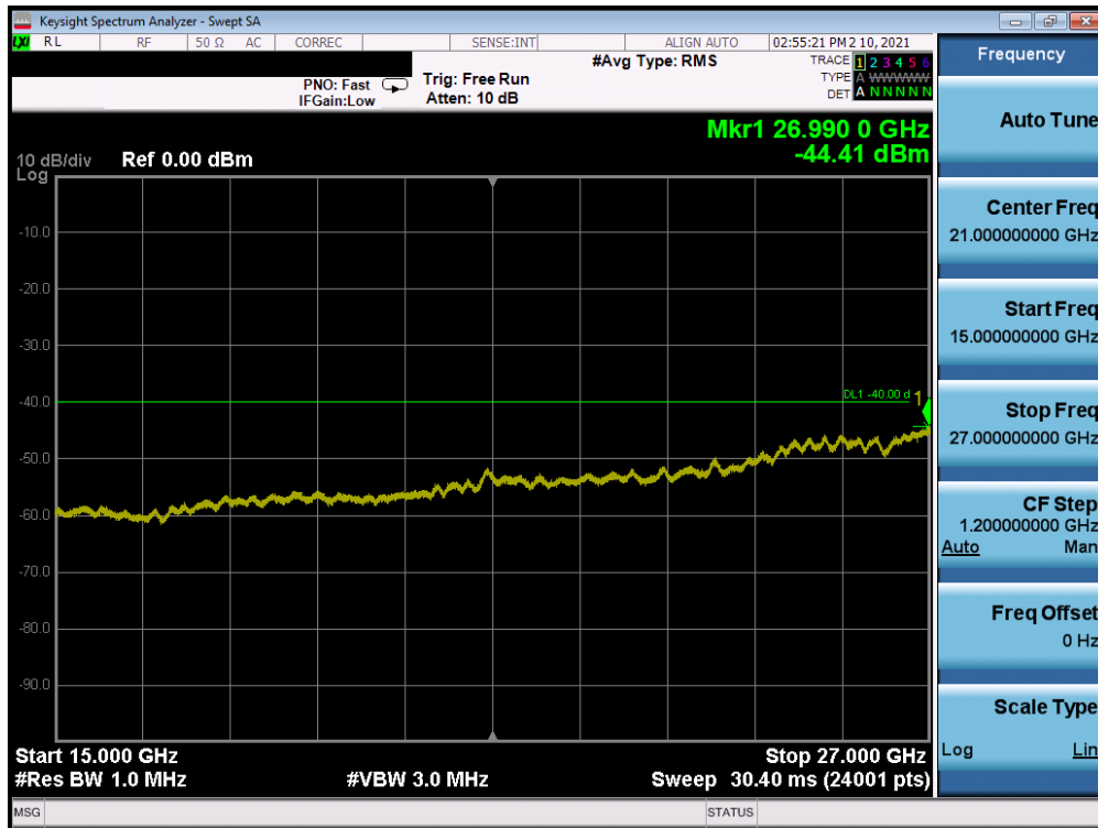
Plot 7-35. Conducted Spurious Plot (LTE Band 48 - 20MHz QPSK - RB Size 1, RB Offset 0 - Low Channel)
