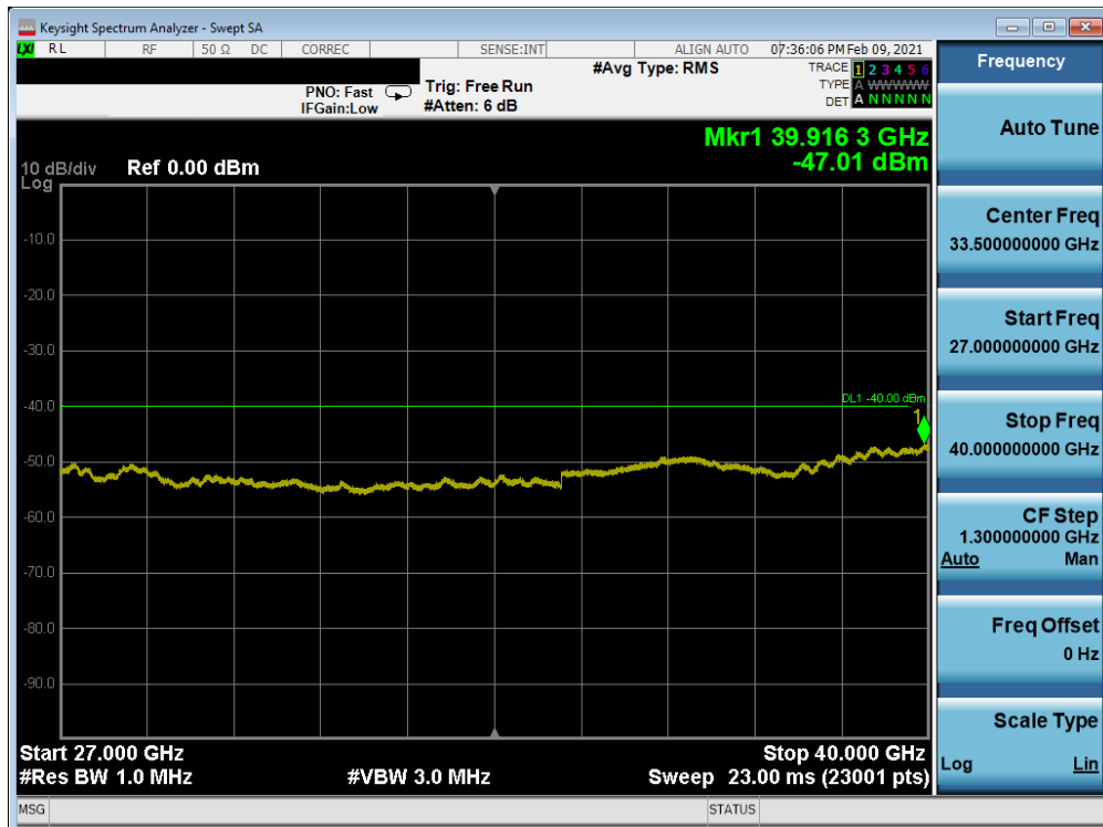
Plot 7-40. Conducted Spurious Plot (LTE Band 48 - 20MHz QPSK - RB Size 1, RB Offset 0 - Mid Channel)
