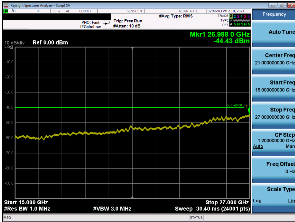
Plot 7-39. Conducted Spurious Plot (LTE Band 48 - 20MHz QPSK - RB Size 1, RB Offset 0 - Mid Channel)
