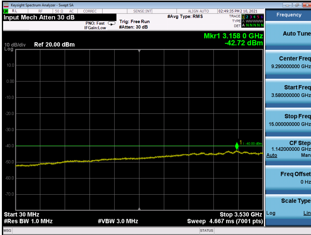
Plot 7-33. Conducted Spurious Plot (LTE Band 48 - 20MHz QPSK - RB Size 1, RB Offset 0 - Low Channel)
