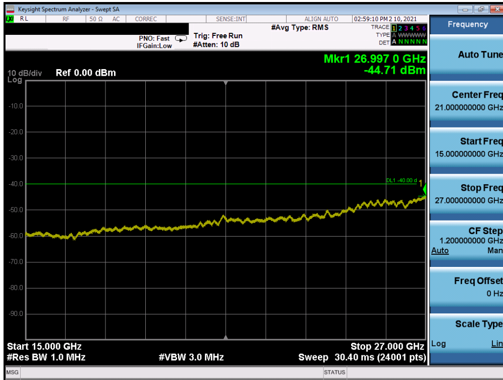
Plot 7-43. Conducted Spurious Plot (LTE Band 48 - 20MHz QPSK - RB Size 1, RB Offset 0 - High Channel)
