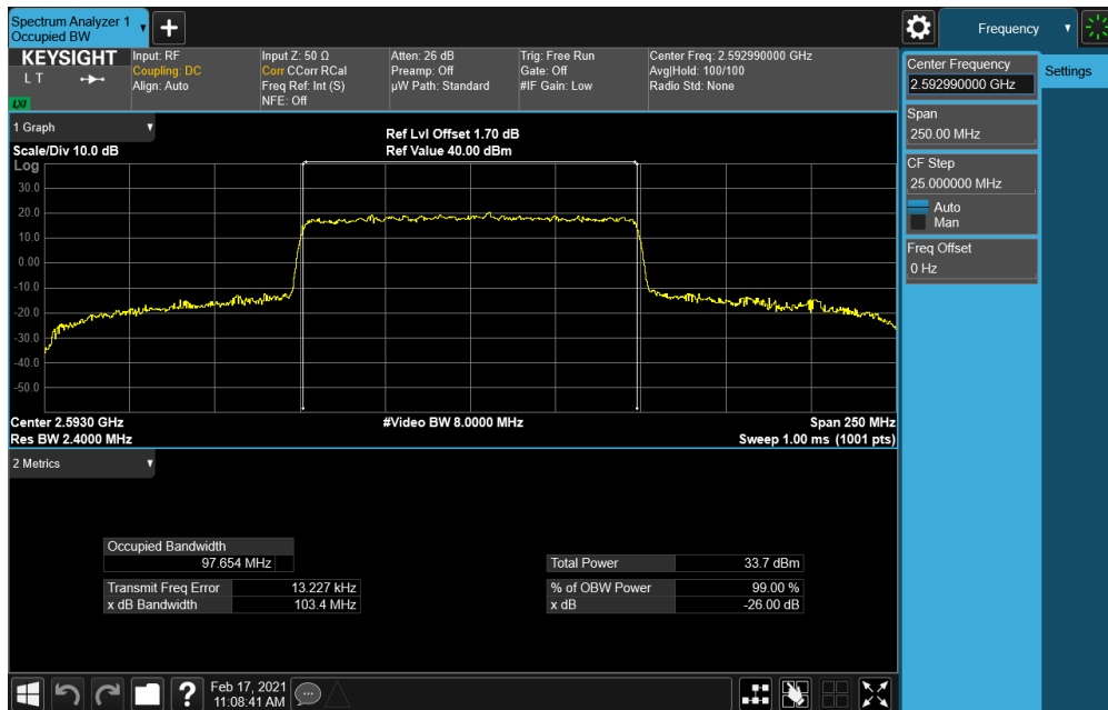
Plot 7-44. Occupied Bandwidth Plot (NR Band n41 - 100MHz CP-OFDM 64-QAM - Full RB Configuration)
