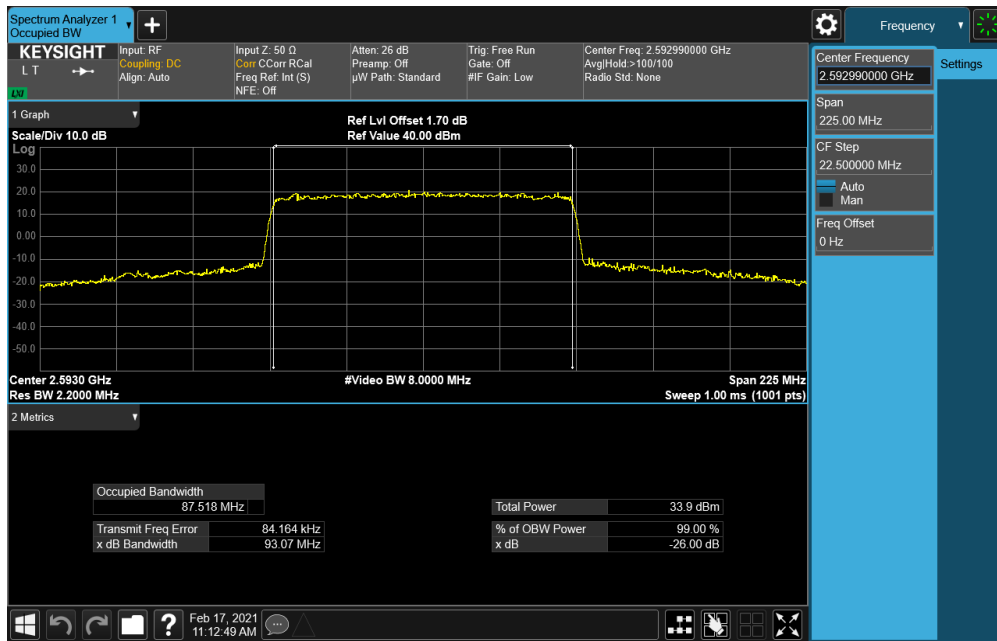
Plot 7-48. Occupied Bandwidth Plot (NR Band n41 - 90MHz CP-OFDM 16-QAM - Full RB Configuration)
