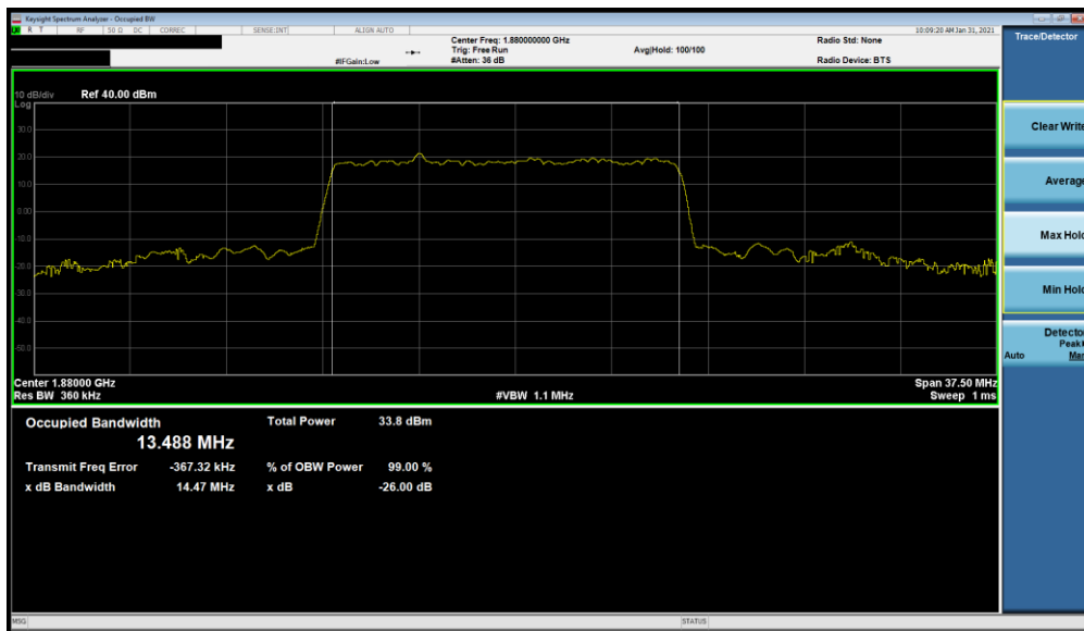
Plot 7-30. Occupied Bandwidth Plot (NR Band n25/n2 - 15.0MHz DFT-s-OFDM \pi/2 BPSK - Full RB)
