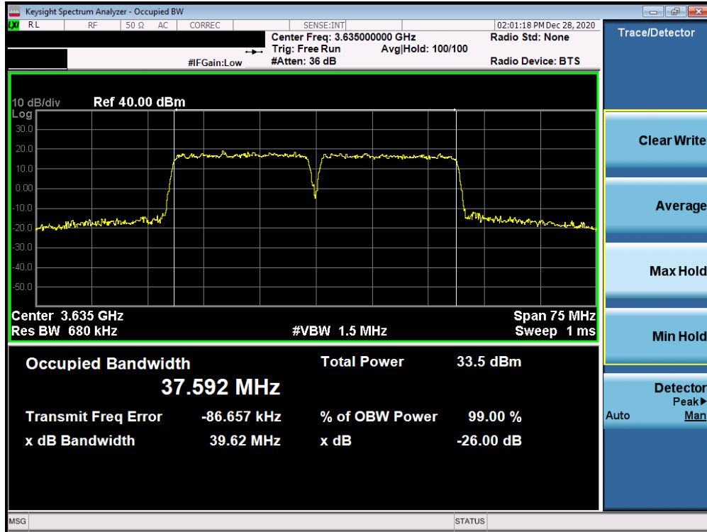
Plot 7-19. Occupied Bandwidth Plot (ULCA LTE Band 48 – 20+20MHz 64-QAM - Full RB Configuration)
