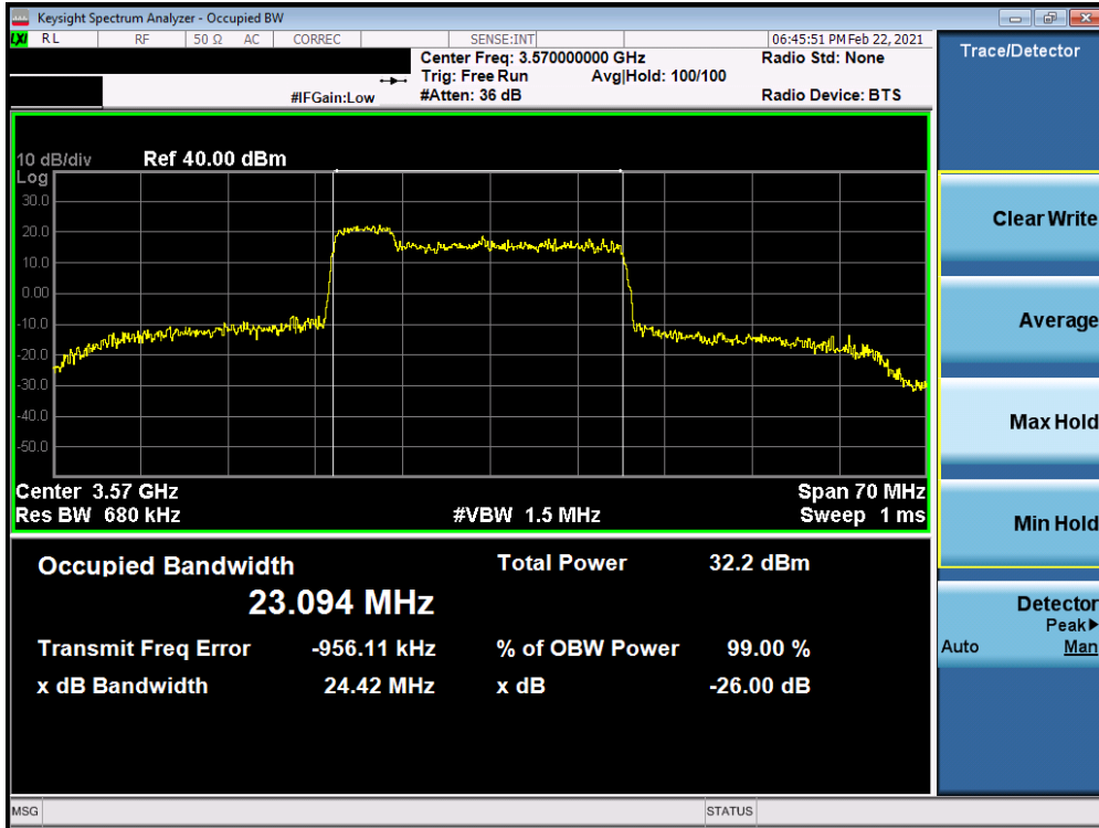
Plot 7-29. Occupied Bandwidth Plot (ULCA LTE Band 48 – 20+5MHz QPSK - Full RB Configuration)
