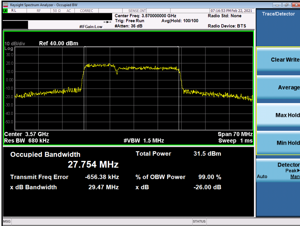
Plot 7-27. Occupied Bandwidth Plot (ULCA LTE Band 48 – 20+10MHz 64-QAM - Full RB Configuration)
