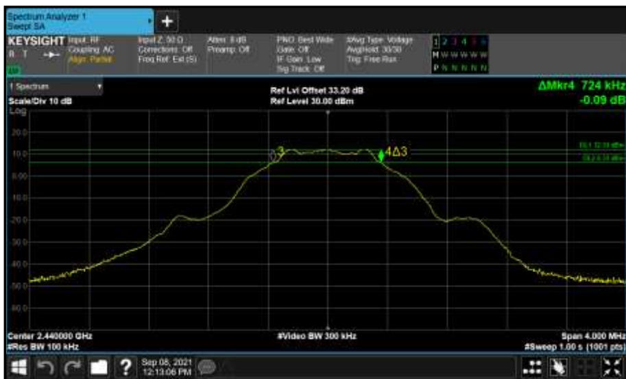
Figure 96 - Core 1 (B) 2440 MHz (CH17) 6 dB Bandwidth
