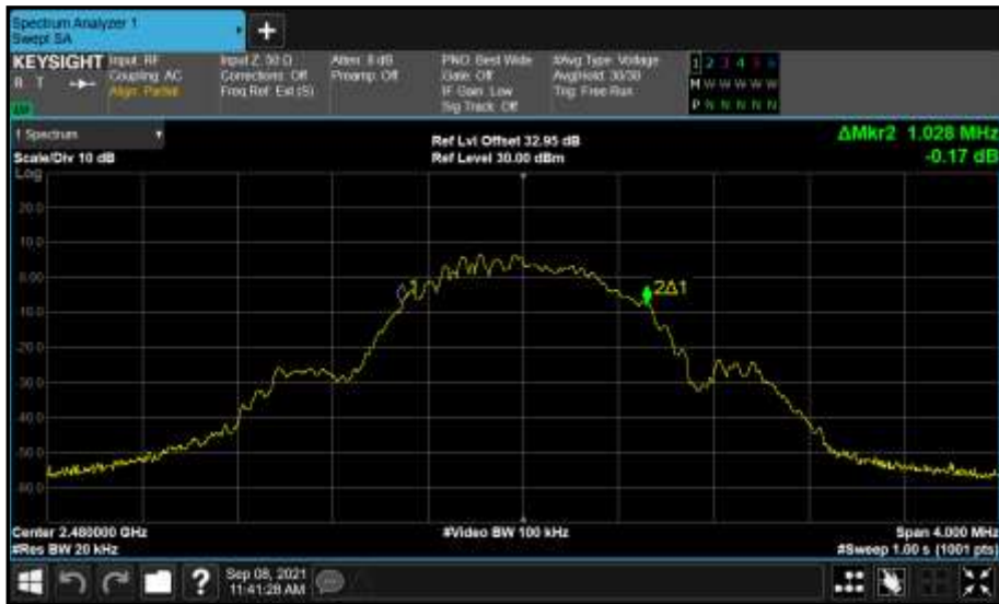
Figure 192 - Core 0 (A) 2480 MHz (CH39) 99% Bandwidth
