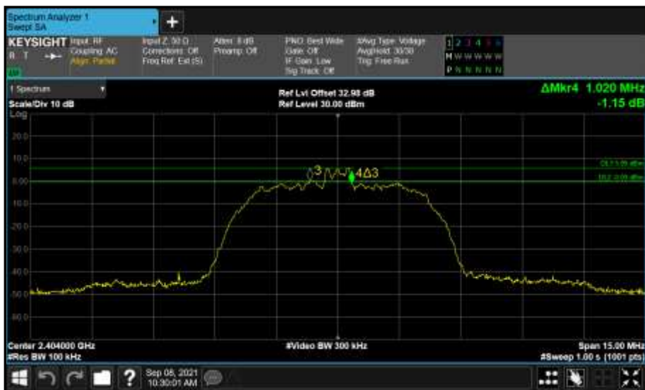
Figure 149 - Core 0 (A) 2404 MHz (CH2) 6 dB Bandwidth
