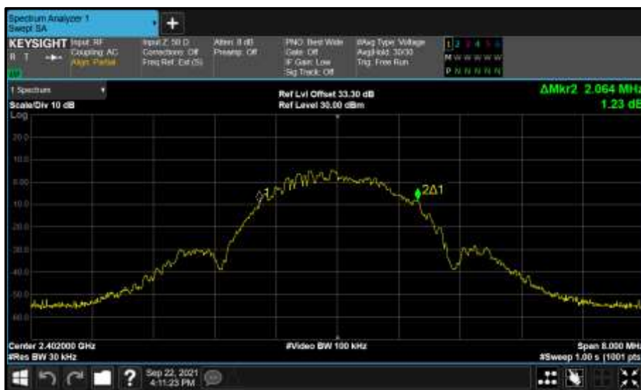
Figure 198 - Core 1 (B) 2402 MHz (CH37) 99% Bandwidth
