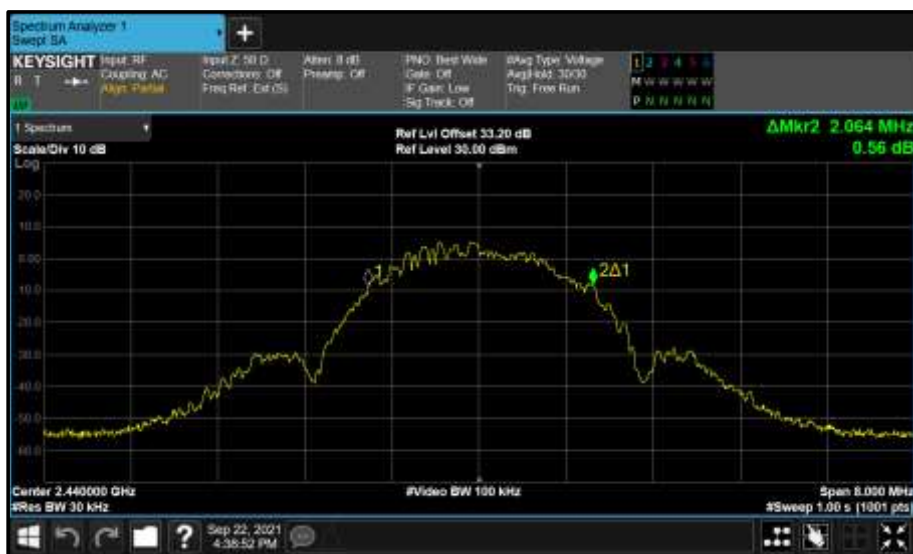
Figure 107 - Core 1 (B) 2440 MHz (CH17) 99% Bandwidth
