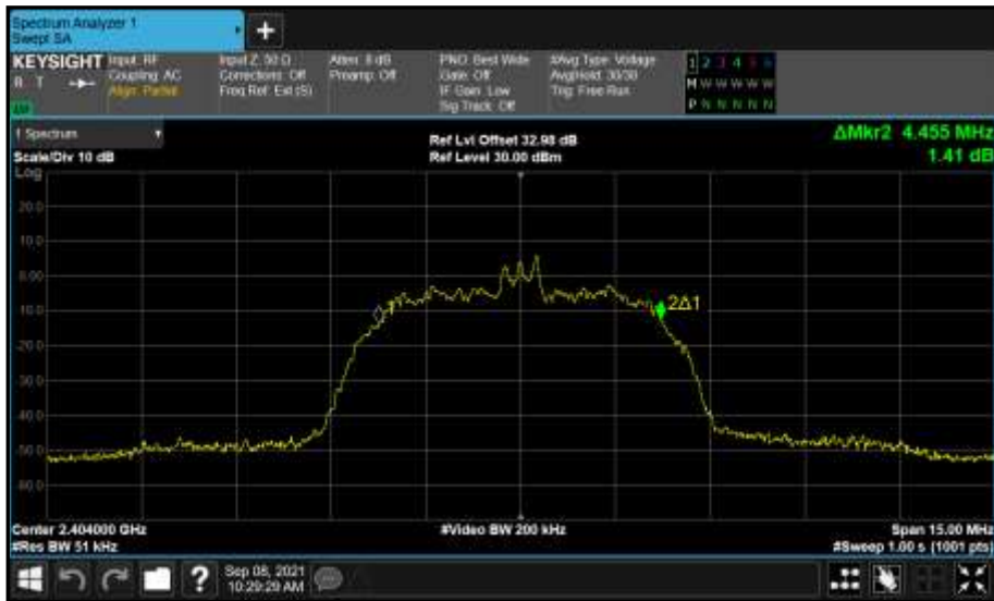
Figure 148 - Core 0 (A) 2404 MHz (CH2) 99% Bandwidth
