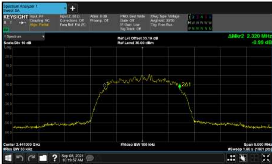
Figure 142 - Core 1 (B) 2441 MHz (CH39) 99% Bandwidth
