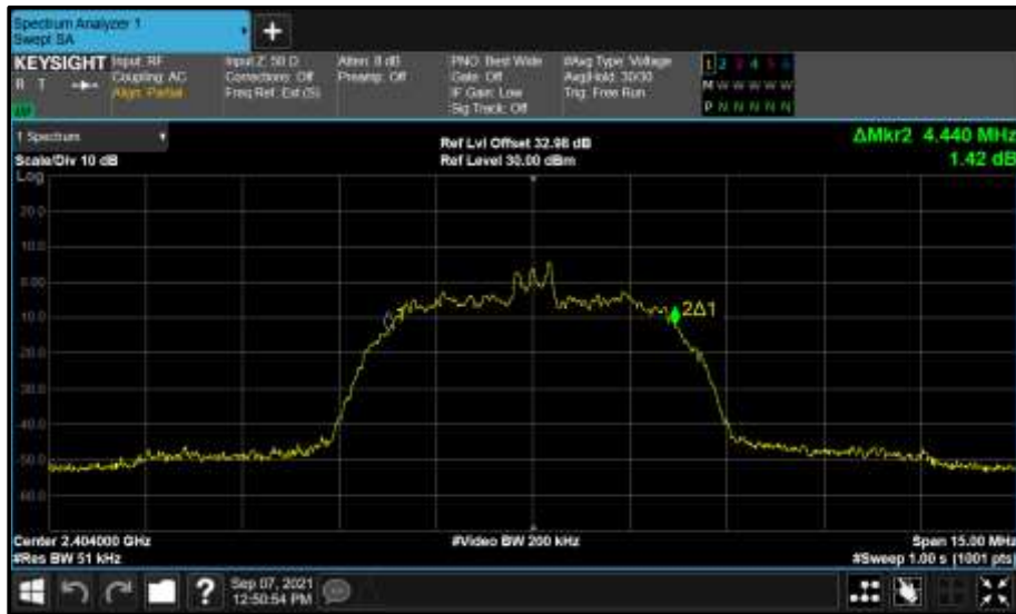
Figure 118 - Core 0 (A) 2404 MHz (CH2) 99% Bandwidth
