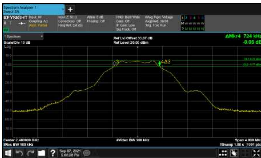
Figure 177 - Core 2 (C) 2480 MHz (CH39) 6 dB Bandwidth
