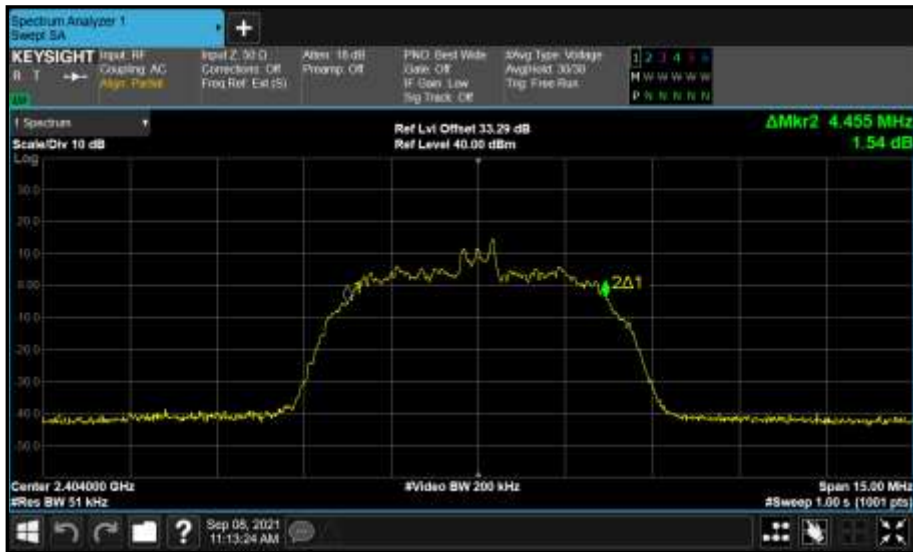
Figure 67 - Core 1 (B) 2404 MHz (CH2) 99% Bandwidth
