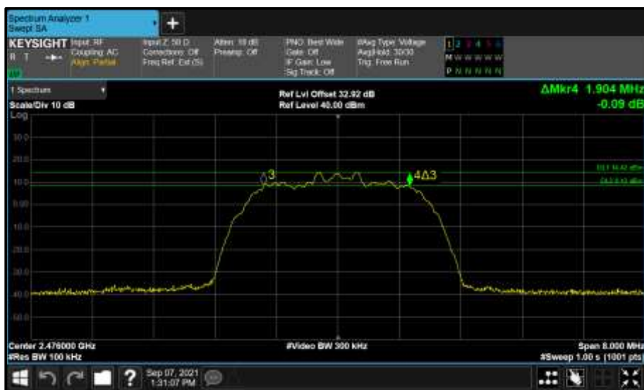
Figure 46 - Core 0 (A) 2476 MHz (CH74) 6 dB Bandwidth
