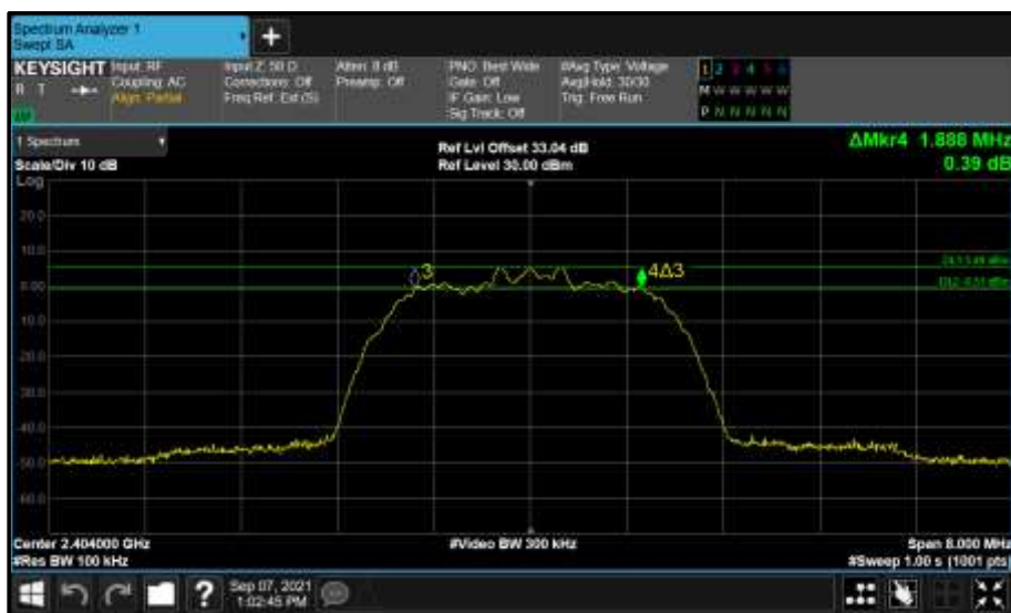
Figure 125 - Core 2 (C) 2404 MHz (CH2) 6 dB Bandwidth
