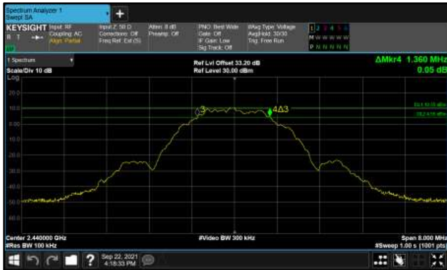
Figure 203 - Core 1 (B) 2440 MHz (CH17) 6 dB Bandwidth
