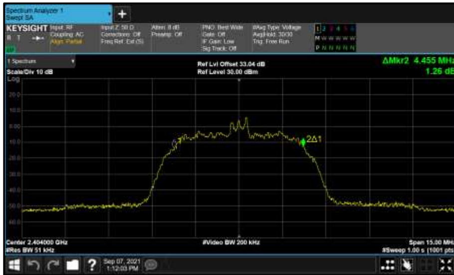
Figure 130 - Core 2 (C) 2404 MHz (CH2) 99% Bandwidth
