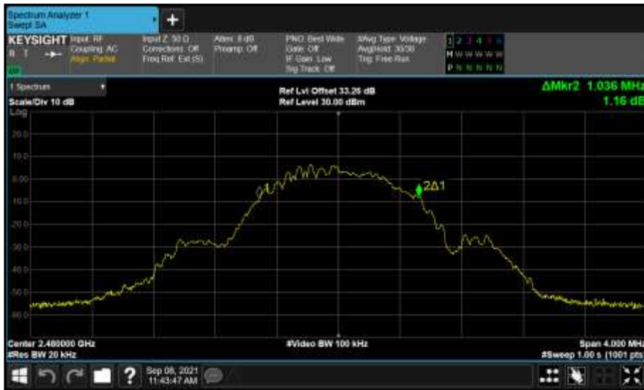
Figure 194 - Core 1 (B) 2480 MHz (CH39) 99% Bandwidth
