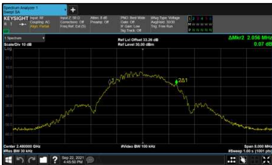
Figure 111 - Core 1 (B) 2480 MHz (CH39) 99% Bandwidth
