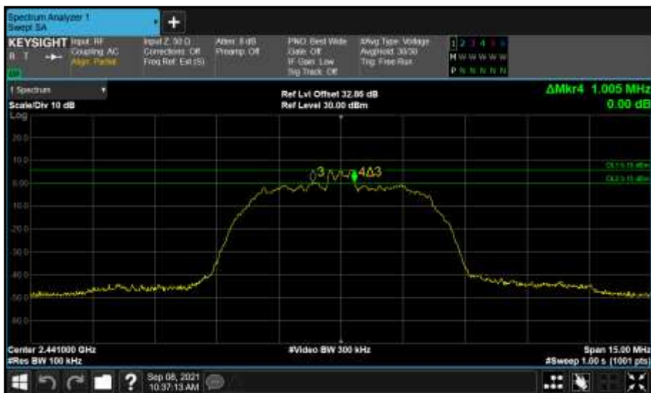
Figure 153 - Core 0 (A) 2441 MHz (CH39) 6 dB Bandwidth
