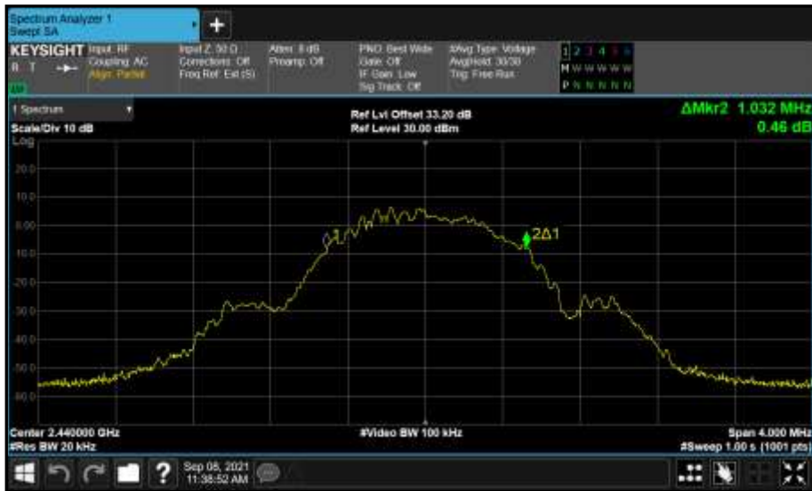
Figure 190 - Core 1 (B) 2440 MHz (CH17) 99% Bandwidth
