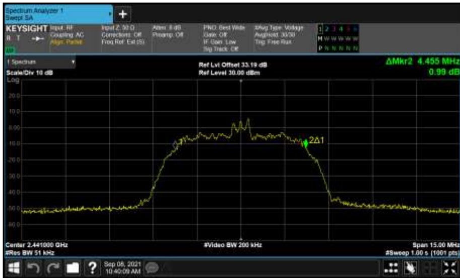
Figure 154 - Core 1 (B) 2441 MHz (CH39) 99% Bandwidth
