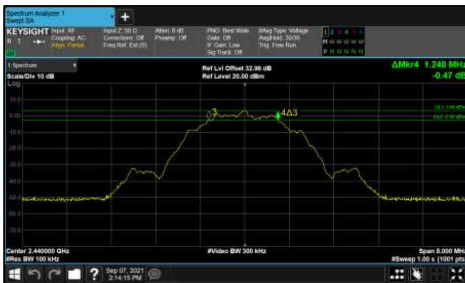
Figure 181 - Core 2 (C) 2440 MHz (CH17) 6 dB Bandwidth
