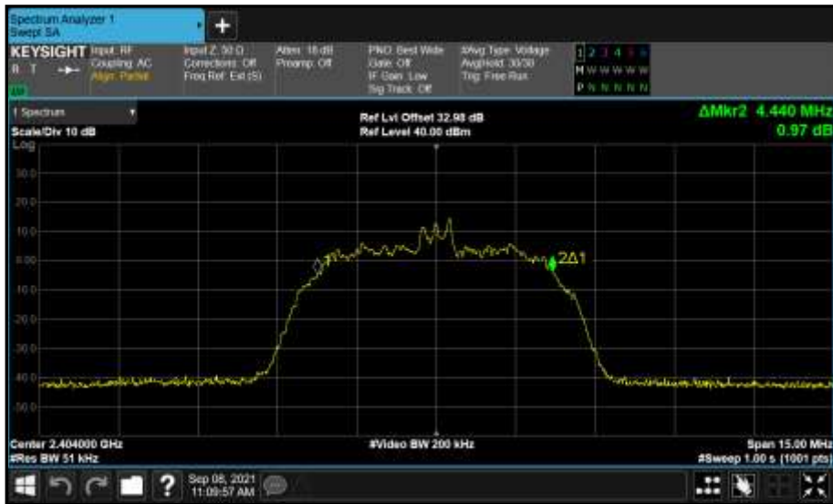
Figure 65 - Core 0 (A) 2404 MHz (CH2) 99% Bandwidth
