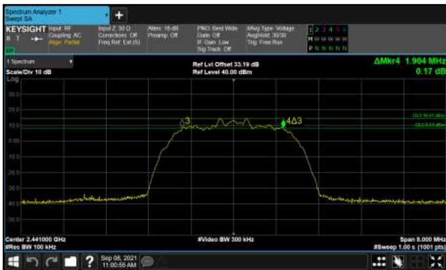
Figure 60 - Core 1 (B) 2441 MHz (CH39) 6 dB Bandwidth
