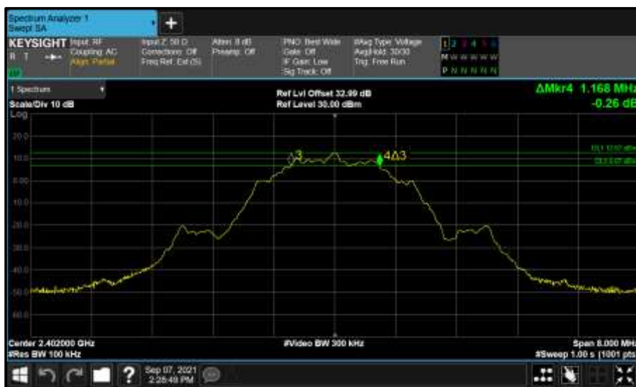
Figure 84 - Core 0 (A) 2402 MHz (CH37) 6 dB Bandwidth
