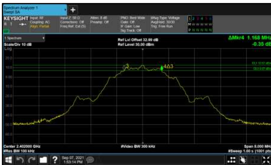
Figure 167 - Core 0 (A) 2402 MHz (CH37) 6 dB Bandwidth
