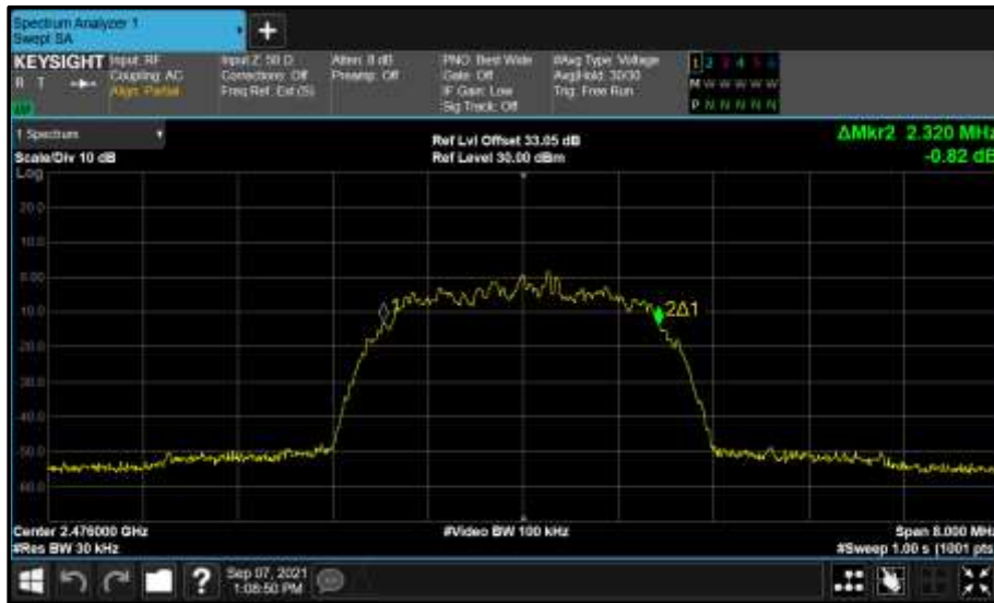
Figure 128 - Core 2 (C) 2476 MHz (CH74) 99% Bandwidth
