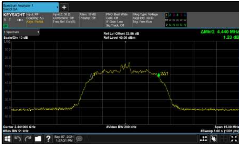
Figure 49 - Core 0 (A) 2441 MHz (CH39) 99% Bandwidth
