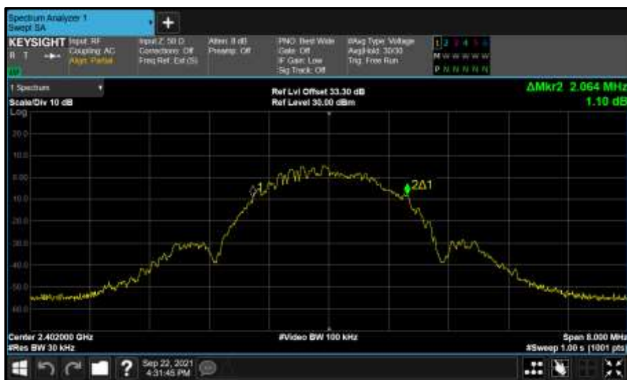
Figure 103 - Core 1 (B) 2402 MHz (CH37) 99% Bandwidth
