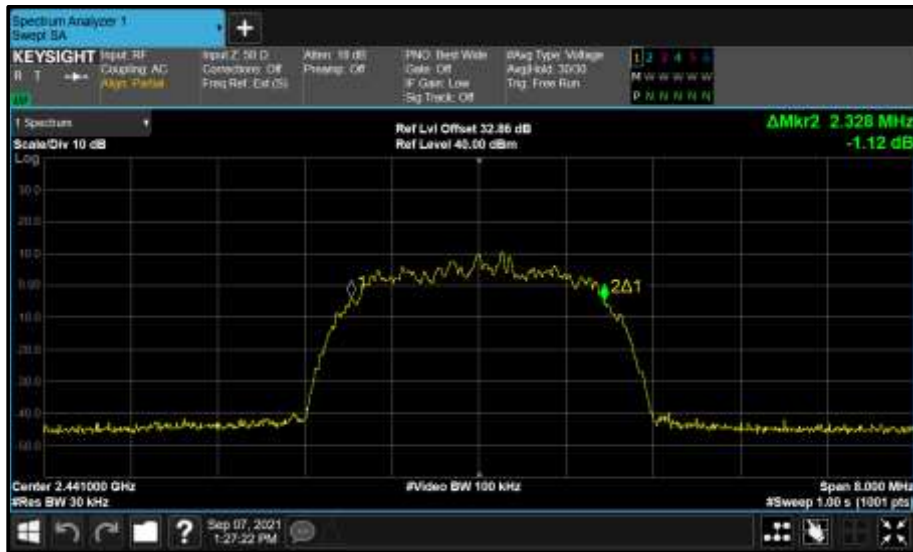
Figure 43 - Core 0 (A) 2441 MHz (CH39) 99% Bandwidth
