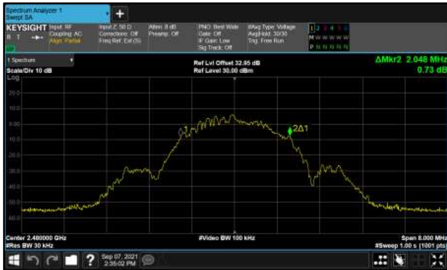
Figure 87 - Core 0 (A) 2480 MHz (CH39) 99% Bandwidth
