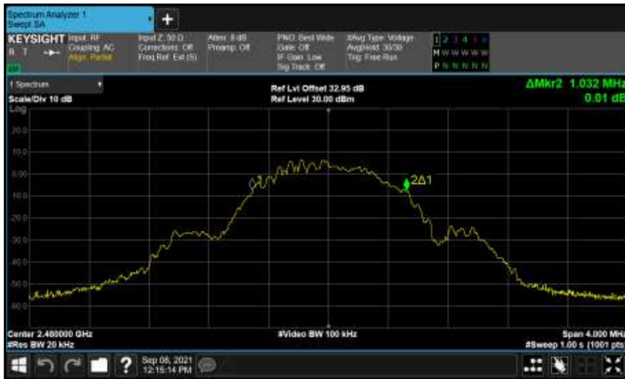
Figure 97 - Core 0 (A) 2480 MHz (CH39) 99% Bandwidth
