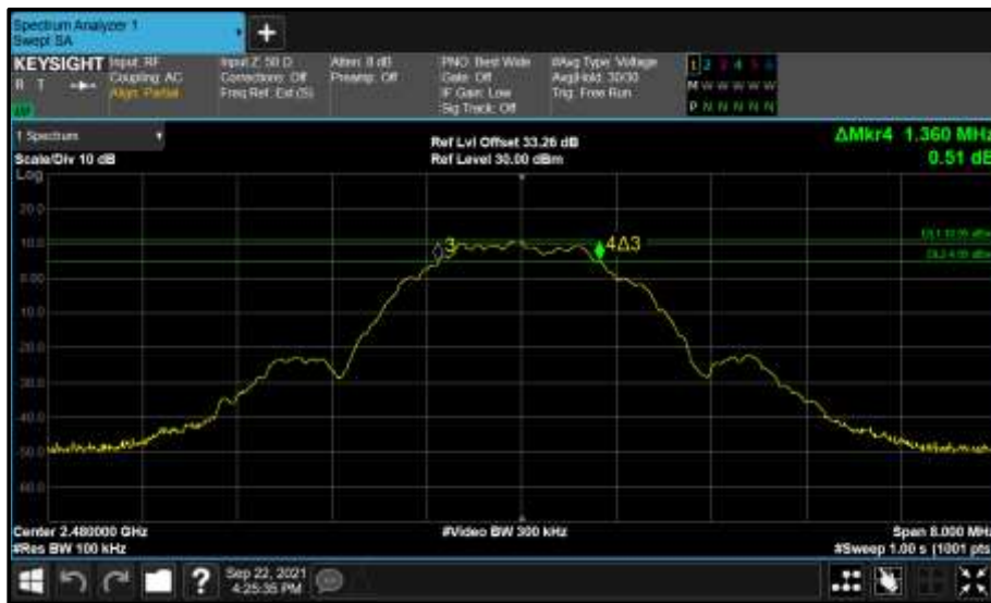
Figure 207 - Core 1 (B) 2480 MHz (CH39) 6 dB Bandwidth
