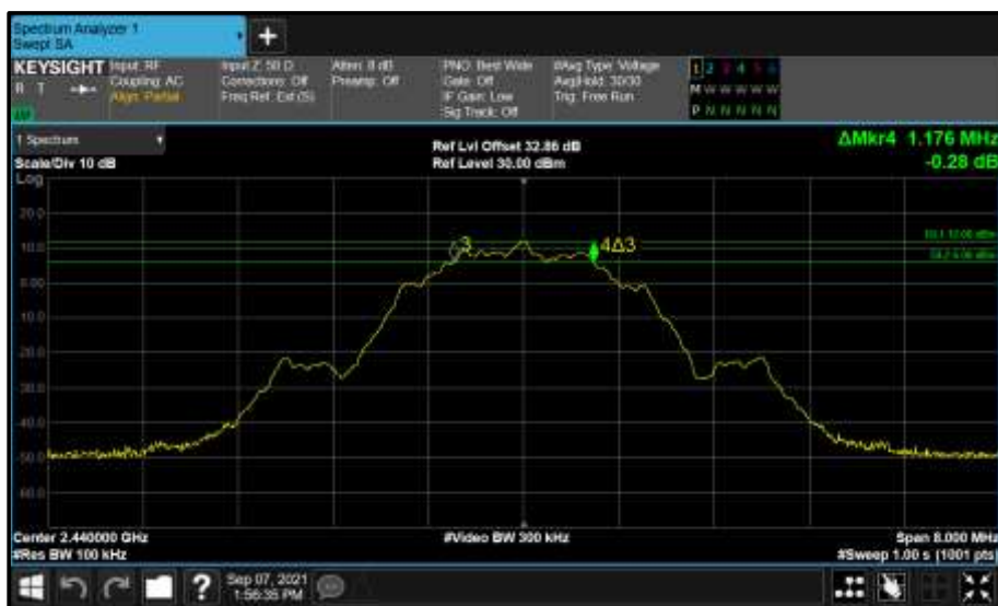
Figure 169 - Core 0 (A) 2440 MHz (CH17) 6 dB Bandwidth
