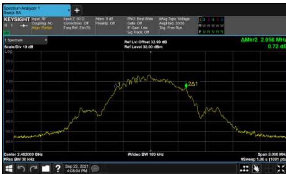
Figure 196 - Core 0 (A) 2402 MHz (CH37) 99% Bandwidth
