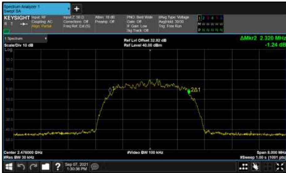
Figure 45 - Core 0 (A) 2476 MHz (CH74) 99% Bandwidth
