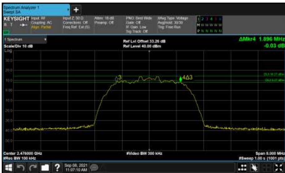
Figure 64 - Core 1 (B) 2476 MHz (CH74) 6 dB Bandwidth
