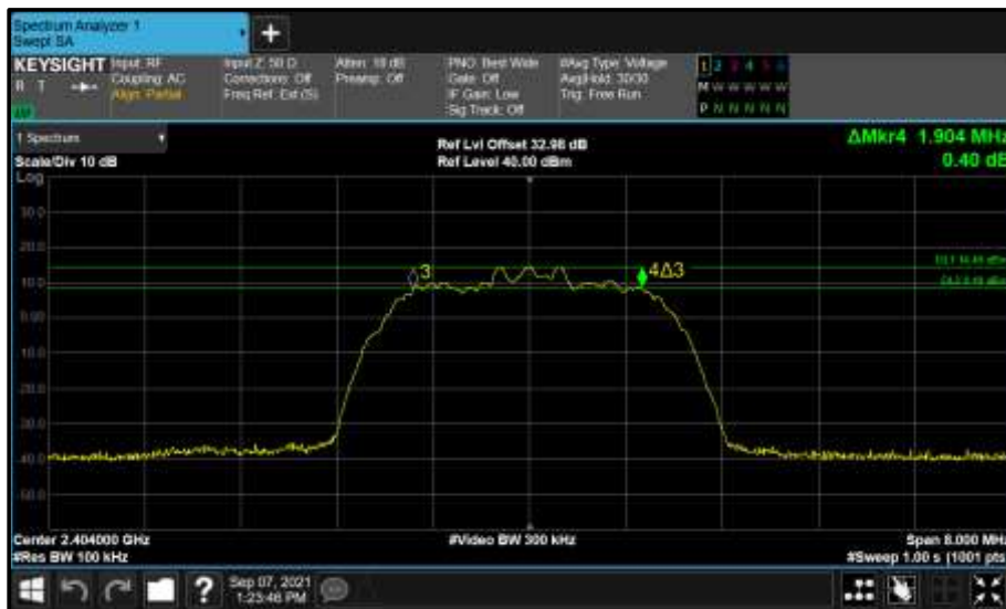
Figure 42 - Core 0 (A) 2404 MHz (CH2) 6 dB Bandwidth
