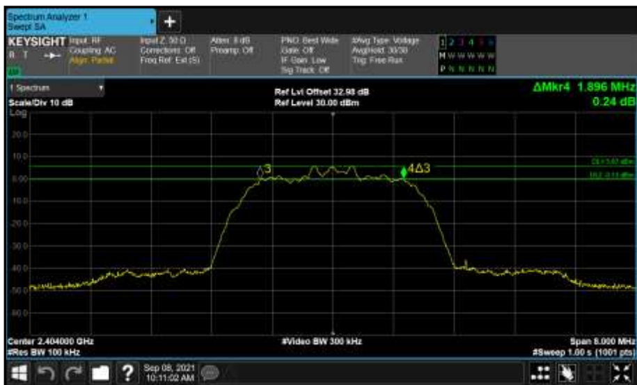
Figure 137 - Core 0 (A) 2404 MHz (CH2) 6 dB Bandwidth
