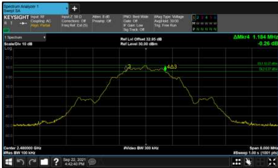
Figure 110 - Core 0 (A) 2480 MHz (CH39) 6 dB Bandwidth
