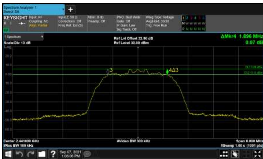
Figure 127 - Core 2 (C) 2441 MHz (CH39) 6 dB Bandwidth
