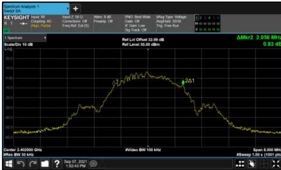
Figure 166 - Core 0 (A) 2402 MHz (CH37) 99% Bandwidth
