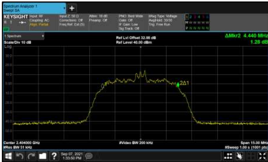
Figure 47 - Core 0 (A) 2404 MHz (CH2) 99% Bandwidth
