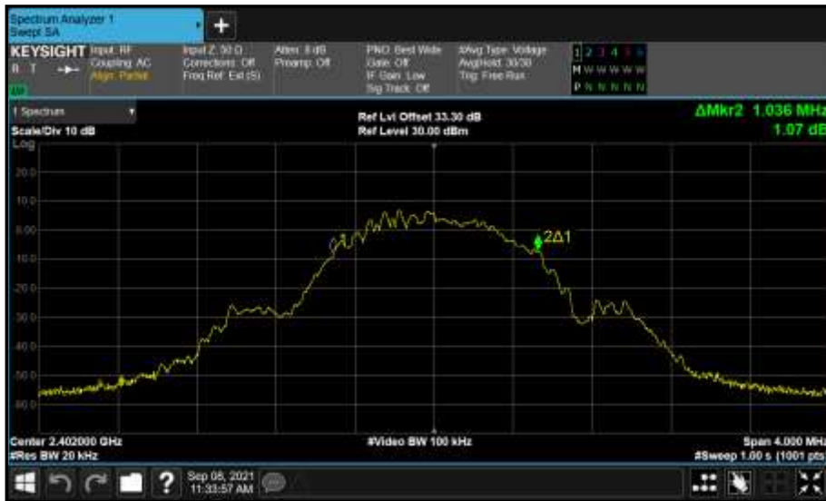
Figure 186 - Core 1 (B) 2402 MHz (CH37) 99% Bandwidth
