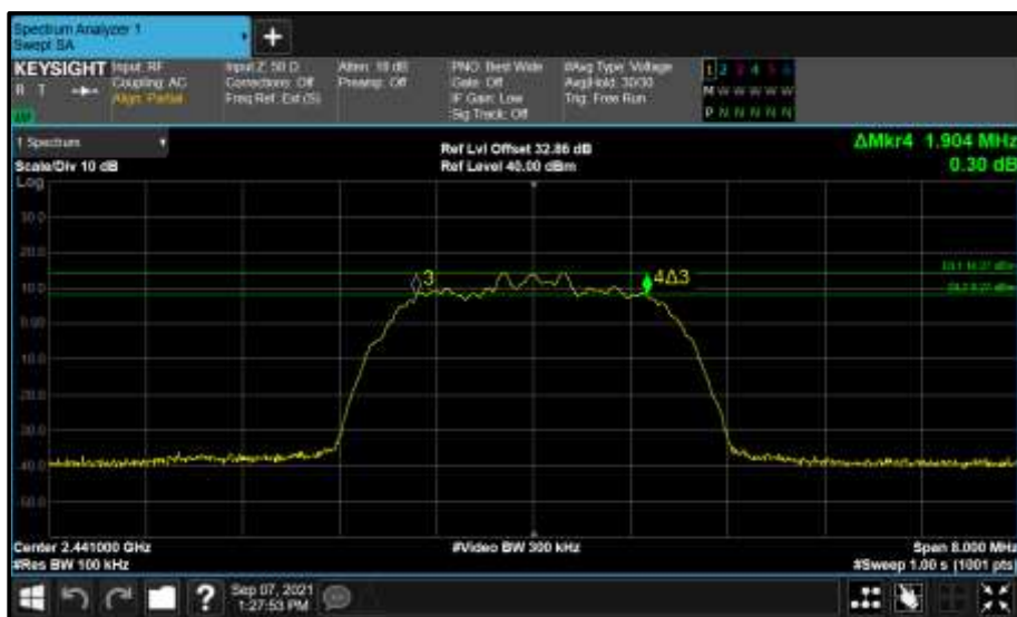
Figure 44 - Core 0 (A) 2441 MHz (CH39) 6 dB Bandwidth
