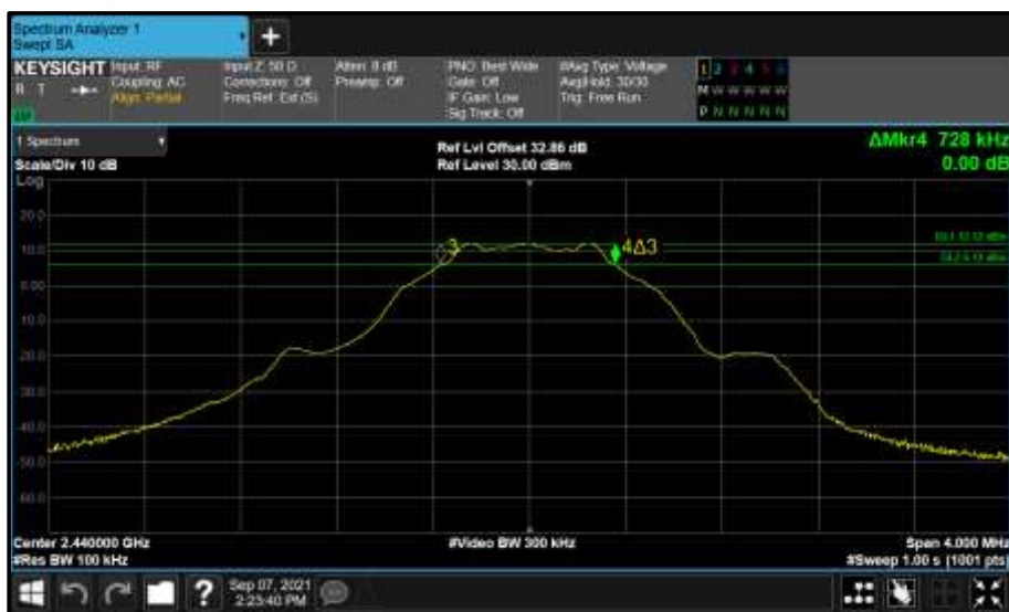
Figure 80 - Core 0 (A) 2440 MHz (CH17) 6 dB Bandwidth
