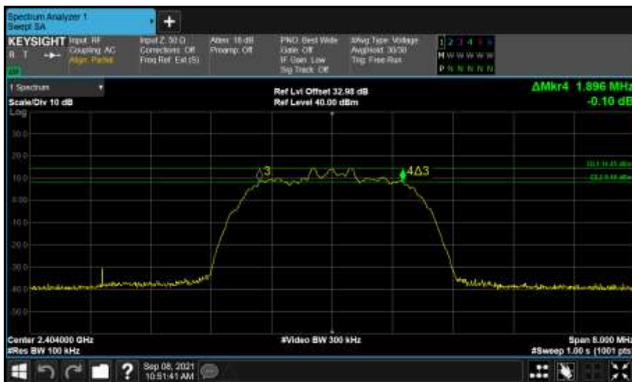
Figure 54 - Core 0 (A) 2404 MHz (CH2) 6 dB Bandwidth
