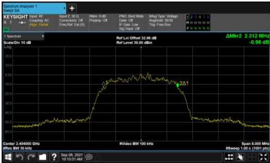
Figure 136 - Core 0 (A) 2404 MHz (CH2) 99% Bandwidth
