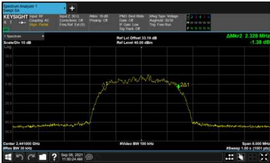
Figure 59 - Core 1 (B) 2441 MHz (CH39) 99% Bandwidth
