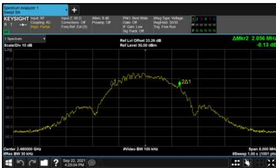
Figure 206 - Core 1 (B) 2480 MHz (CH39) 99% Bandwidth
