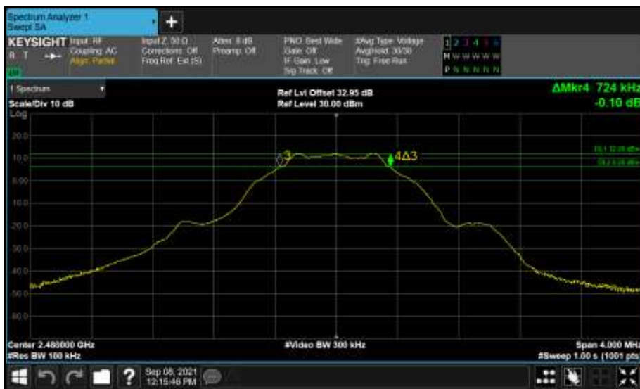
Figure 98 - Core 0 (A) 2480 MHz (CH39) 6 dB Bandwidth
