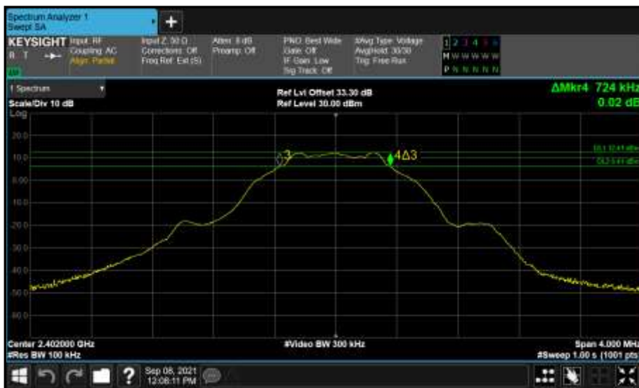
Figure 92 - Core 1 (B) 2402 MHz (CH37) 6 dB Bandwidth
