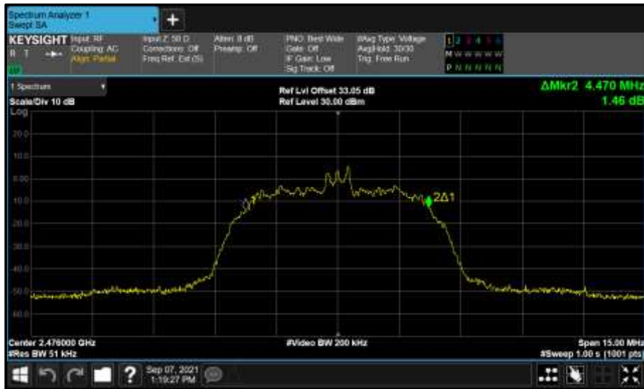
Figure 134 - Core 2 (C) 2476 MHz (CH74) 99% Bandwidth
