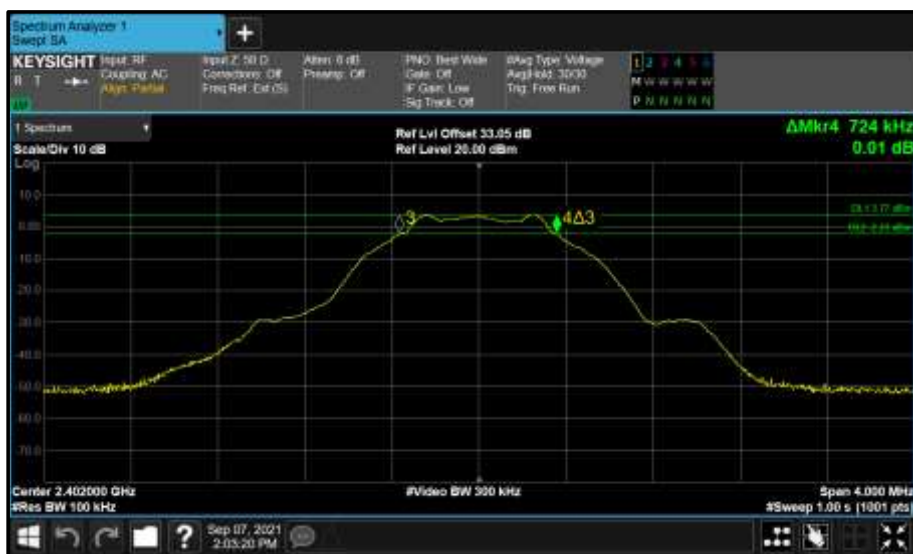
Figure 173 - Core 2 (C) 2402 MHz (CH37) 6 dB Bandwidth
