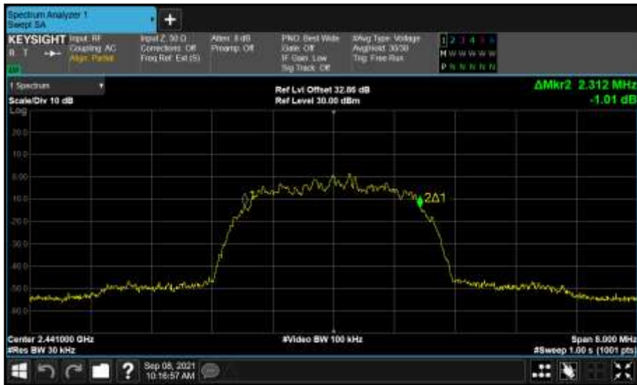
Figure 140 - Core 0 (A) 2441 MHz (CH39) 99% Bandwidth
