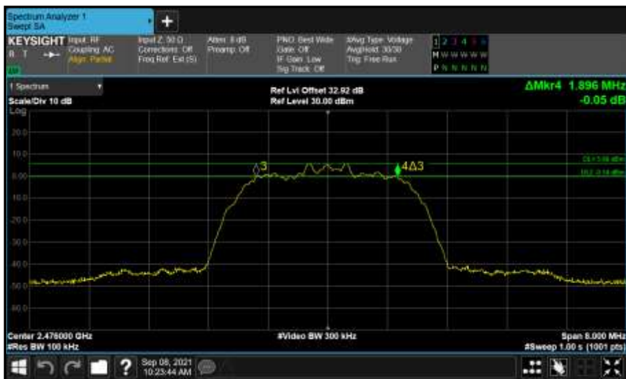
Figure 145 - Core 0 (A) 2476 MHz (CH74) 6 dB Bandwidth
