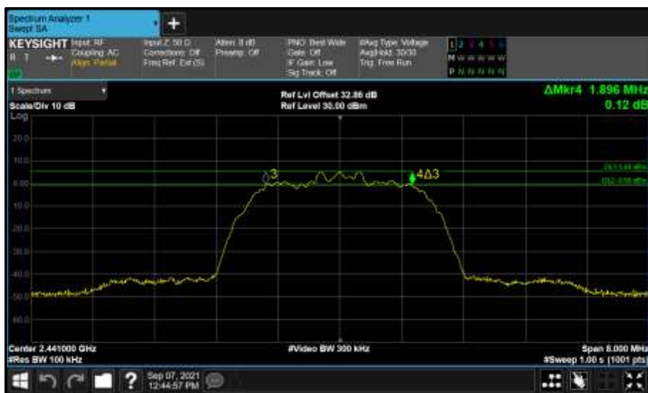
Figure 115 - Core 0 (A) 2441 MHz (CH39) 6 dB Bandwidth
