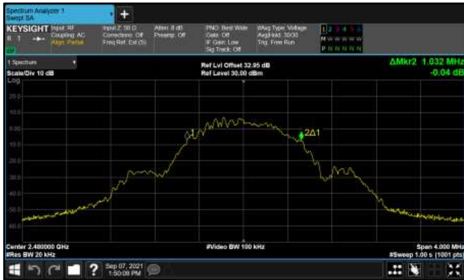
Figure 164 - Core 0 (A) 2480 MHz (CH39) 99% Bandwidth
