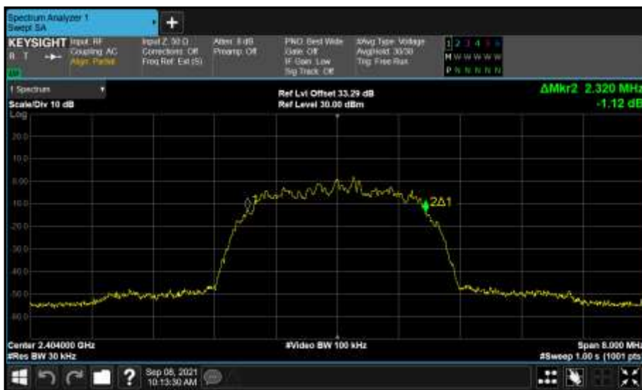
Figure 138 - Core 1 (B) 2404 MHz (CH2) 99% Bandwidth
