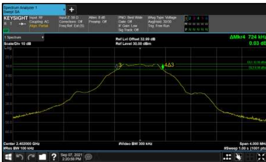
Figure 78 - Core 0 (A) 2402 MHz (CH37) 6 dB Bandwidth
