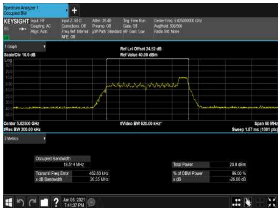
Figure 730 - 5825 MHz - 99% Occupied Bandwidth
