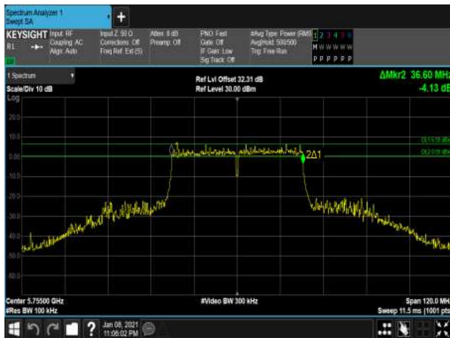
Figure 761 - 5755 MHz - 6 dB DTS Bandwidth
