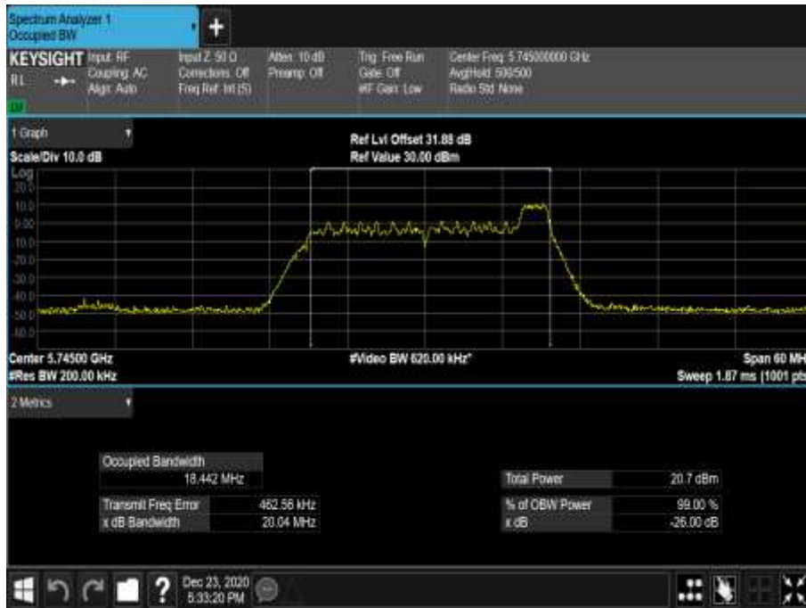
Figure 694 - 5745 MHz - 99% Occupied Bandwidth
