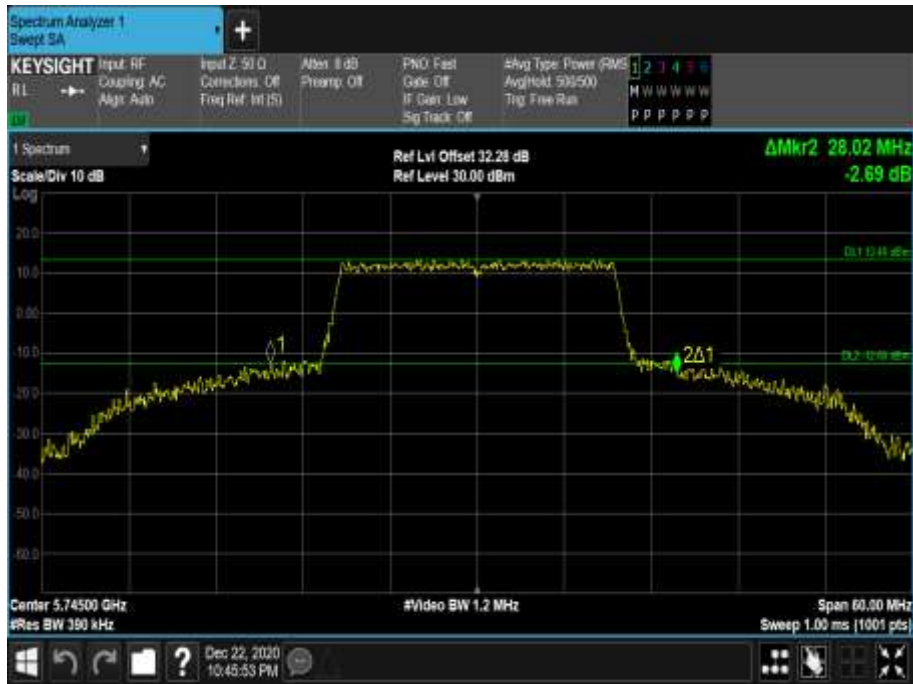
Figure 675 - 5745 MHz - 26 dB Emission Bandwidth
