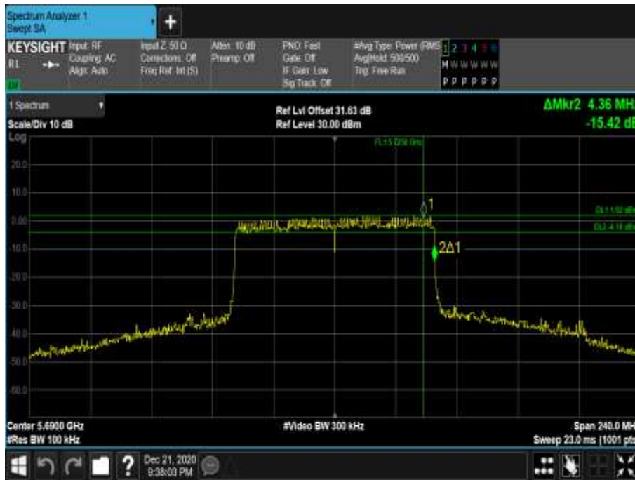
Figure 854 - 5690 MHz - 6 dB DTS Bandwidth
