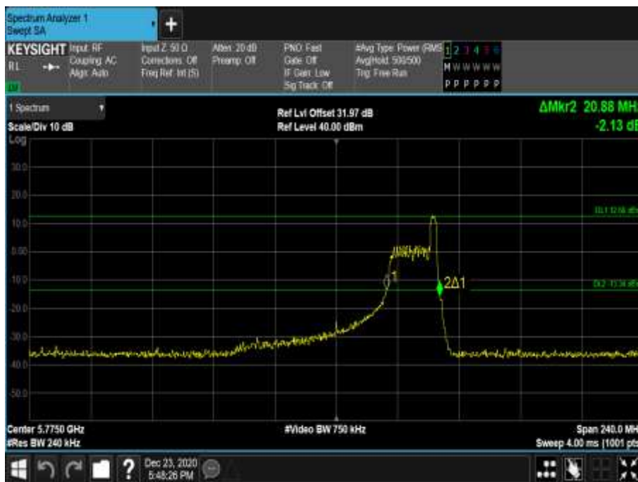
Figure 876 - 5775 MHz - 26 dB Emission Bandwidth
