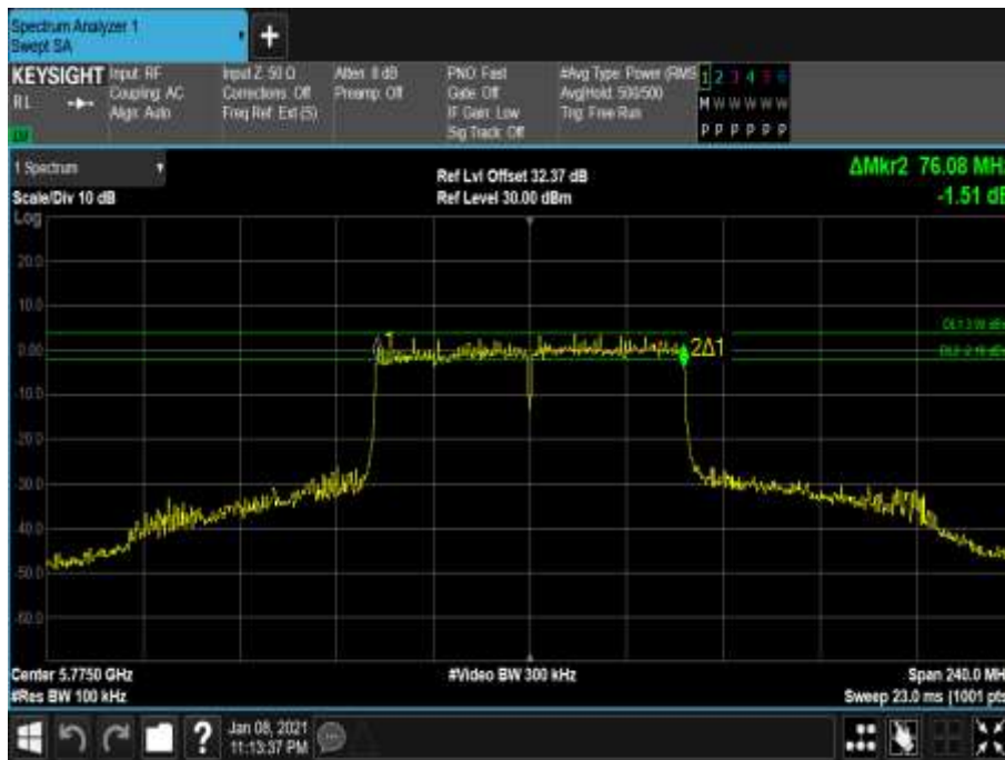
Figure 851 - 5775 MHz - 6 dB DTS Bandwidth
