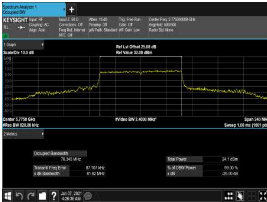
Figure 841 - 5775 MHz - 99% Occupied Bandwidth
