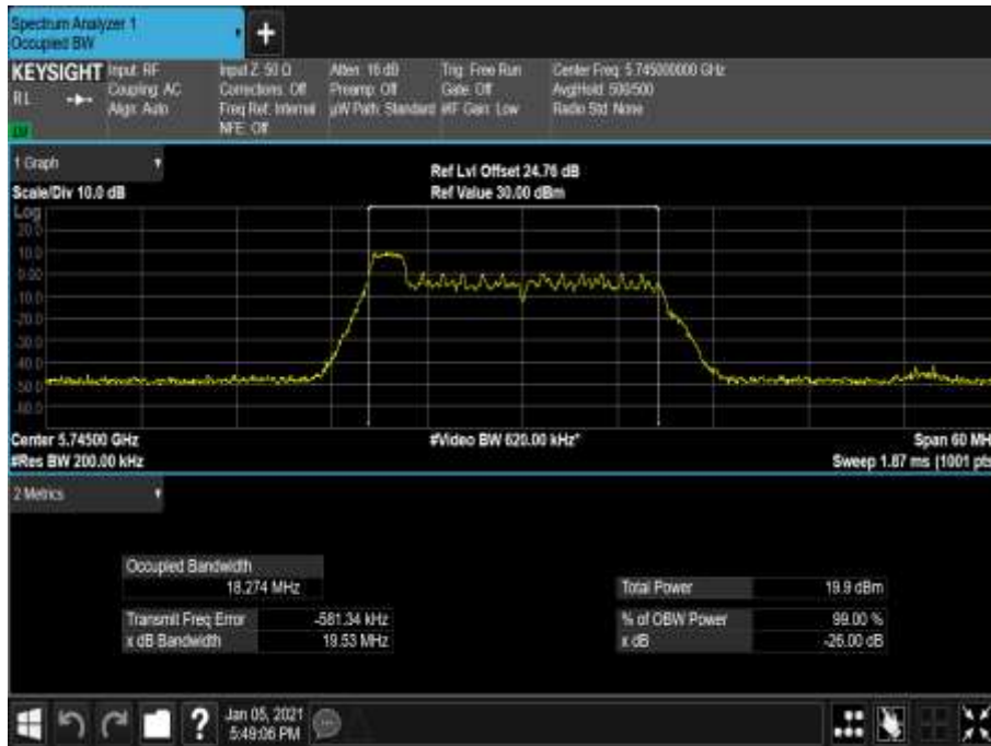
Figure 715 - 5745 MHz - 99% Occupied Bandwidth
