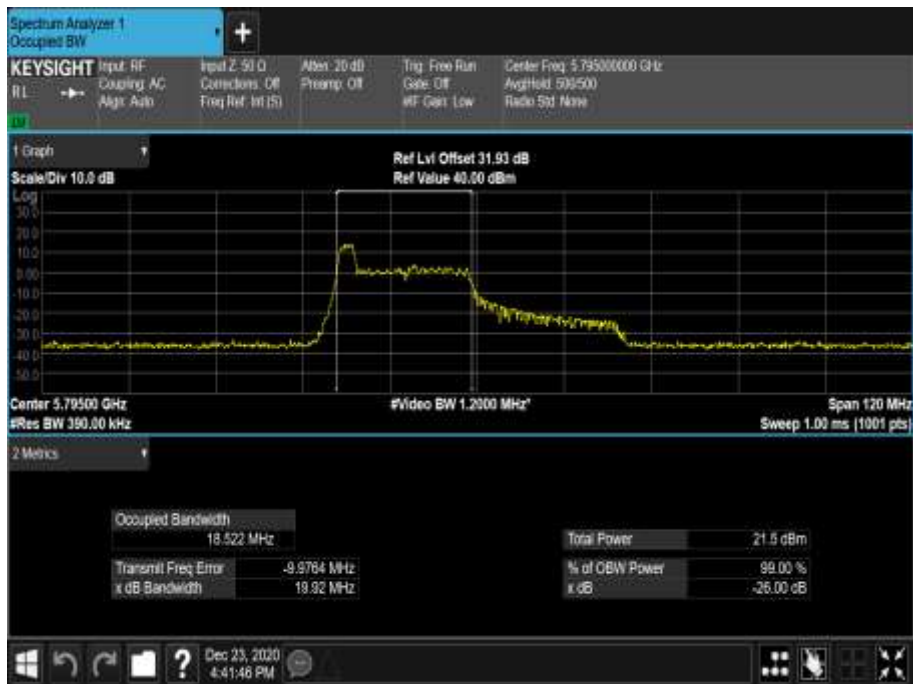
Figure 802 - 5795 MHz - 99% Occupied Bandwidth
