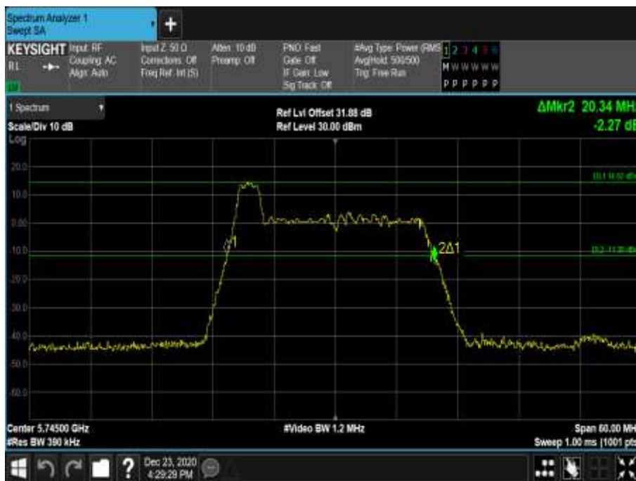
Figure 684 - 5745 MHz - 26 dB Emission Bandwidth
