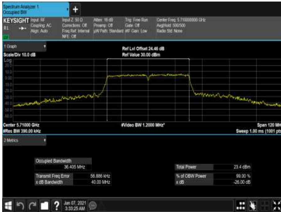
Figure 742 - 5710 MHz - 99% Occupied Bandwidth
