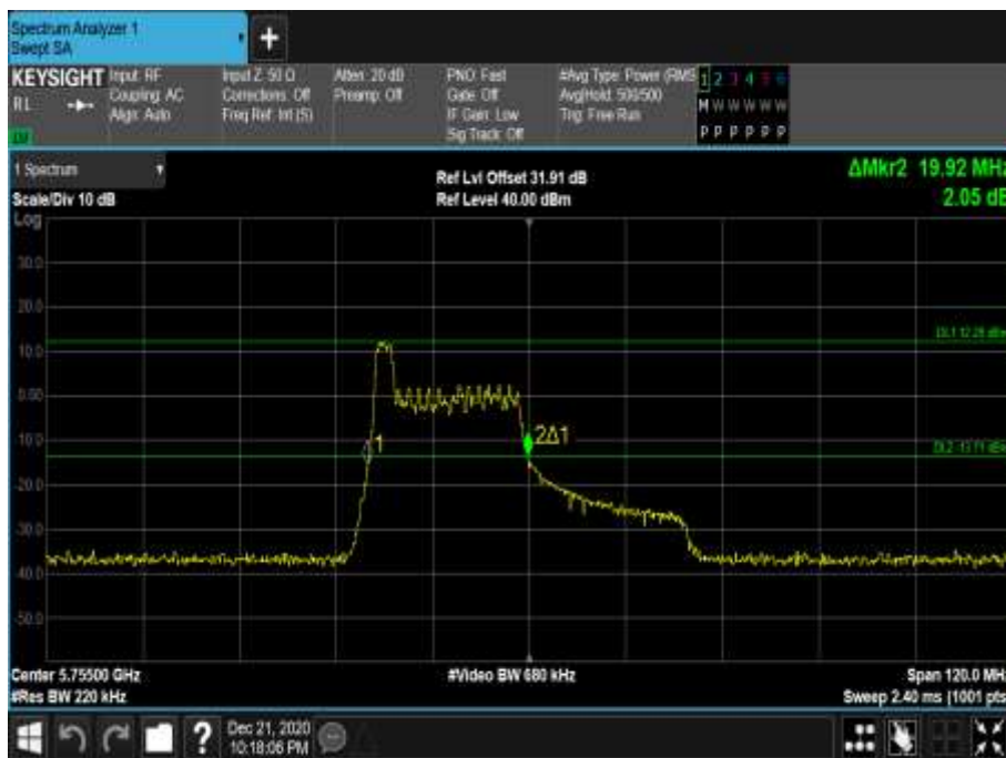
Figure 777 - 5755 MHz - 26 dB Emission Bandwidth
