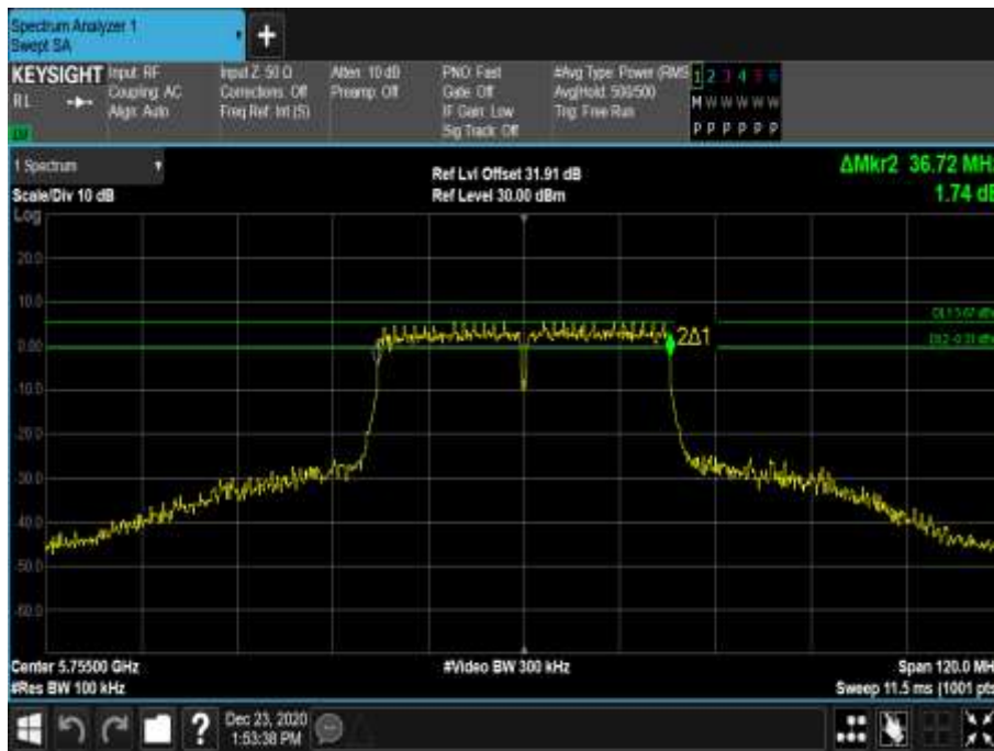
Figure 743 - 5755 MHz - 6 dB DTS Bandwidth
