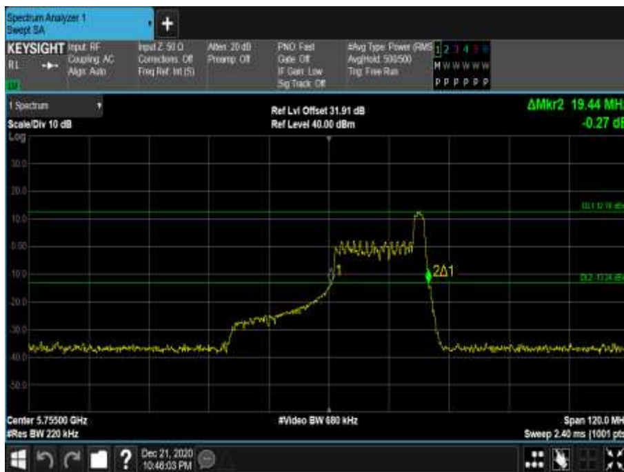
Figure 783 - 5755 MHz - 26 dB Emission Bandwidth
