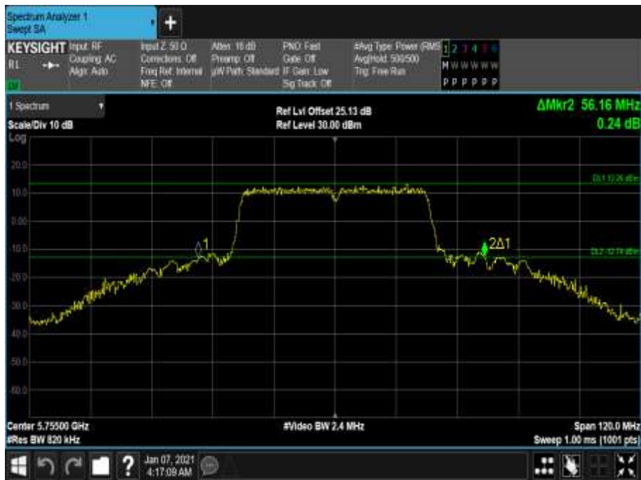
Figure 753 - 5755 MHz - 26 dB Emission Bandwidth
