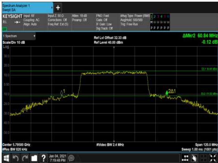
Figure 816 - 5795 MHz - 26 dB Emission Bandwidth
