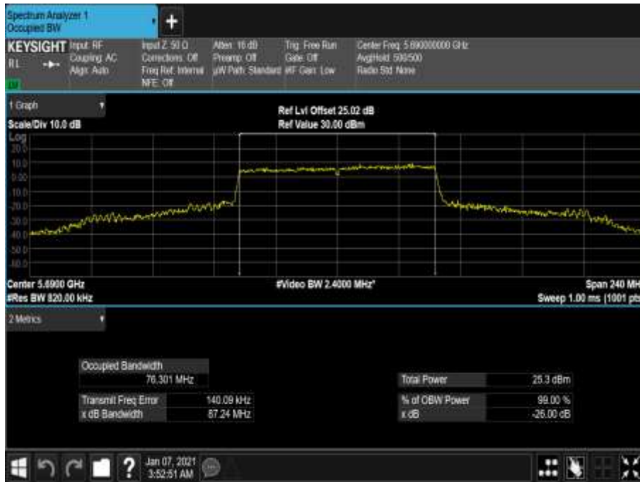
Figure 832 - 5690 MHz - 99% Occupied Bandwidth
