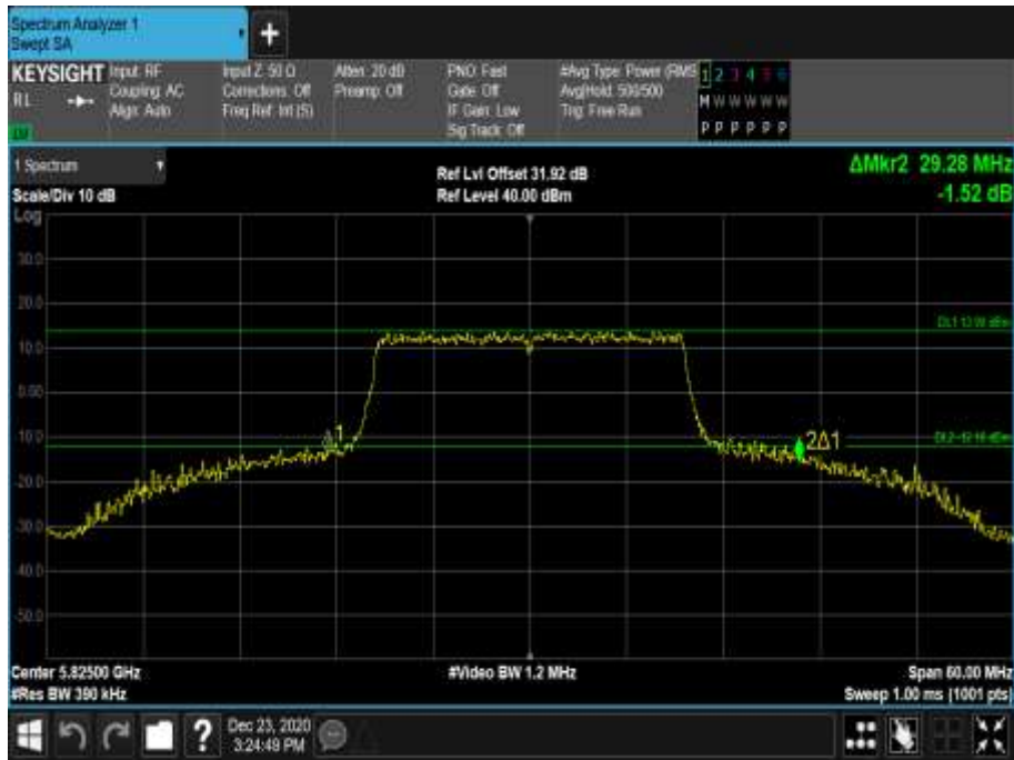
Figure 681 - 5825 MHz - 26 dB Emission Bandwidth
