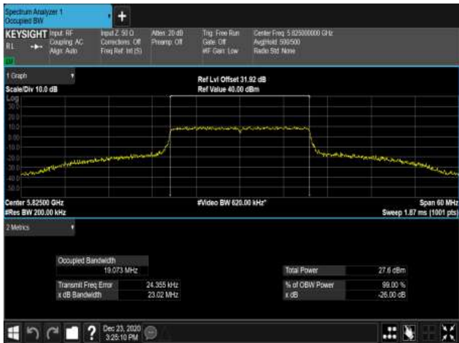
Figure 682 - 5825 MHz - 99% Occupied Bandwidth
