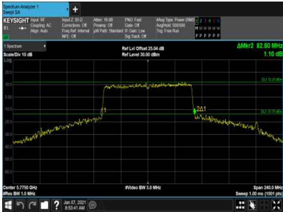
Figure 870 - 5775 MHz - 26 dB Emission Bandwidth
