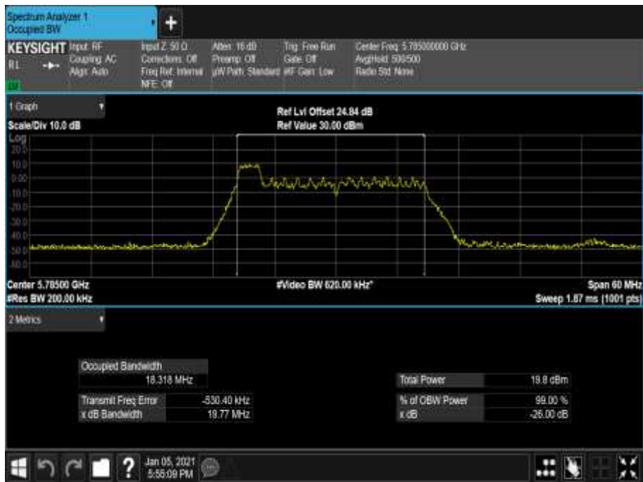
Figure 718 - 5785 MHz - 99% Occupied Bandwidth
