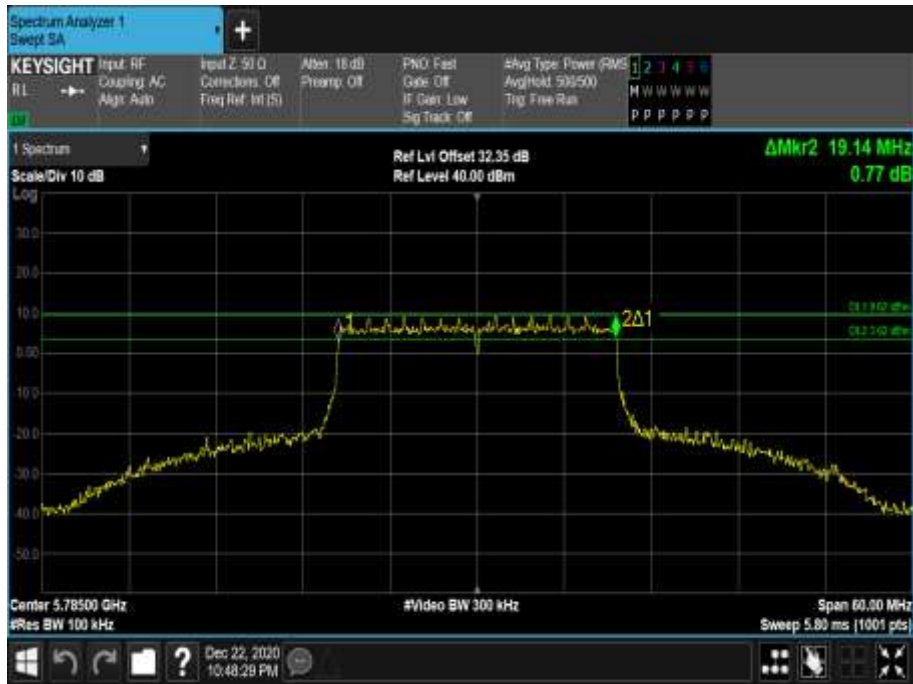
Figure 677 - 5785 MHz - 6 dB DTS Bandwidth
