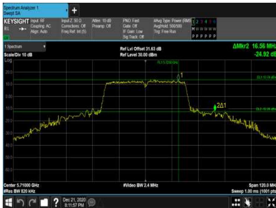
Figure 732 - 5710 MHz - 26 dB Emission Bandwidth
