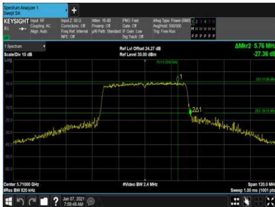
Figure 789 - 5710 MHz - 26 dB Emission Bandwidth
