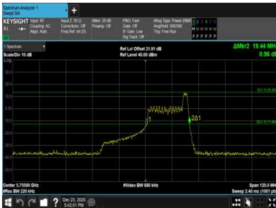
Figure 804 - 5755 MHz - 26 dB Emission Bandwidth
