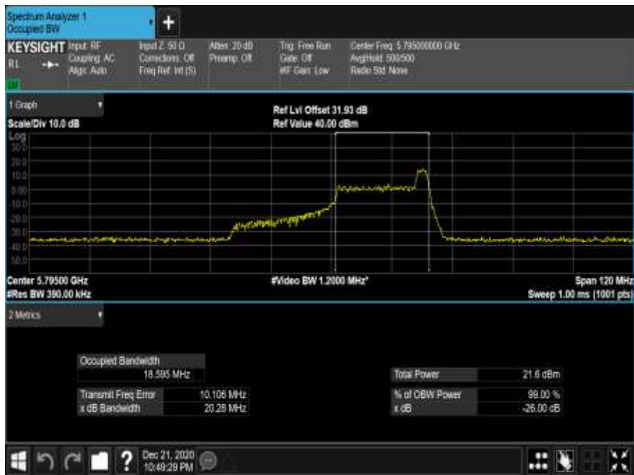
Figure 787 - 5795 MHz - 99% Occupied Bandwidth
