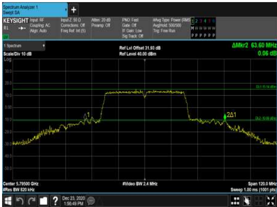
Figure 747 - 5795 MHz - 26 dB Emission Bandwidth
