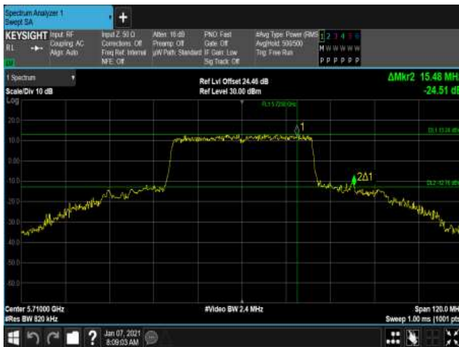
Figure 810 - 5710 MHz - 26 dB Emission Bandwidth
