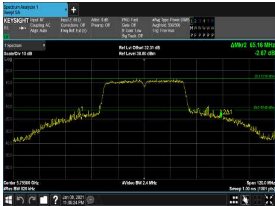
Figure 762 - 5755 MHz - 26 dB Emission Bandwidth
