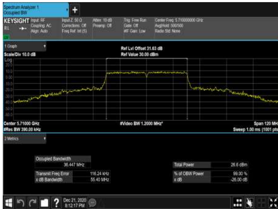
Figure 733 - 5710 MHz - 99% Occupied Bandwidth
