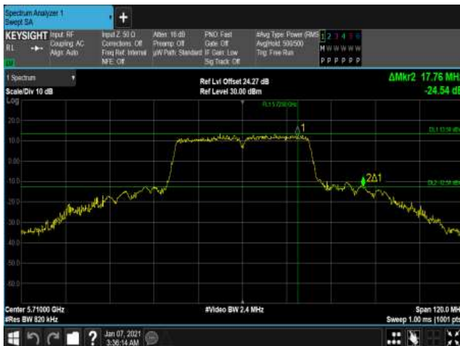
Figure 750 - 5710 MHz - 26 dB Emission Bandwidth
