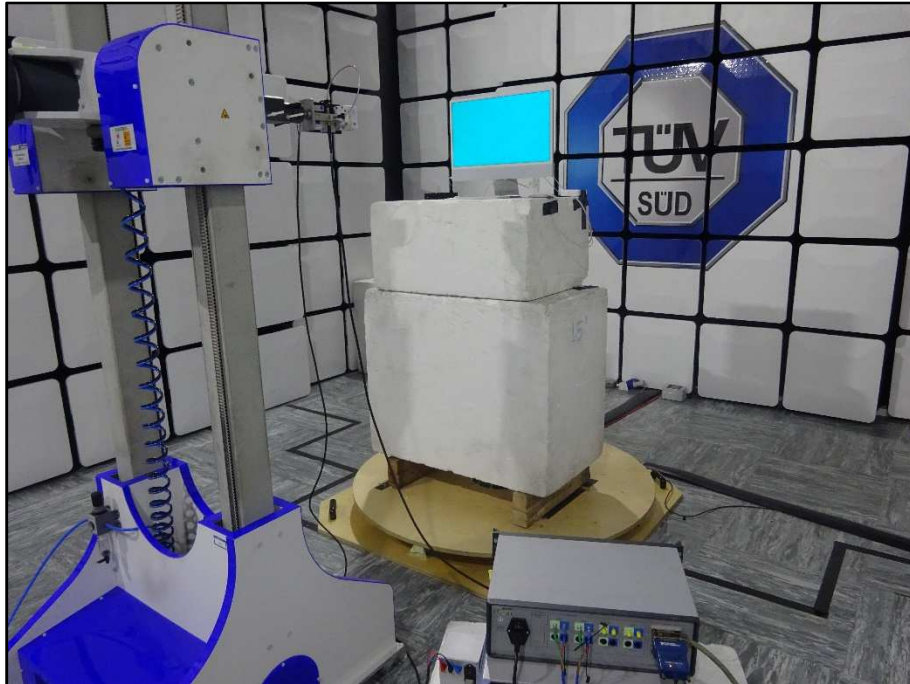
Figure 3 Radiated Disturbance - Above 1 GHz
