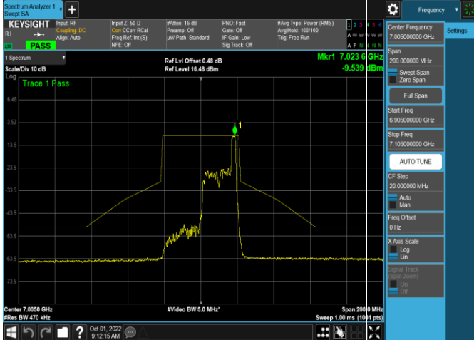
Plot 7-621. In-Band Emission Plot SDM Antenna 5b (40MHz 802.11ax RU26 (UNII Band 8) – Ch. 211)
