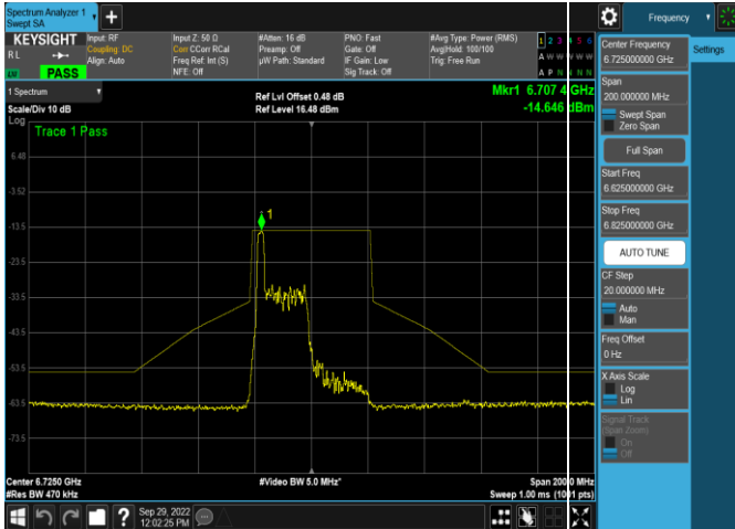
Plot 7-585. In-Band Emission Plot SDM Antenna 5b (40MHz 802.11ax RU26 (UNII Band 7) – Ch. 155)
