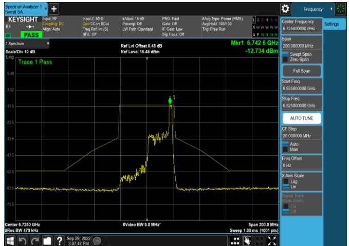
Plot 7-589. In-Band Emission Plot SDM Antenna 5b (40MHz 802.11ax RU26 (UNII Band 7) – Ch. 155)
