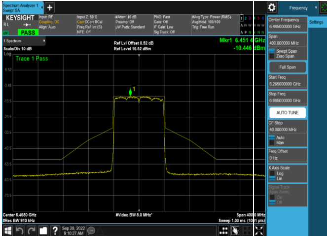
Plot 7-567. In-Band Emission Plot SDM Antenna 5b (80MHz 802.11ax RU996 (UNII Band 6) – Ch. 103)
