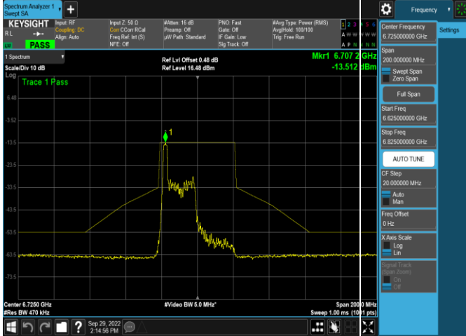
Plot 7-421. In-Band Emission Plot Antenna 5b (40MHz 802.11ax RU26 (UNII Band 7) – Ch. 155)
