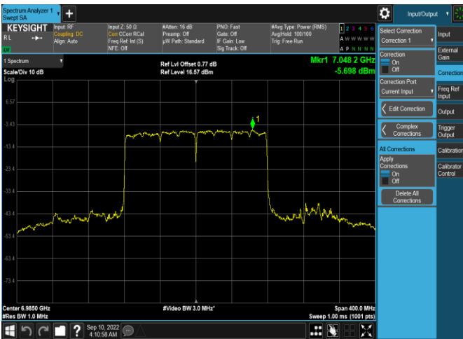
Plot 7-384. Power Spectral Density Plot SDM Antenna 4a (160MHz 802.11ax RU996x2 (UNII Band 8) – Ch. 207)
