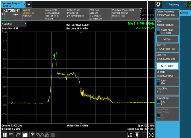
Plot 7-229. Power Spectral Density Plot Antenna 4a (40MHz 802.11ax RU26 (UNII Band 7) – Ch. 155)
