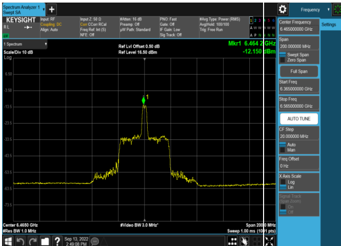
Plot 7-154. Power Spectral Density Plot Antenna 5b (80MHz 802.11ax RU26 (UNII Band 6) – Ch. 103)
