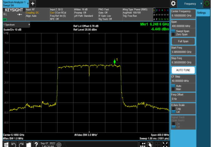
Plot 7-144. Power Spectral Density Plot Antenna 5b (160MHz 802.11ax RU996x2 (UNII Band 5) – Ch. 47)
