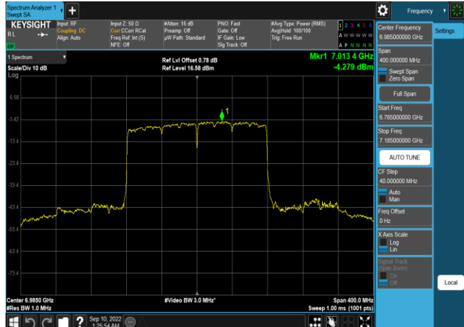
Plot 7-192. Power Spectral Density Plot Antenna 5b (160MHz 802.11ax RU996x2 (UNII Band 8) – Ch. 207)
