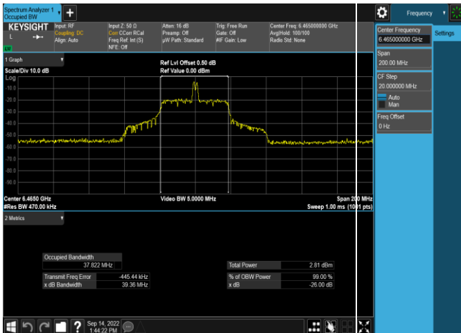
Plot 7-90. 26dB & 99% Bandwidth Plot Antenna 4a (80MHz 802.11ax RU26 (UNII Band 6) – Ch. 103)
