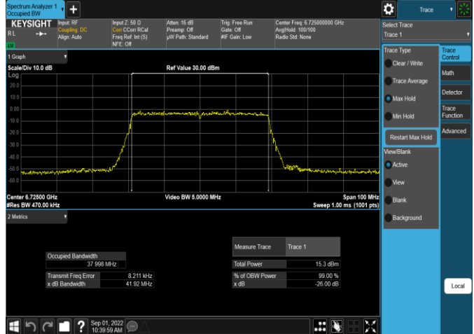
Plot 7-104. 26dB & 99% Bandwidth Plot Antenna 4a (40MHz 802.11ax RU484 (UNII Band 7) – Ch. 155)
