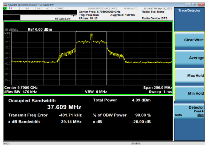
Plot 7-106. 26dB & 99% Bandwidth Plot Antenna 4a (80MHz 802.11ax RU26 (UNII Band 7) – Ch. 151)
