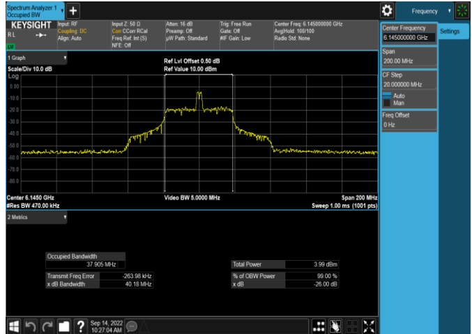
Plot 7-74. 26dB & 99% Bandwidth Plot Antenna 4a (80MHz 802.11ax RU26 (UNII Band 5) – Ch. 39)
