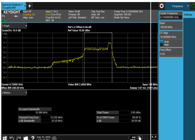
Plot 7-103. 26dB & 99% Bandwidth Plot Antenna 4a (40MHz 802.11ax RU26 (UNII Band 7) – Ch. 155)
