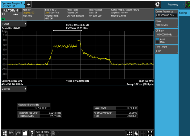
Plot 7-102. 26dB & 99% Bandwidth Plot Antenna 4a (40MHz 802.11ax RU26 (UNII Band 7) – Ch. 155)
