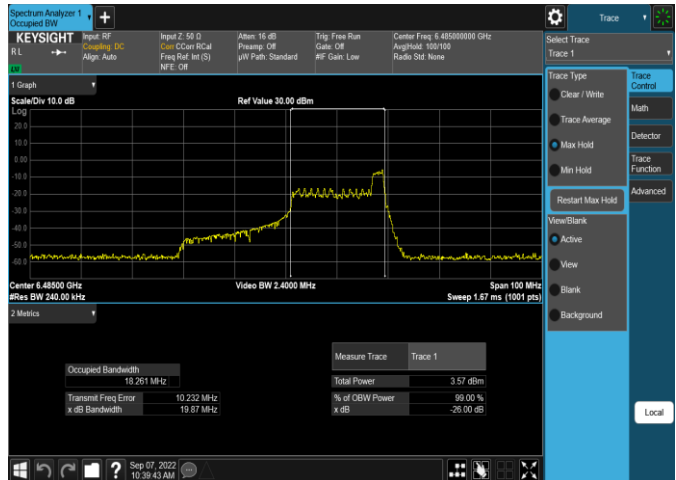
Plot 7-87. 26dB & 99% Bandwidth Plot Antenna 4a (40MHz 802.11ax RU26 (UNII Band 6) – Ch. 107)
