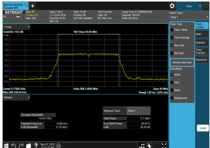
Plot 7-68. 26dB & 99% Bandwidth Plot Antenna 4a (20MHz 802.11ax RU242 (UNII Band 5) – Ch. 45)
