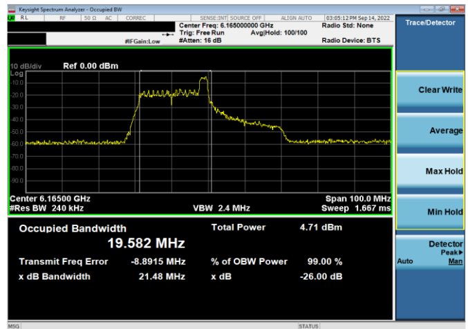
Plot 7-70. 26dB & 99% Bandwidth Plot Antenna 4a (40MHz 802.11ax RU26 (UNII Band 5) – Ch. 43)
