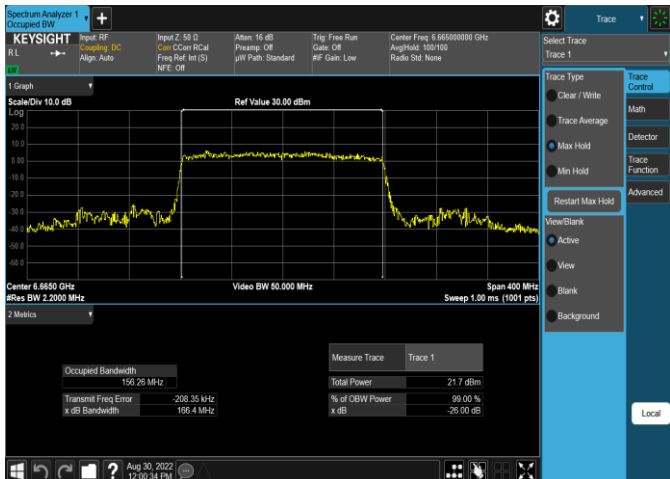
Plot 7-48. 26dB & 99% Bandwidth Plot Antenna 5b (160MHz 802.11ax RU484 (UNII Band 7) – Ch. 143)
