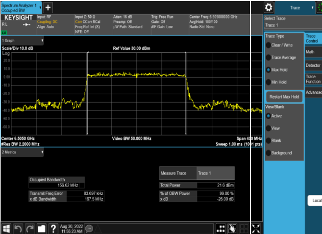
Plot 7-32. 26dB & 99% Bandwidth Plot Antenna 5b (160MHz 802.11ax RU484 (UNII Band 6) – Ch. 111)
