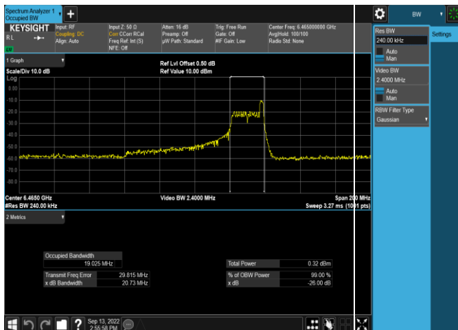
Plot 7-27. 26dB & 99% Bandwidth Plot Antenna 5b (80MHz 802.11ax RU26 (UNII Band 6) – Ch. 103)
