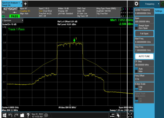
Plot 7-527. In-Band Emission Plot SDM Antenna 5b (160MHz 802.11ax (UNII Band 8) – Ch. 207, MCS4)
