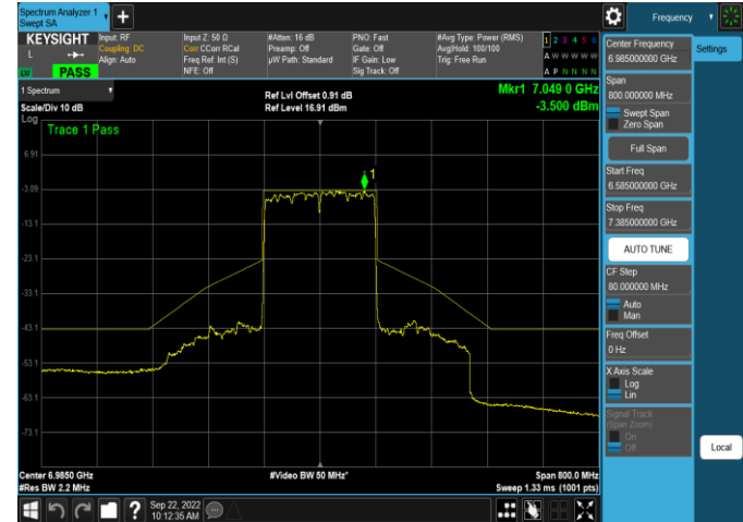
Plot 7-528. In-Band Emission Plot SDM Antenna 4a (160MHz 802.11ax (UNII Band 8) – Ch. 207, MCS4)
