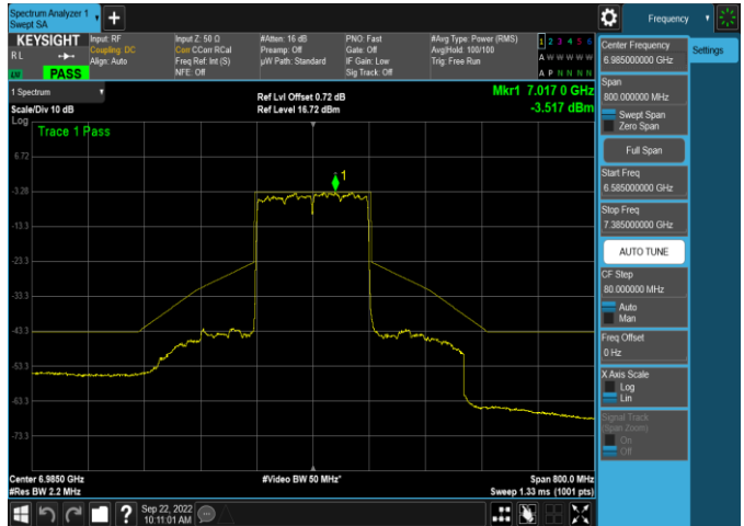
Plot 7-496. In-Band Emission Plot SDM Antenna 4a (160MHz 802.11ax (UNII Band 8) – Ch. 207, MCS2)
