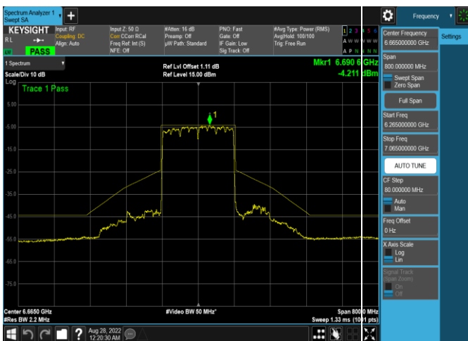
Plot 7-455. In-Band Emission Plot Antenna 4a (160MHz 802.11ax (UNII Band 7) – Ch. 143, MCS11)
