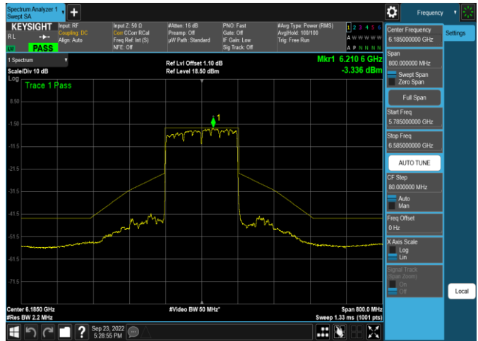
Plot 7-385. In-Band Emission Plot Antenna 5b (160MHz 802.11ax (UNII Band 5) – Ch. 47, MCS11)
