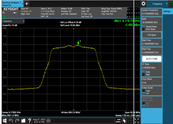
Plot 7-205. Power Spectral Density Plot Antenna 4a (20MHz 802.11a (UNII Band 5) – Ch. 45, MCS4)
