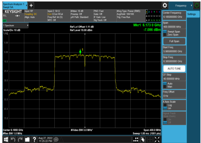
Plot 7-229. Power Spectral Density Plot Antenna 4a (160MHz 802.11ax (UNII Band 5) – Ch. 47, MCS11)
