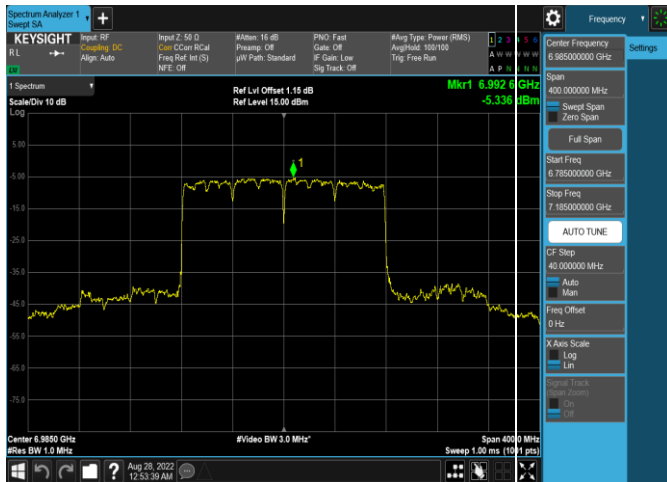
Plot 7-244. Power Spectral Density Plot Antenna 4a (160MHz 802.11ax (UNII Band 8) – Ch. 207, MCS11)
