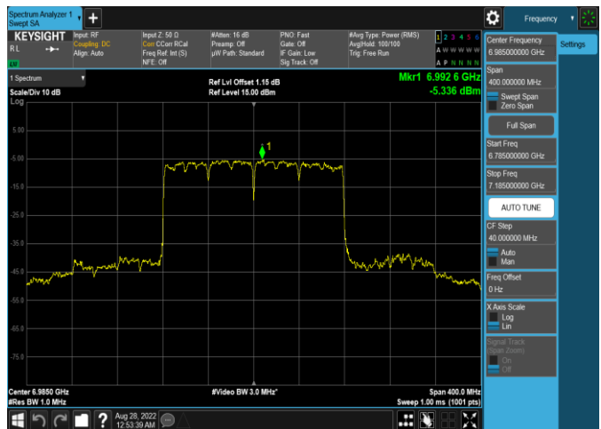
Plot 7-248. Power Spectral Density Plot Antenna 4a (160MHz 802.11ax (UNII Band 8) – Ch. 207, MCS11)
