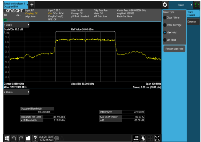
Plot 7-120. 26dB & 99% Bandwidth Plot Antenna 4a (160MHz 802.11ax (UNII Band 8) – Ch. 207, MCS11)
