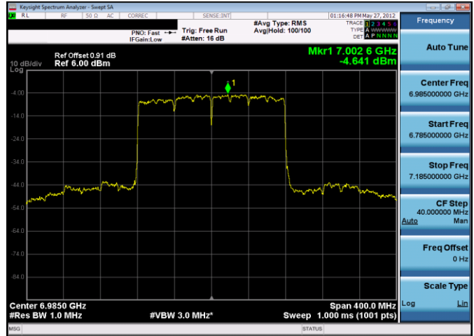
Plot 7-160. Power Spectral Density Plot Antenna 5b (160MHz 802.11ax (UNII Band 8) – Ch. 207, MCS4)
