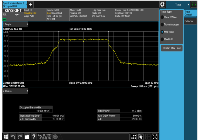
Plot 7-116. 26dB & 99% Bandwidth Plot Antenna 4a (20MHz 802.11a (UNII Band 8) – Ch. 209, MCS11)
