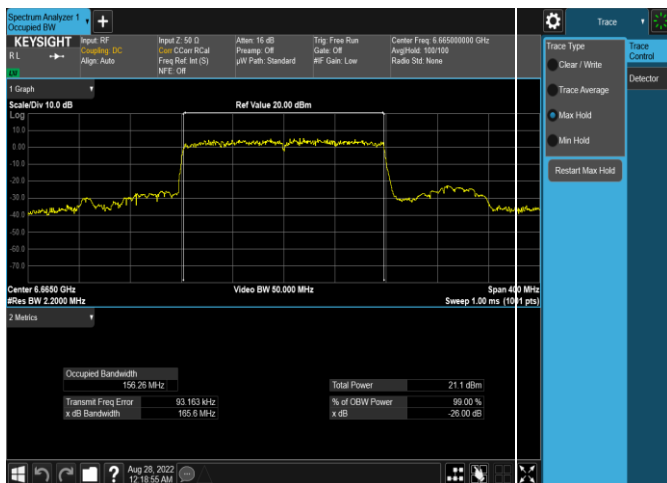
Plot 7-115. 26dB & 99% Bandwidth Plot Antenna 4a (160MHz 802.11ax (UNII Band 7) – Ch. 143, MCS11)
