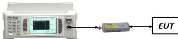
Figure 7-2. Test Instrument & Measurement Setup
