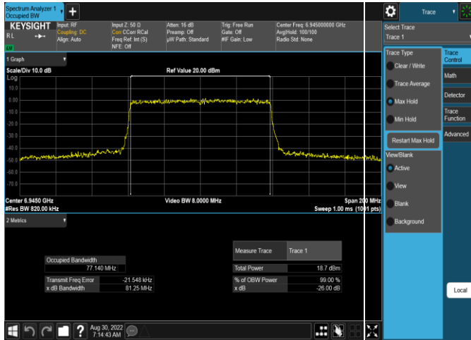
Plot 7-119. 26dB & 99% Bandwidth Plot Antenna 4a (80MHz 802.11ax (UNII Band 8) – Ch. 199, MCS11)
