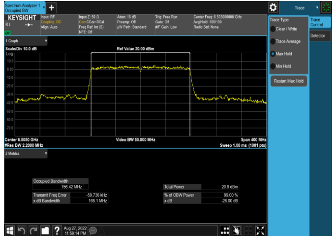
Plot 7-90. 26dB & 99% Bandwidth Plot Antenna 4a (160MHz 802.11ax (UNII Band 6) – Ch. 111, MCS4)
