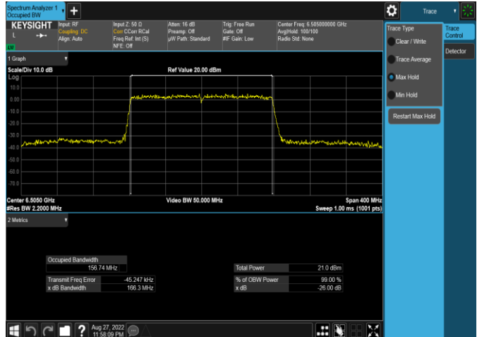
Plot 7-70. 26dB & 99% Bandwidth Plot Antenna 4a (160MHz 802.11ax (UNII Band 6) – Ch. 111, MCS2)
