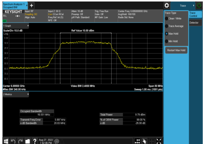
Plot 7-71. 26dB & 99% Bandwidth Plot Antenna 4a (20MHz 802.11a (UNII Band 7) – Ch. 149, MCS2)
