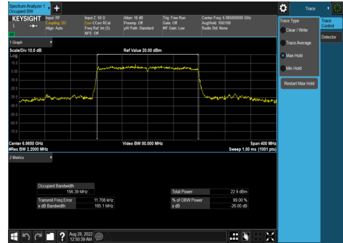
Plot 7-100. 26dB & 99% Bandwidth Plot Antenna 4a (160MHz 802.11ax (UNII Band 8) – Ch. 207, MCS4)
