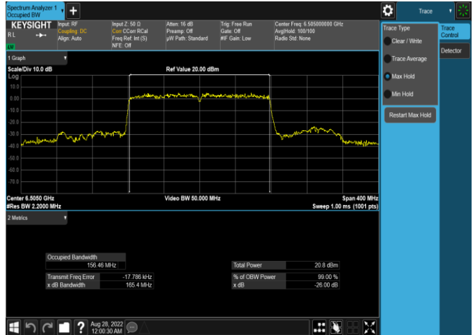
Plot 7-110. 26dB & 99% Bandwidth Plot Antenna 4a (160MHz 802.11ax (UNII Band 6) – Ch. 111, MCS11)
