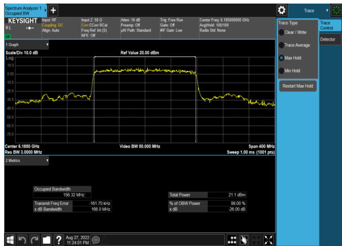
Plot 7-105. 26dB & 99% Bandwidth Plot Antenna 4a (160MHz 802.11ax (UNII Band 5) – Ch. 47, MCS11)
