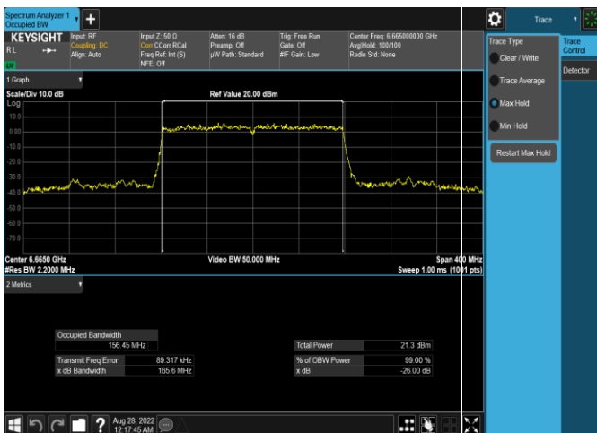
Plot 7-95. 26dB & 99% Bandwidth Plot Antenna 4a (160MHz 802.11ax (UNII Band 7) – Ch. 143, MCS4)
