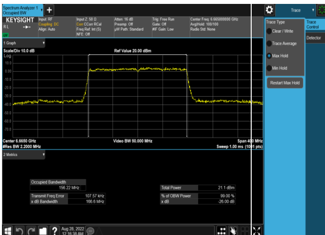
Plot 7-75. 26dB & 99% Bandwidth Plot Antenna 4a (160MHz 802.11ax (UNII Band 7) – Ch. 143, MCS2)
