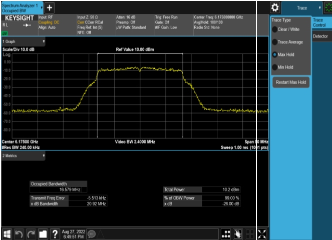
Plot 7-61. 26dB & 99% Bandwidth Plot Antenna 4a (20MHz 802.11a (UNII Band 5) – Ch. 45, MCS2)
