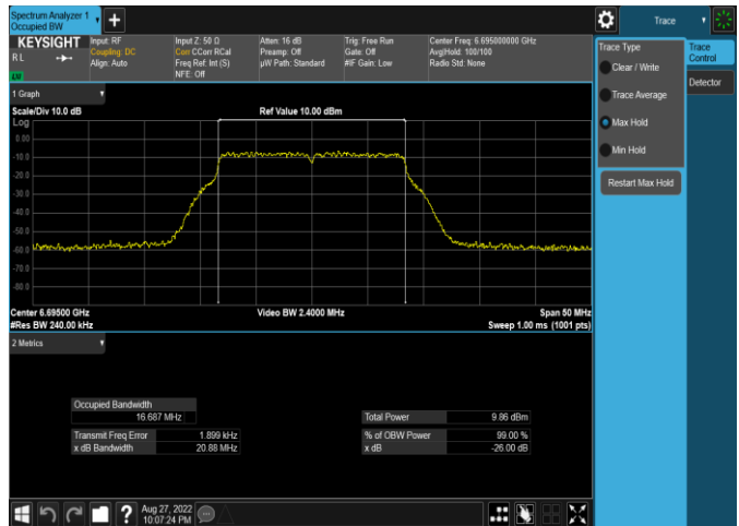
Plot 7-111. 26dB & 99% Bandwidth Plot Antenna 4a (20MHz 802.11a (UNII Band 7) – Ch. 149, MCS11)
