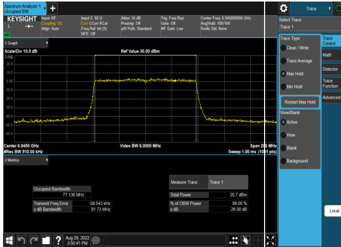
Plot 7-99. 26dB & 99% Bandwidth Plot Antenna 4a (80MHz 802.11ax (UNII Band 8) – Ch. 199, MCS4)
