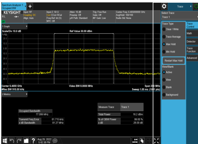
Plot 7-109. 26dB & 99% Bandwidth Plot Antenna 4a (80MHz 802.11ax (UNII Band 6) – Ch. 103, MCS11)
