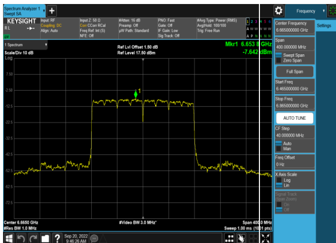
Plot 7-239. Power Spectral Density Plot Antenna 4a (160MHz 802.11ax (UNII Band 7) – Ch. 143, MCS11)
