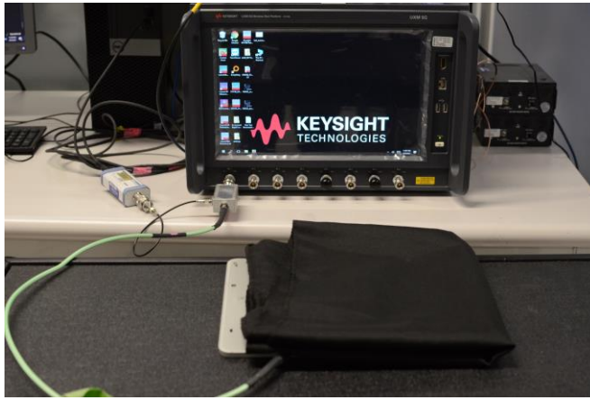
Test Setup Photo 3 – Conducted Test Setup (Figure 5-1a)
