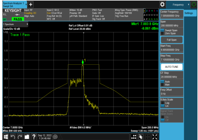
Plot 7-617. In-Band Emission Plot SDM Antenna WF5t (40MHz 802.11ax RU26 (UNII Band 8) – Ch. 211)
