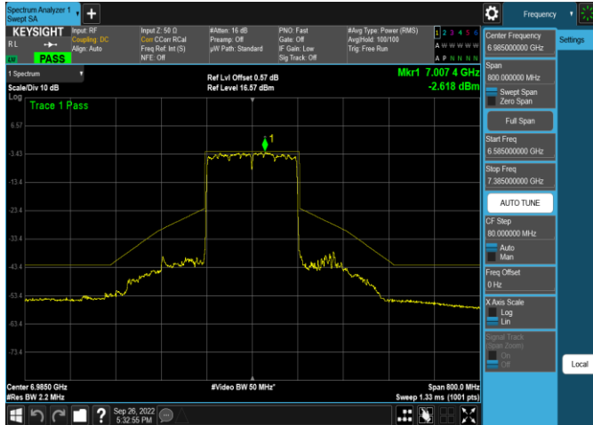
Plot 7-638. In-Band Emission Plot SDM Antenna WF5b (160MHz 802.11ax RU484 (UNII Band 8) – Ch. 207)
