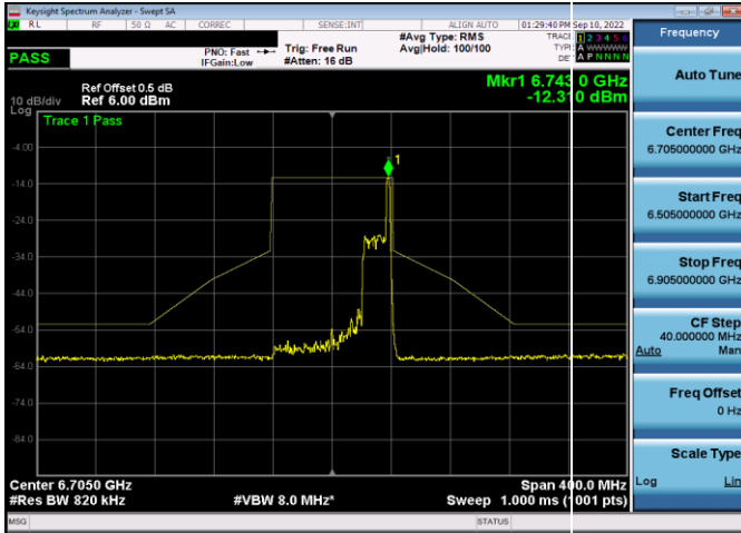
Plot 7-596. In-Band Emission Plot SDM Antenna WF5t (80MHz 802.11ax RU26 (UNII Band 7) – Ch. 151)
