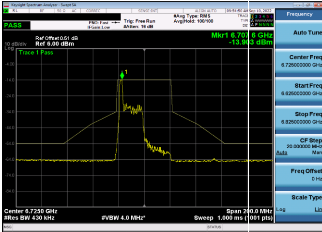
Plot 7-584. In-Band Emission Plot SDM Antenna WF5t (40MHz 802.11ax RU26 (UNII Band 7) – Ch. 155)
