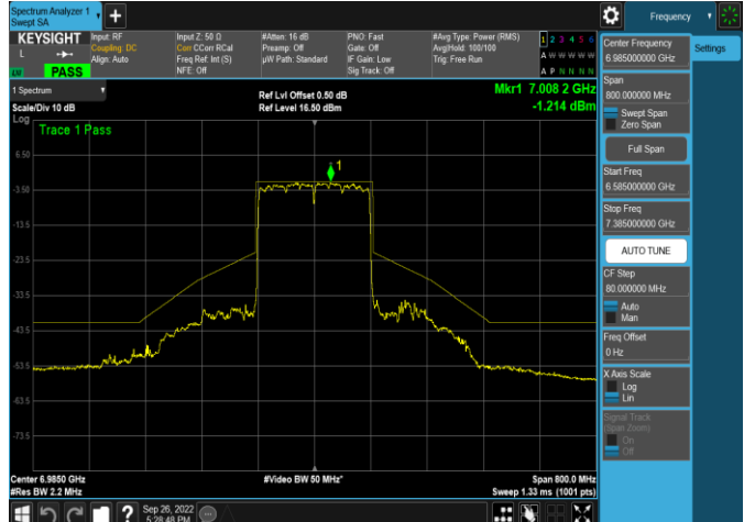
Plot 7-511. In-Band Emission Plot Antenna WF5b (160MHz 802.11ax RU484 (UNII Band 8) – Ch. 207)
