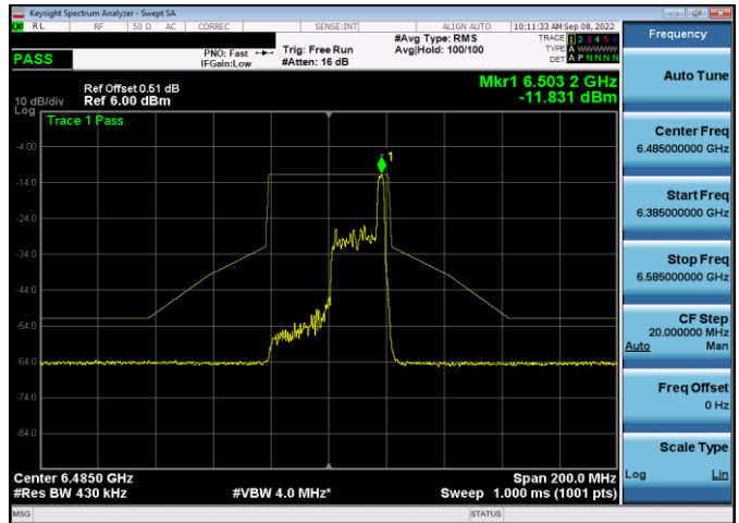
Plot 7-406. In-Band Emission Plot Antenna WF5t (40MHz 802.11ax RU26 (UNII Band 6) – Ch. 107)
