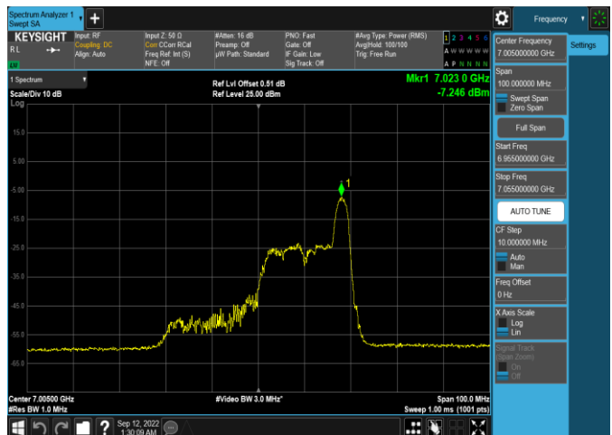
Plot 7-364. Power Spectral Density Plot SDM Antenna WF5t (40MHz 802.11ax RU26 (UNII Band 8) – Ch. 211)
