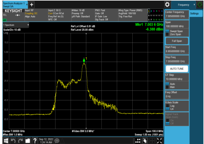
Plot 7-362. Power Spectral Density Plot SDM Antenna WF5t (40MHz 802.11ax RU26 (UNII Band 8) – Ch. 211)
