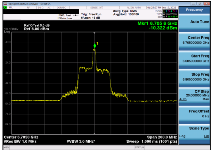
Plot 7-339. Power Spectral Density Plot SDM Antenna WF5t (80MHz 802.11ax RU26 (UNII Band 7) – Ch. 151)
