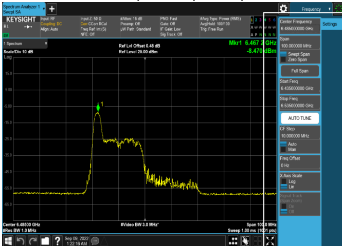
Plot 7-213. Power Spectral Density Plot Antenna WF5b (40MHz 802.11ax RU26 (UNII Band 6) – Ch. 107)
