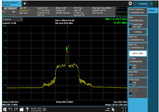
Plot 7-202. Power Spectral Density Plot Antenna WF5b (80MHz 802.11ax RU26 (UNII Band 5) – Ch. 39)
