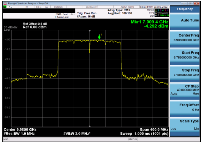
Plot 7-192. Power Spectral Density Plot Antenna WF5t (160MHz 802.11ax RU484 (UNII Band 8) – Ch. 207)
