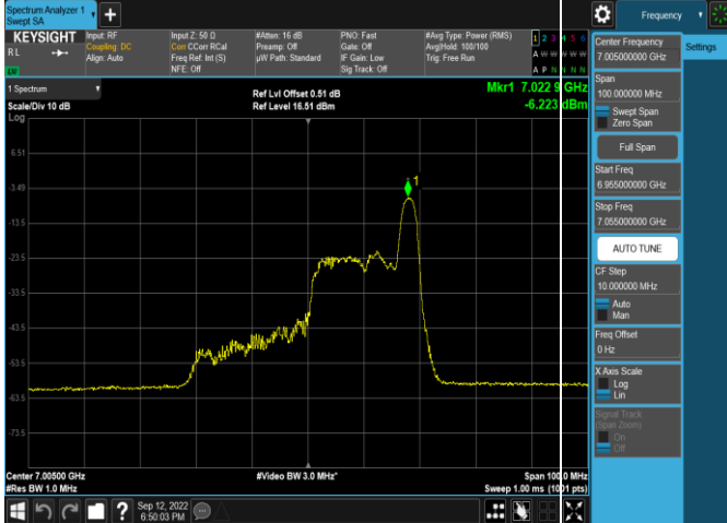
Plot 7-183. Power Spectral Density Plot Antenna WF5t (40MHz 802.11ax RU26 (UNII Band 8) – Ch. 211)
