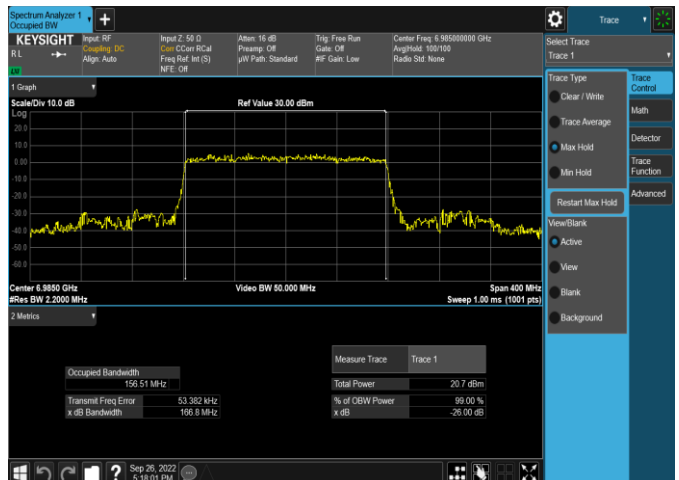
Plot 7-128. 26dB & 99% Bandwidth Plot Antenna WF5t (160MHz 802.11ax RU484 (UNII Band 8) – Ch. 207)
