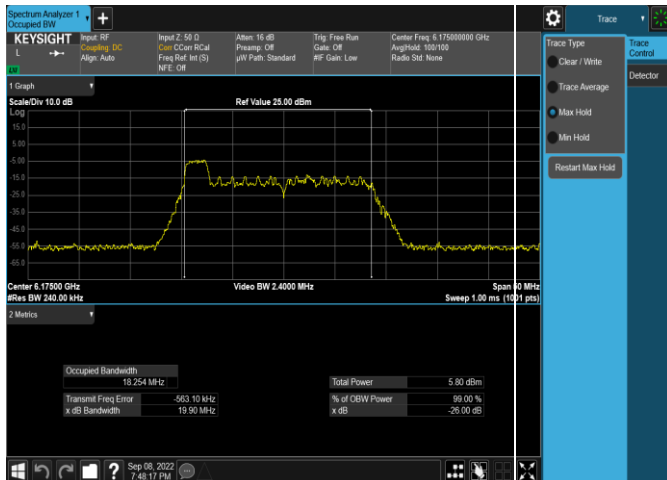
Plot 7-65. 26dB & 99% Bandwidth Plot Antenna WF5t (20MHz 802.11ax RU26 (UNII Band 5) – Ch. 45)
