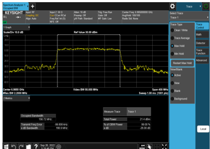
Plot 7-64. 26dB & 99% Bandwidth Plot Antenna WF5t (160MHz 802.11ax RU484 (UNII Band 8) – Ch. 207)
