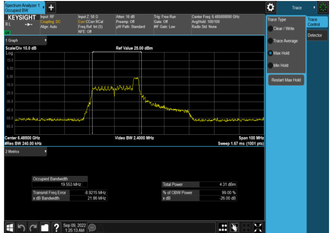
Plot 7-86. 26dB & 99% Bandwidth Plot Antenna WF5t (40MHz 802.11ax RU26 (UNII Band 6) – Ch. 107)
