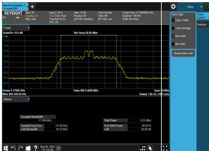
Plot 7-66. 26dB & 99% Bandwidth Plot Antenna WF5t (20MHz 802.11ax RU26 (UNII Band 5) – Ch. 45)
