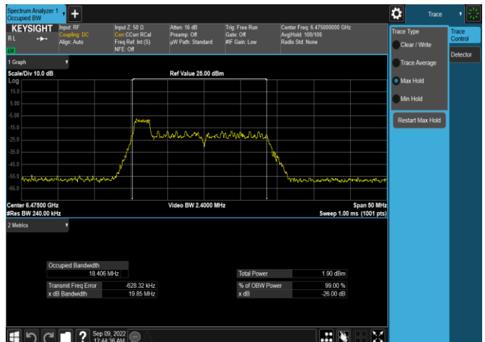
Plot 7-81. 26dB & 99% Bandwidth Plot Antenna WF5t (20MHz 802.11ax RU26 (UNII Band 6) – Ch. 105)
