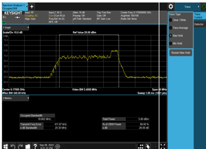
Plot 7-67. 26dB & 99% Bandwidth Plot Antenna WF5t (20MHz 802.11ax RU26 (UNII Band 5) – Ch. 45)
