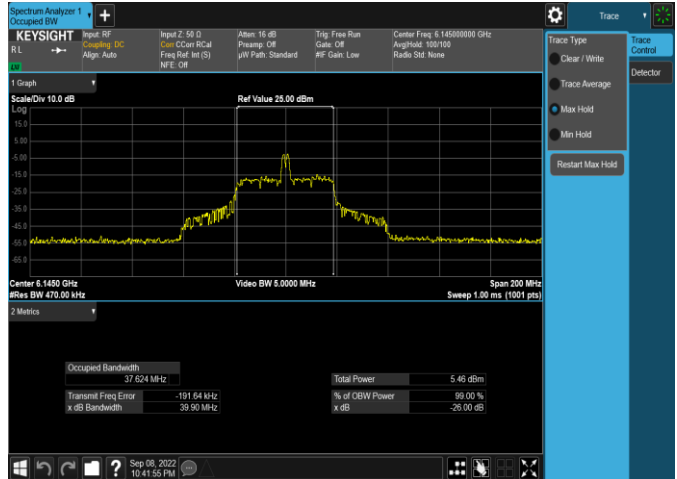
Plot 7-74. 26dB & 99% Bandwidth Plot Antenna WF5t (80MHz 802.11ax RU26 (UNII Band 5) – Ch. 39)
