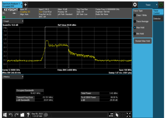
Plot 7-5. 26dB & 99% Bandwidth Plot Antenna WF5t (40MHz 802.11ax RU26 (UNII Band 5) – Ch. 43)
