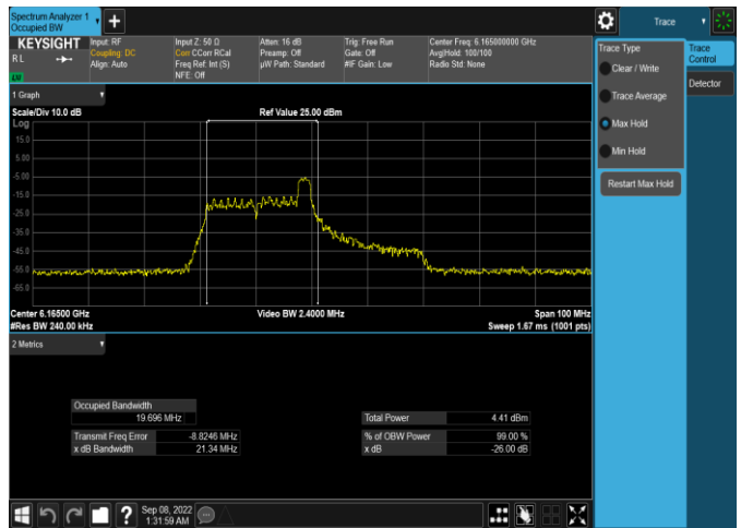
Plot 7-6. 26dB & 99% Bandwidth Plot Antenna WF5t (40MHz 802.11ax RU26 (UNII Band 5) – Ch. 43)
