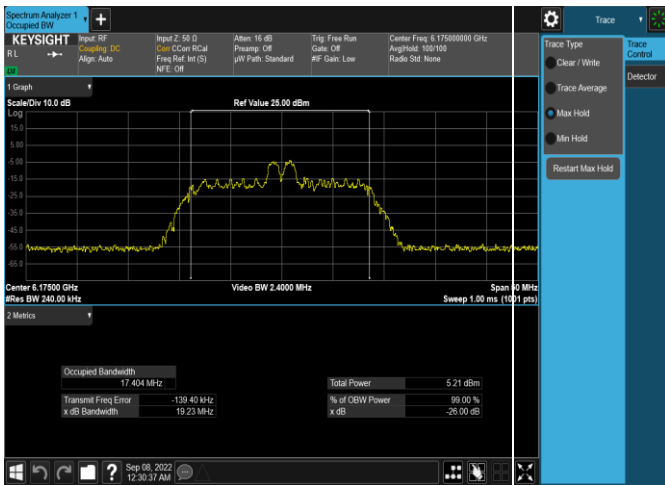
Plot 7-2. 26dB & 99% Bandwidth Plot Antenna WF5t (20MHz 802.11ax RU26 (UNII Band 5) – Ch. 45)
