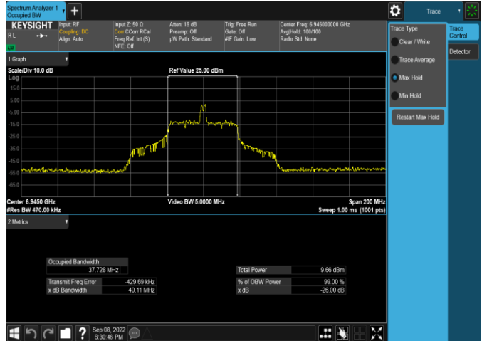
Plot 7-58. 26dB & 99% Bandwidth Plot Antenna WF5t (80MHz 802.11ax RU26 (UNII Band 8) – Ch. 199)
