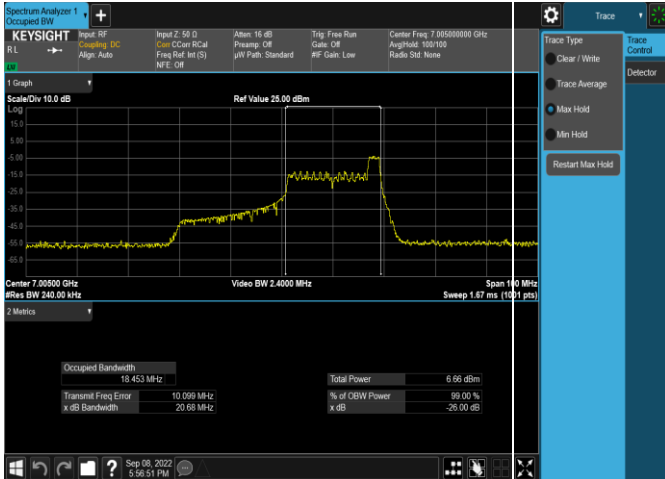
Plot 7-55. 26dB & 99% Bandwidth Plot Antenna WF5t (40MHz 802.11ax RU26 (UNII Band 8) – Ch. 211)
