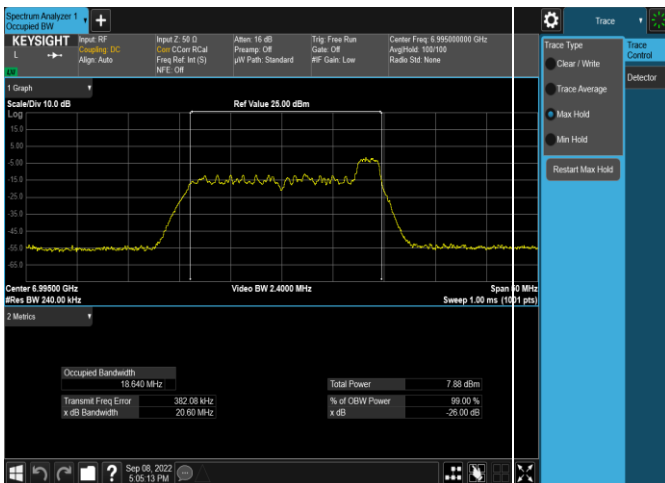
Plot 7-51. 26dB & 99% Bandwidth Plot Antenna WF5t (20MHz 802.11ax RU26 (UNII Band 8) - Ch. 209)
