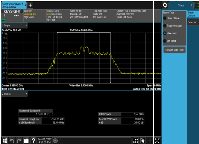
Plot 7-50. 26dB & 99% Bandwidth Plot Antenna WF5t (20MHz 802.11ax RU26 (UNII Band 8) - Ch. 209)
