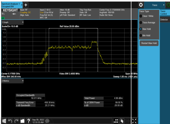
Plot 7-3. 26dB & 99% Bandwidth Plot Antenna WF5t (20MHz 802.11ax RU26 (UNII Band 5) – Ch. 45)
