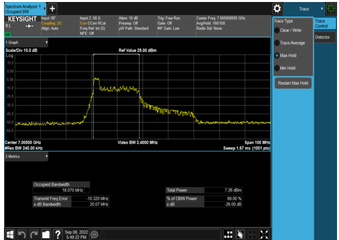
Plot 7-53. 26dB & 99% Bandwidth Plot Antenna WF5t (40MHz 802.11ax RU26 (UNII Band 8) - Ch. 211)
