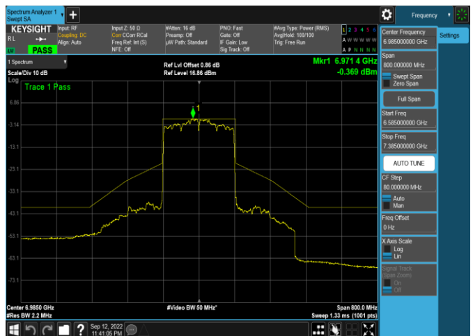
Plot 7-456. In-Band Emission Plot Antenna WF5b (160MHz 802.11ax (UNII Band 8) – Ch. 207, MCS11)
