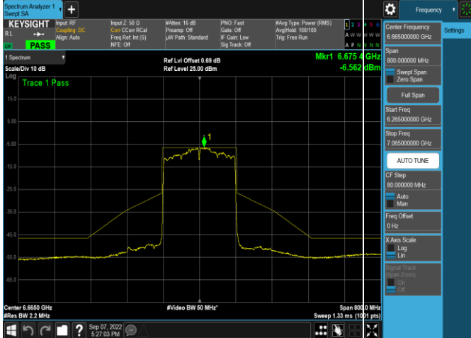
Plot 7-479. In-Band Emission Plot SDM Antenna WF5t (160MHz 802.11ax (UNII Band 7) – Ch. 143, MCS2)
