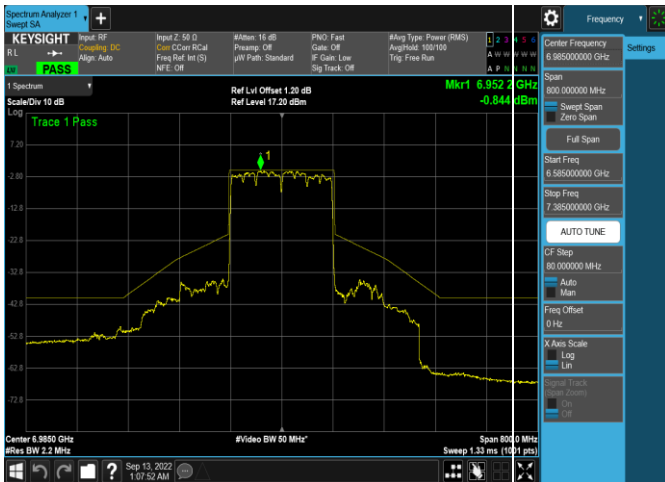
Plot 7-392. In-Band Emission Plot Antenna WF5t (160MHz 802.11ax (UNII Band 8) – Ch. 207, MCS11)
