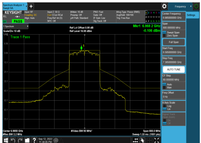
Plot 7-396. In-Band Emission Plot Antenna WF5t (160MHz 802.11ax (UNII Band 8) – Ch. 207, MCS11)
