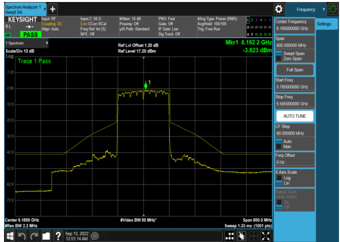
Plot 7-377. In-Band Emission Plot Antenna WF5t (160MHz 802.11ax (UNII Band 5) – Ch. 47, MCS11)
