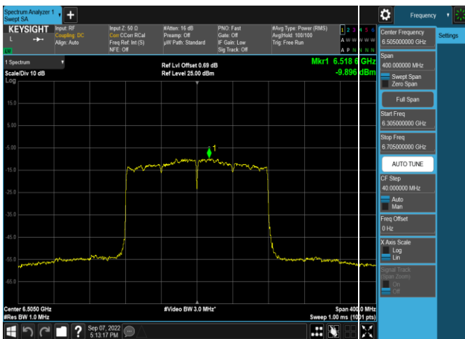
Plot 7-255. Power Spectral Density Plot SDM Antenna WF5t (160MHz 802.11ax (UNII Band 6) – Ch. 111, MCS2)
