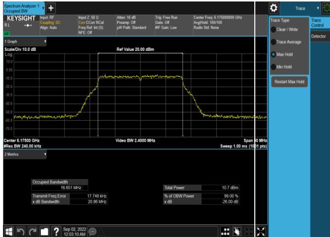
Plot 7-101. 26dB & 99% Bandwidth Plot Antenna WF5b (20MHz 802.11a (UNII Band 5) – Ch. 47, 54Mbps)
