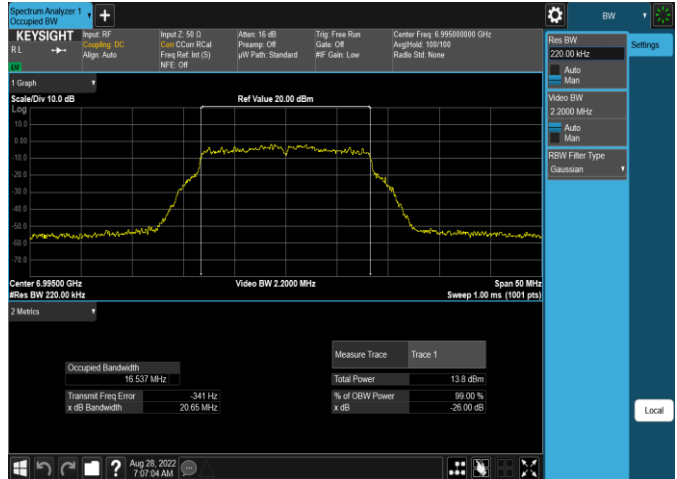
Plot 7-76. 26dB & 99% Bandwidth Plot Antenna WF5b (20MHz 802.11a (UNII Band 8) – Ch. 209, 12Mbps)
