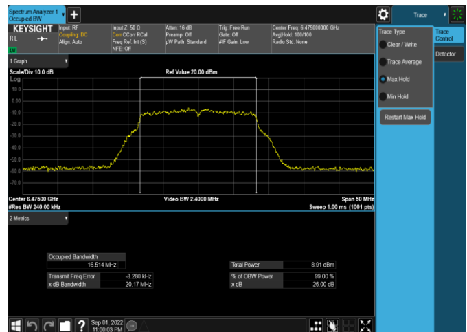
Plot 7-86. 26dB & 99% Bandwidth Plot Antenna WF5b (20MHz 802.11a (UNII Band 6) – Ch. 105, 24Mbps)
