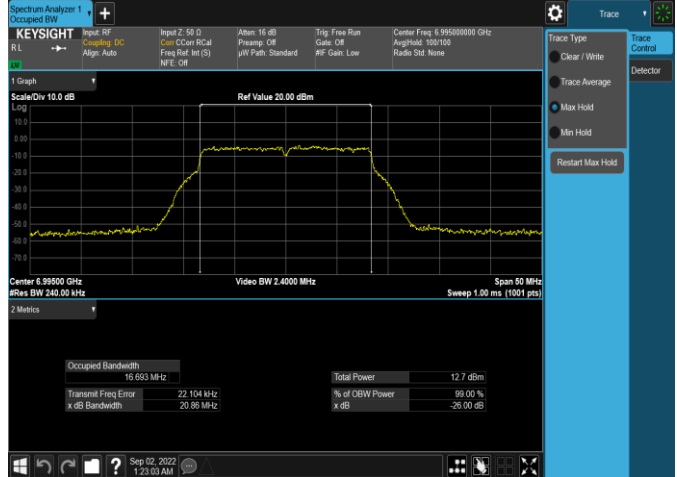
Plot 7-116. 26dB & 99% Bandwidth Plot Antenna WF5b (20MHz 802.11a (UNII Band 8) – Ch. 209, 54Mbps)
