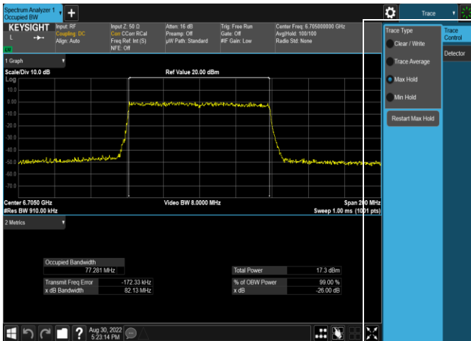
Plot 7-94. 26dB & 99% Bandwidth Plot Antenna WF5b (80MHz) 802.11ax (UNII Band 7) – Ch. 151, MCS4)
