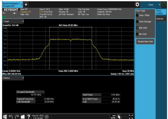
Plot 7-111. 26dB & 99% Bandwidth Plot Antenna WF5b (20MHz 802.11a (UNII Band 7) – Ch. 149, 54Mbps)
