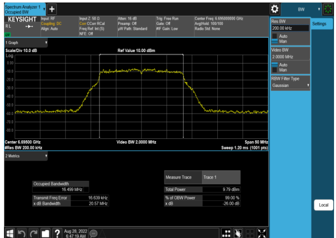
Plot 7-71. 26dB & 99% Bandwidth Plot Antenna WF5b (20MHz 802.11a (UNII Band 7) – Ch. 149, 12Mbps)
