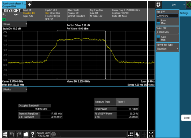
Plot 7-81. 26dB & 99% Bandwidth Plot Antenna WF5b (20MHz 802.11a (UNII Band 5) – Ch. 47, 24Mbps)
