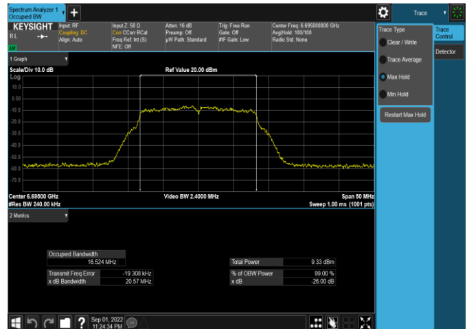
Plot 7-91. 26dB & 99% Bandwidth Plot Antenna WF5b (20MHz 802.11a (UNII Band 7) – Ch. 149, 24Mbps)
