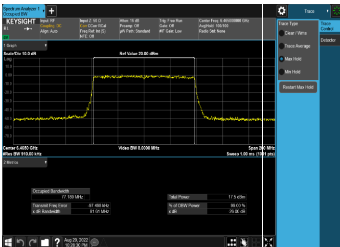
Plot 7-29. 26dB & 99% Bandwidth Plot Antenna WF5t (80MHz) 802.11ax (UNII Band 6) – Ch. 103, MCS4)
