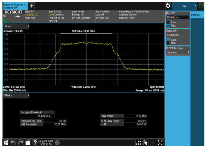
Plot 7-6. 26dB & 99% Bandwidth Plot Antenna WF5t (20MHz 802.11a (UNII Band 6) – Ch. 105, 12Mbps)
