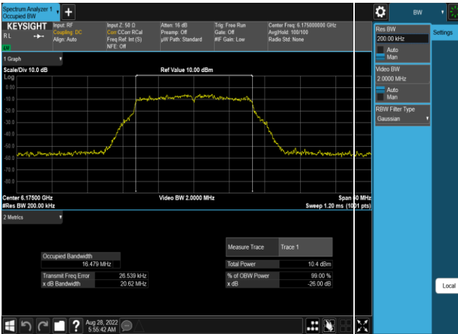
Plot 7-61. 26dB & 99% Bandwidth Plot Antenna WF5b (20MHz 802.11a (UNII Band 5) – Ch. 47, 12Mbps)
