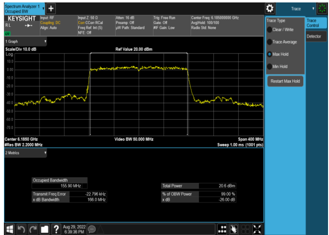
Plot 7-45. 26dB & 99% Bandwidth Plot Antenna WF5t (160MHz 802.11ax (UNII Band 5) – Ch. 47, MCS11)
