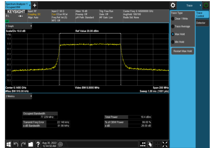
Plot 7-64. 26dB & 99% Bandwidth Plot Antenna WF5b (80MHz 802.11ax (UNII Band 5) – Ch. 39, MCS2)
