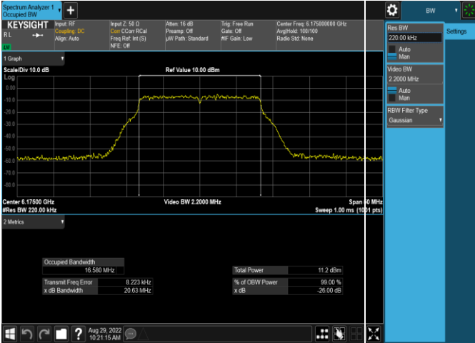
Plot 7-41. 26dB & 99% Bandwidth Plot Antenna WF5t (20MHz 802.11a (UNII Band 5) – Ch. 47, 54Mbps)
