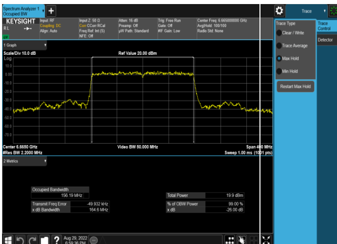
Plot 7-55. 26dB & 99% Bandwidth Plot Antenna WF5t (160MHz 802.11ax (UNII Band 7) – Ch. 143, MCS11)
