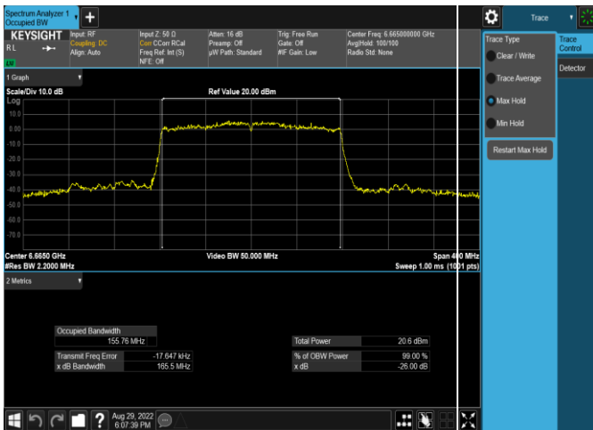
Plot 7-35. 26dB & 99% Bandwidth Plot Antenna WF5t (160MHz 802.11ax (UNII Band 7) – Ch. 143, MCS4)
