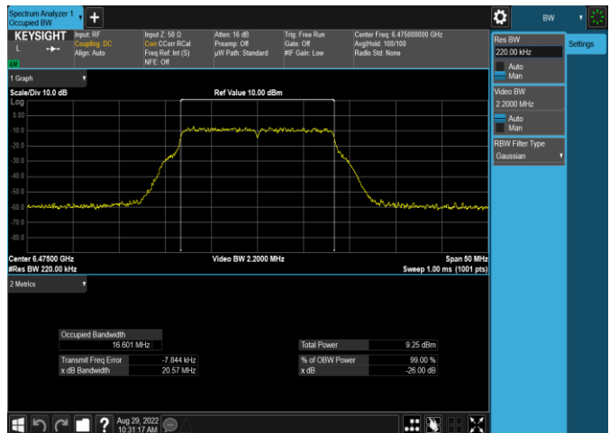
Plot 7-46. 26dB & 99% Bandwidth Plot Antenna WF5t (20MHz 802.11a (UNII Band 6) – Ch. 105, 54Mbps)
