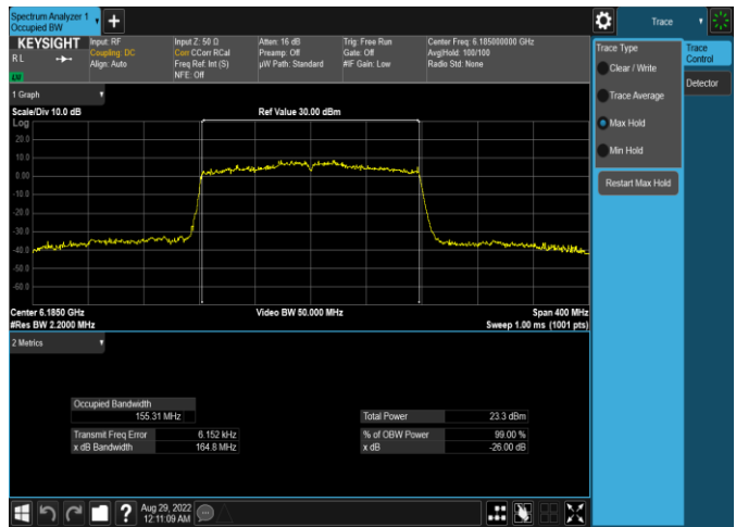
Plot 7-5. 26dB & 99% Bandwidth Plot Antenna WF5t (160MHz 802.11ax (UNII Band 5) – Ch. 47, MCS2)
