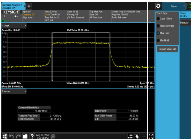
Plot 7-9. 26dB & 99% Bandwidth Plot Antenna WF5t (80MHz 802.11ax (UNII Band 6) – Ch. 103, MCS2)
