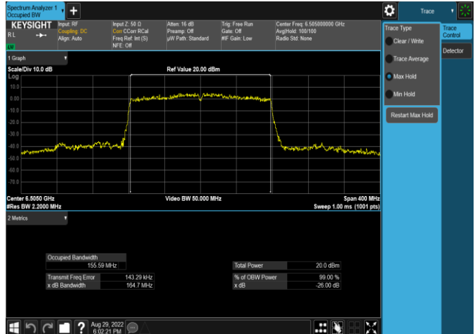
Plot 7-30. 26dB & 99% Bandwidth Plot Antenna WF5t (160MHz) 802.11ax (UNII Band 6) – Ch. 111, MCS4)
