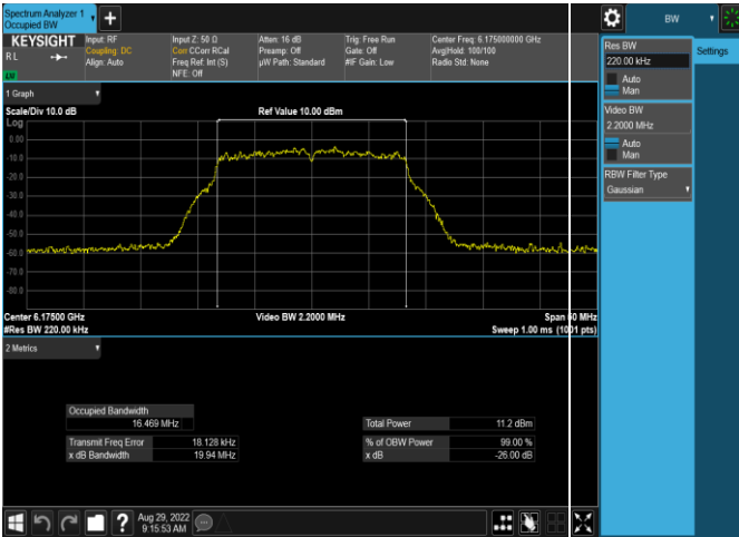
Plot 7-21. 26dB & 99% Bandwidth Plot Antenna WF5t (20MHz 802.11a (UNII Band 5) – Ch. 47, 24Mbps)
