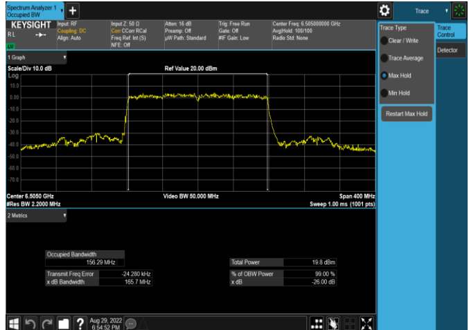
Plot 7-50. 26dB & 99% Bandwidth Plot Antenna WF5t (160MHz 802.11ax (UNII Band 6) – Ch. 111, MCS11)
