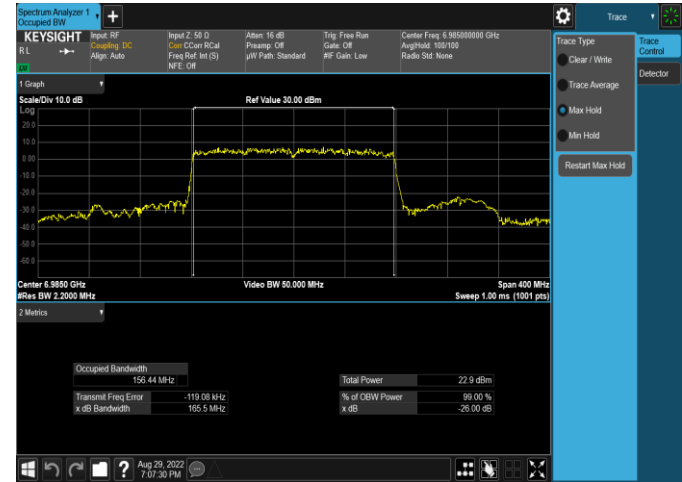
Plot 7-60. 26dB & 99% Bandwidth Plot Antenna WF5t (160MHz 802.11ax (UNII Band 8) – Ch. 207, MCS11)
