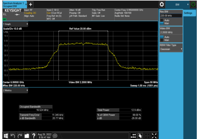
Plot 7-16. 26dB & 99% Bandwidth Plot Antenna WF5t (20MHz 802.11a (UNII Band 8) – Ch. 209, 12Mbps)
