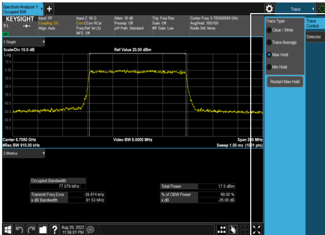
Plot 7-54. 26dB & 99% Bandwidth Plot Antenna WF5t (80MHz 802.11ax (UNII Band 7) – Ch. 151, MCS11)
