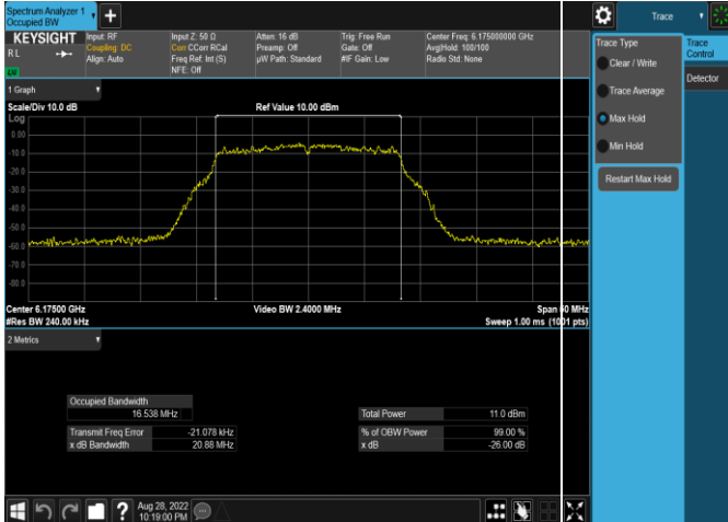
Plot 7-1. 26dB & 99% Bandwidth Plot Antenna WF5t (20MHz 802.11a (UNII Band 5) – Ch. 45, 12Mbps)
