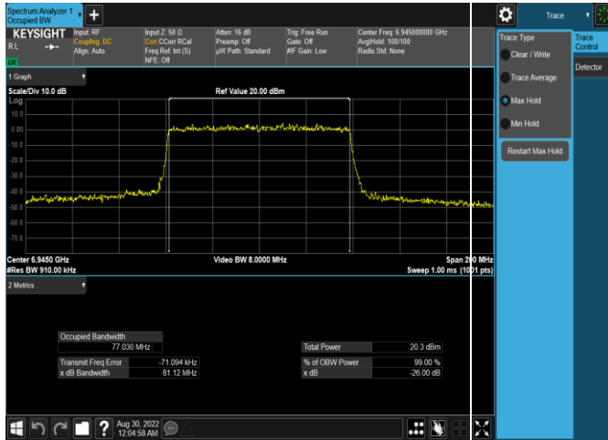
Plot 7-59. 26dB & 99% Bandwidth Plot Antenna WF5t (80MHz 802.11ax (UNII Band 8) – Ch. 199, MCS11)
